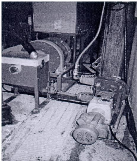
*FIG. 4. Pilot plant ball mill, pump box and classification screen feed pump.*
