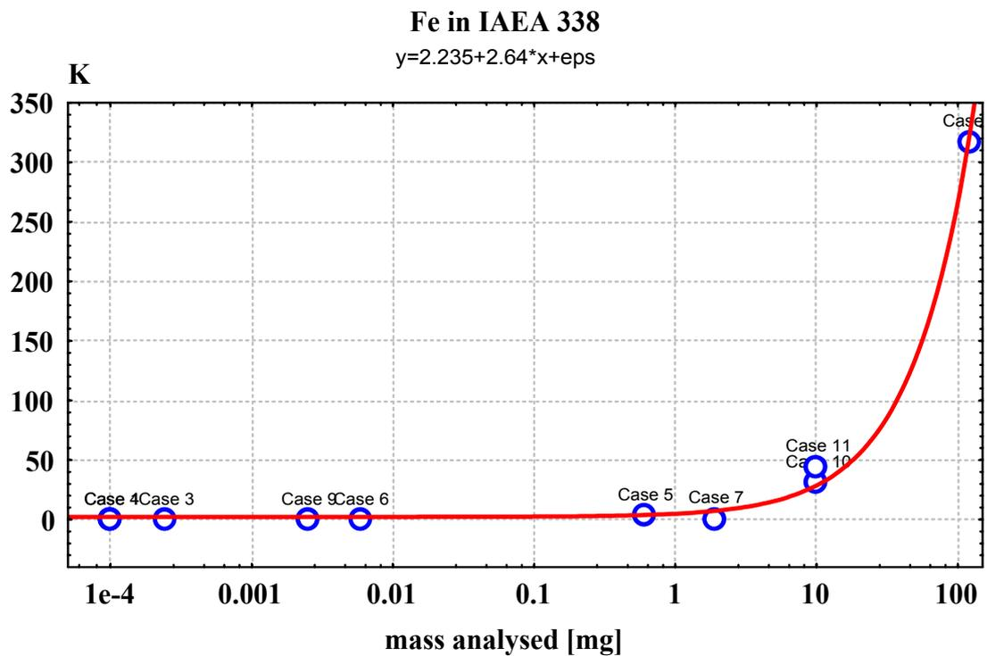
FIG. 6. Ingamels' sampling constant  $K_S$  versus sample mass used for repetitive analysis of Fe by different techniques in IAEA 338.
