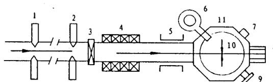
FIG. 1: A diagram of the scanning proton microprobe 1: object; 2: aperture; 3: vacuum valve; 4: quadrupole lenses; 5: deflect. Coils; 6: Si(Li) detector; 7: window; 8: faraday cups; 9: vacuum pump; 10: sample target; 11: target chamber.
