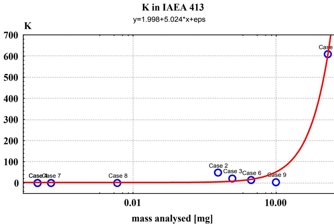
FIG. 11. Ingamels' sampling constant  $K_S$  versus sample mass used for repetitive analysis of K by different techniques in IAEA 413.
