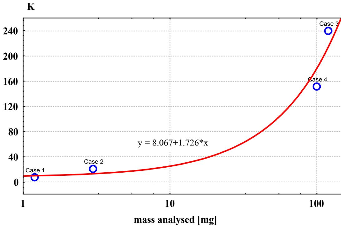
FIG. 19. Ingamels' sampling constant  $K_S$  versus sample mass used for repetitive analysis of Cd by different techniques in IAEA 413.
