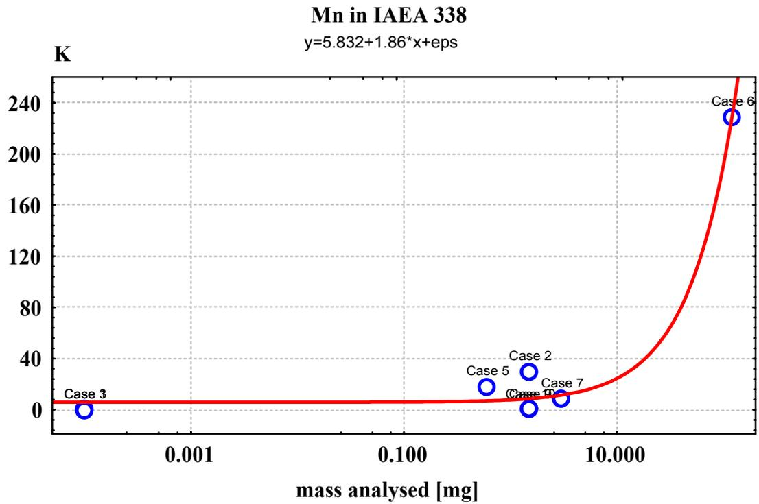
FIG. 5. Ingamels' sampling constant  $K_S$  versus sample mass used for repetitive analysis of Mn by different techniques in IAEA 338.
