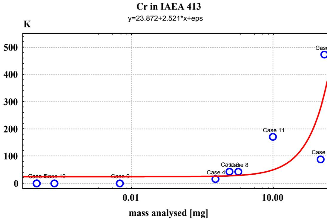
FIG. 13. Ingamels' sampling constant  $K_S$  versus sample mass used for repetitive analysis of Cr by different techniques in IAEA 413.
