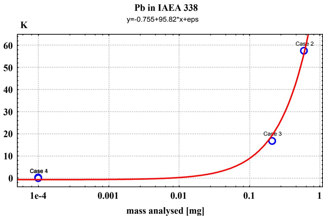
FIG. 10. Ingamels' sampling constant  $K_S$  versus sample mass used for repetitive analysis of Pb by different techniques in IAEA 338.
