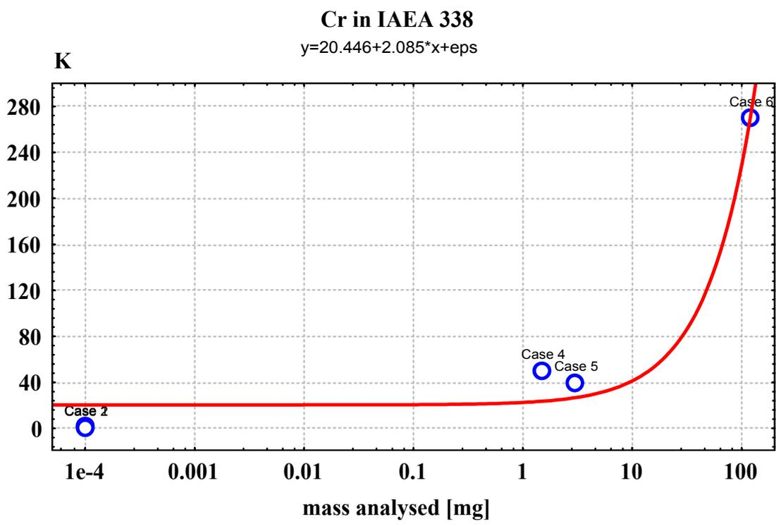
FIG. 4. Ingamels' sampling constant  $K_S$  versus sample mass used for repetitive analysis of Cr by different techniques in IAEA 338.
