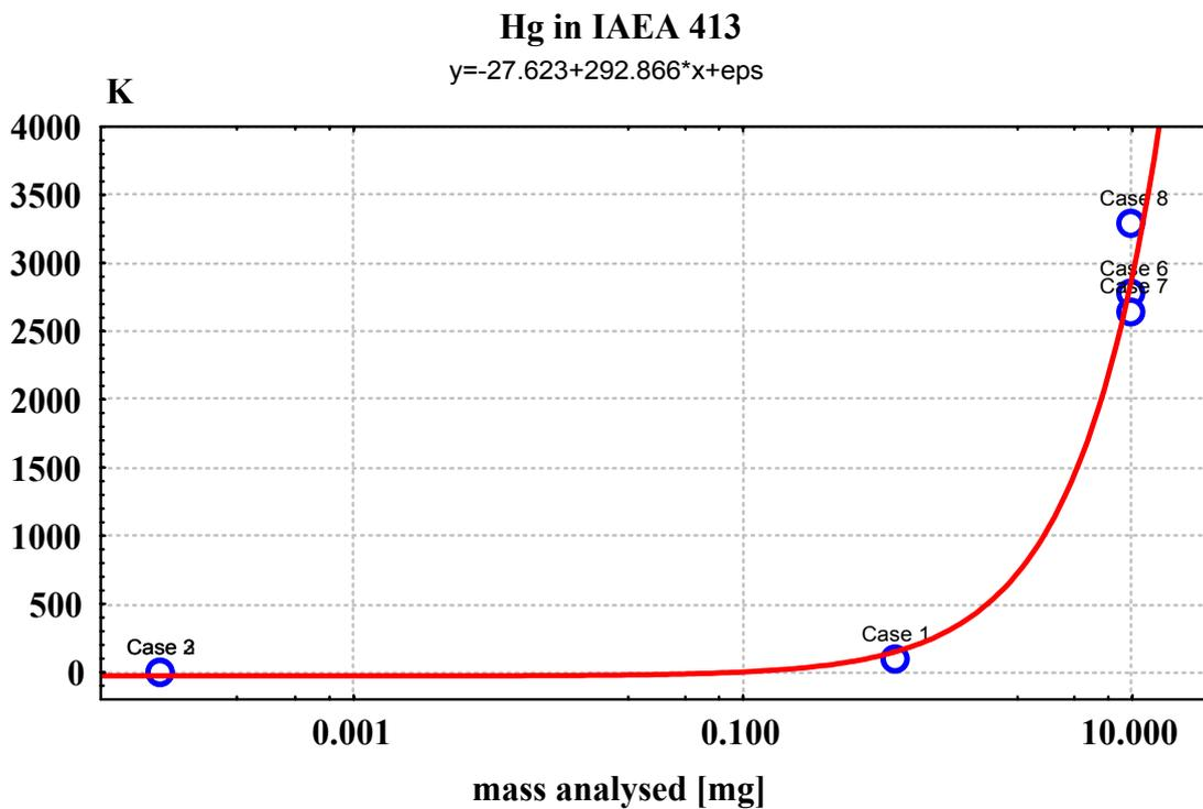
FIG. 20. Ingamels' sampling constant  $K_S$  versus sample mass used for repetitive analysis of Hg by different techniques in IAEA 413.
