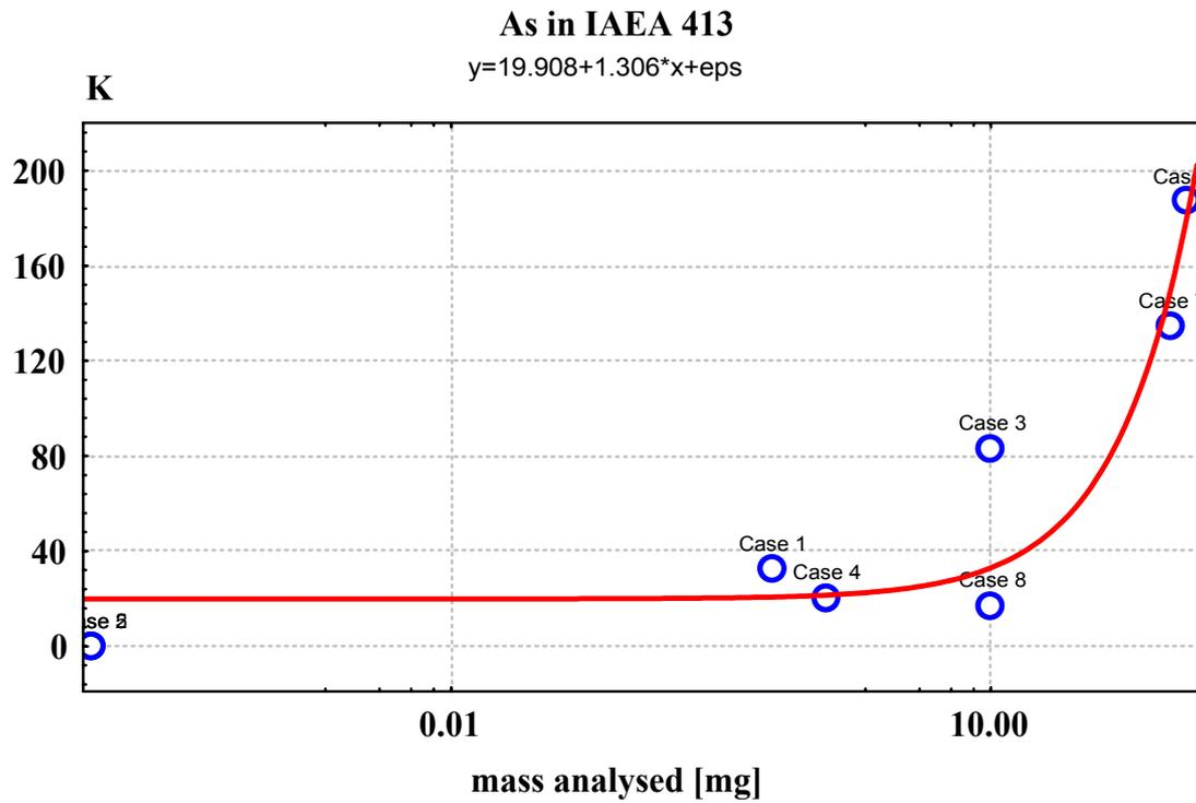
FIG. 17. Ingamels' sampling constant  $K_S$  versus sample mass used for repetitive analysis of As by different techniques in IAEA 413.
