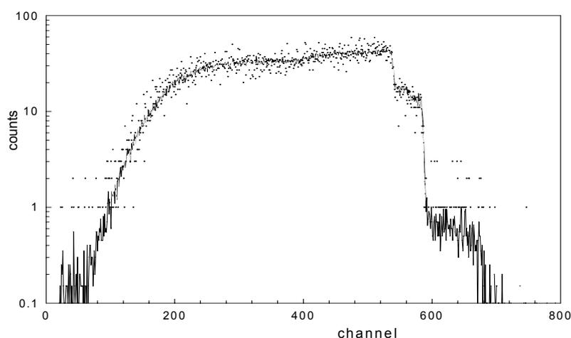
FIG 5. *RBS spectrum of the Algae sample (solid line) and contamination zone from the Figure 6b (dotted line). No significant differences in matrix composition are visible for this particular example.*
