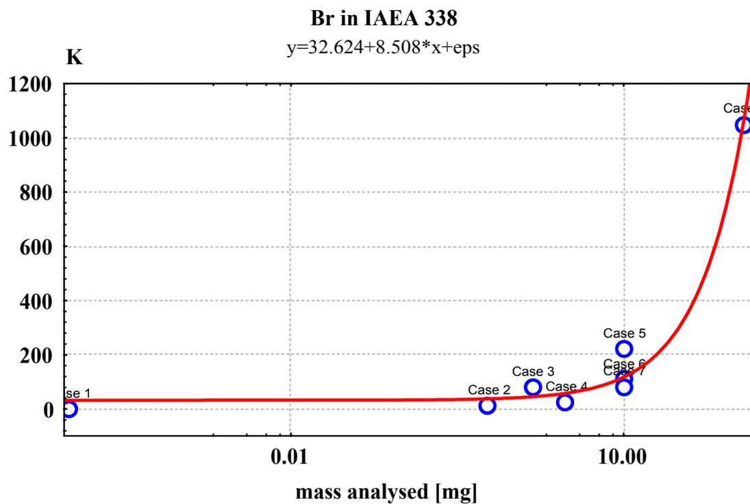
FIG. 8. Ingamels' sampling constant  $K_S$  versus sample mass used for repetitive analysis of Br by different techniques in IAEA 338.
