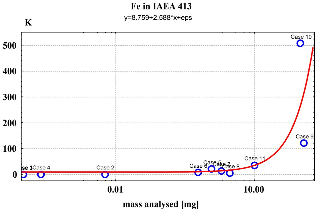
FIG. 15. Ingamels' sampling constant  $K_S$  versus sample mass used for repetitive analysis of Fe by different techniques in IAEA 413.
