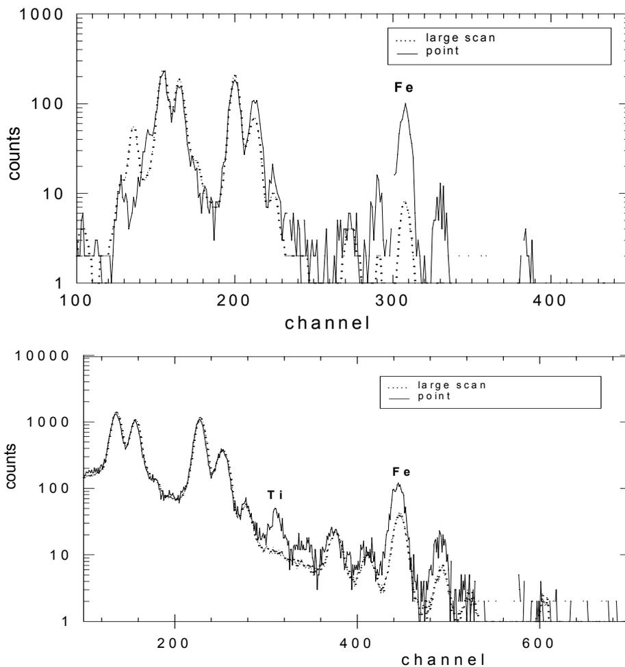
FIG 6a (UP) AND 6b (DOWN). PIXE spectrum of two observed inhomogeneities in the Algae sample.
