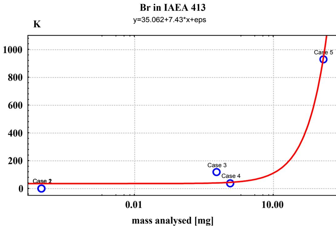
FIG. 18. Ingamels' sampling constant  $K_S$  versus sample mass used for repetitive analysis of Br by different techniques in IAEA 413.
