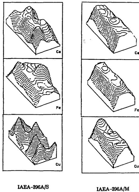
FIG. 5: Distribution maps of elements in the scanning region 100 X200 mm<sup>2</sup> of Vienna urban dust IAEA-396A/M and IAEA-396A/S.
