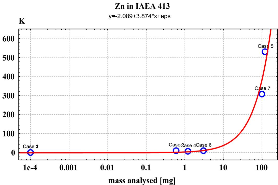
FIG. 16. Ingamels' sampling constant  $K_S$  versus sample mass used for repetitive analysis of Zn by different techniques in IAEA 413.
