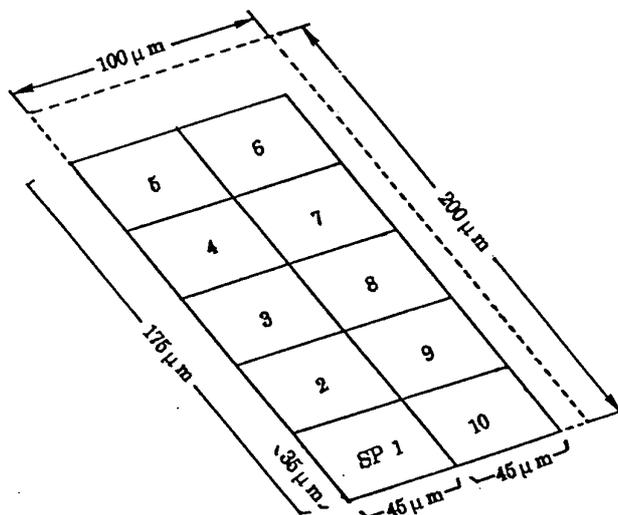
FIG. 2: A scanning region of micro-PIXE.
