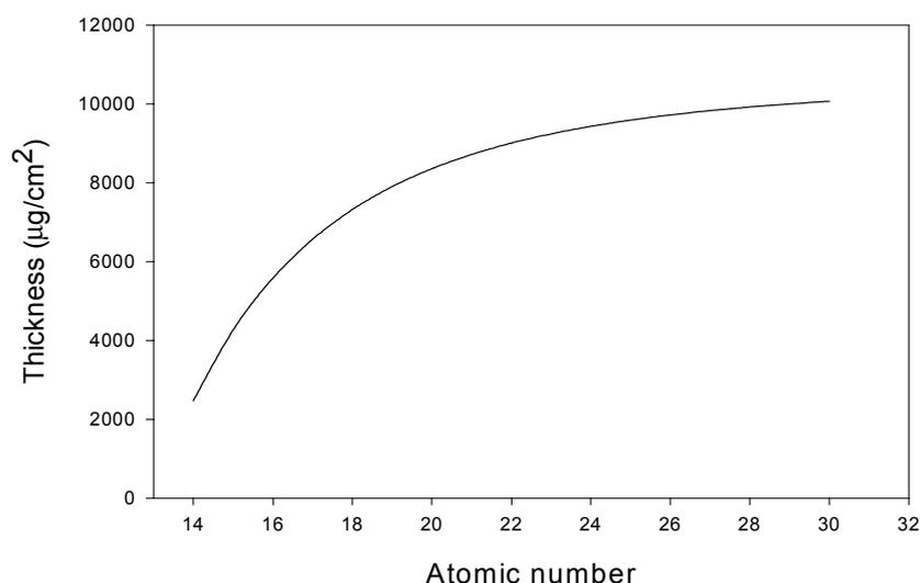
FIG. 3. Thickness of the biological matrix sample that corresponds to the thickness of the sample slab that contribute to the 90% of the K X ray yield for the elements of atomic number  $14 < Z < 30$  excited by 3 MeV protons.
