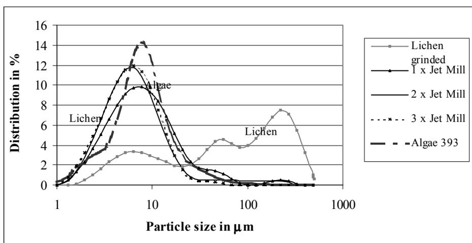
Figure 1. Particle Size Distribution of Algae and Lichen Candidate Reference Materials.
