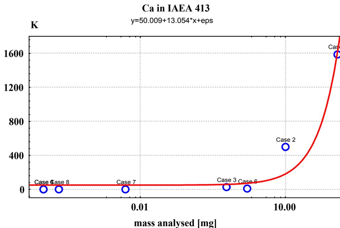
FIG. 12. Ingamels' sampling constant  $K_S$  versus sample mass used for repetitive analysis of Ca by different techniques in IAEA 413.
