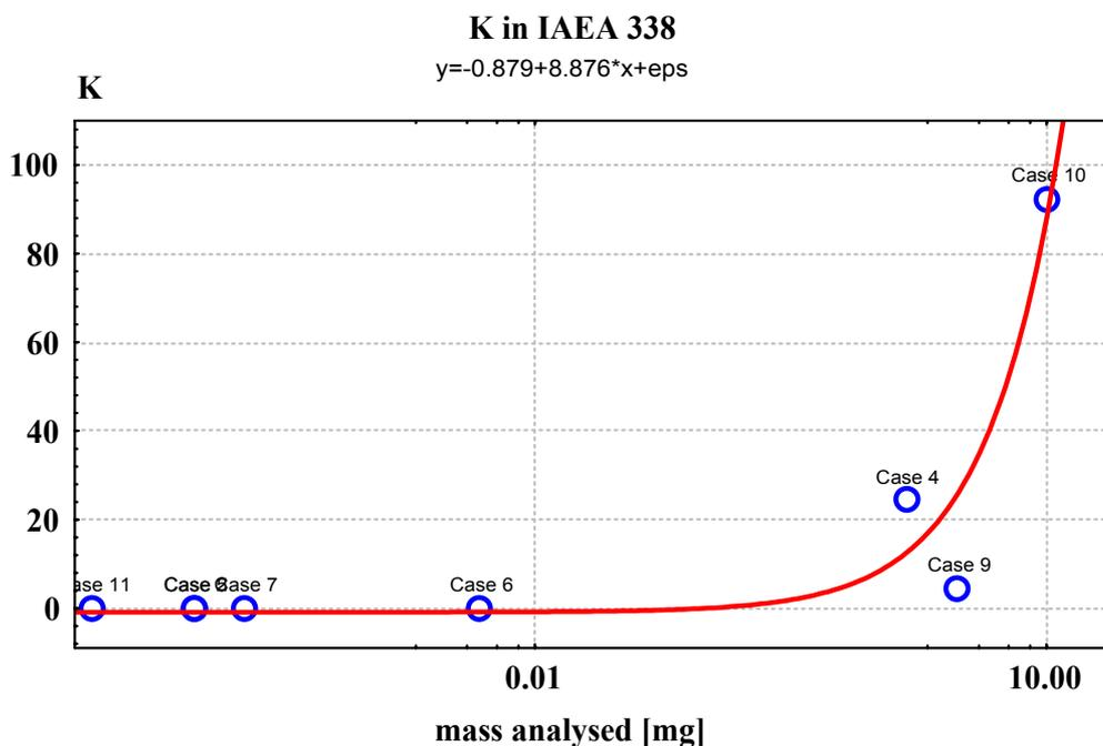
FIG. 2. Ingamels' sampling constant  $K_S$  versus sample mass used for repetitive analysis of K by different techniques in IAEA 338.
