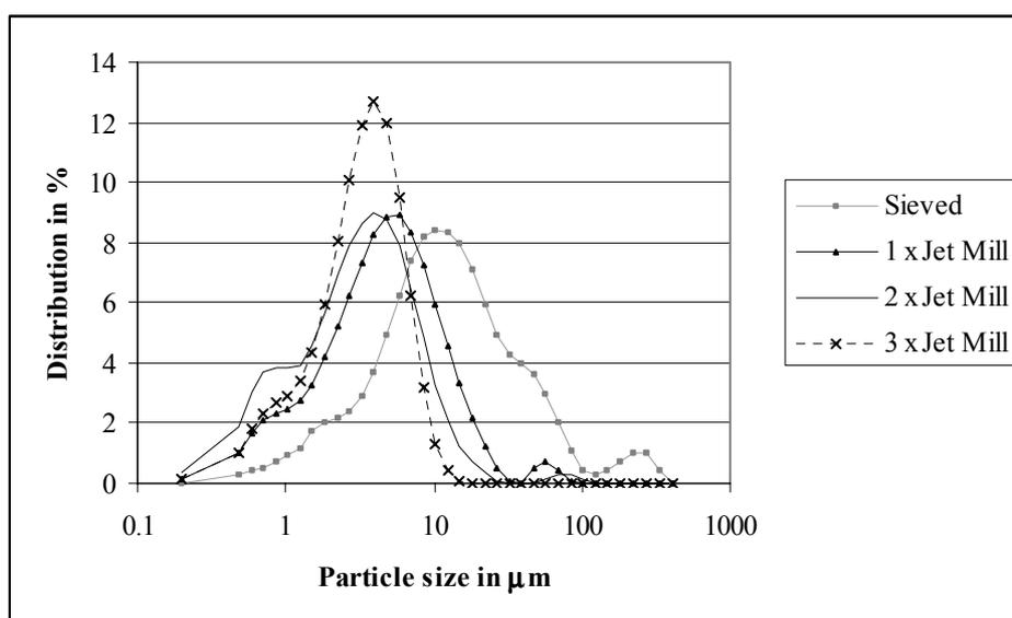
Figure 2. Particle Size Distribution of Urban Dust Candidate Reference Material.
