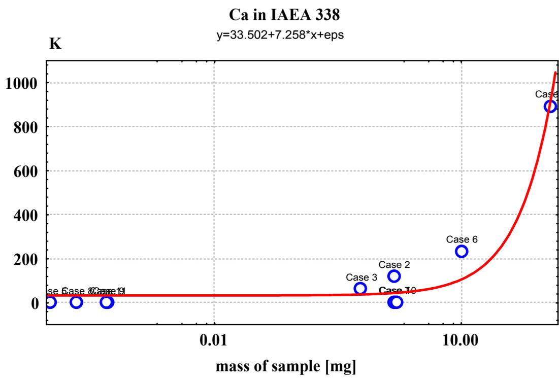
FIG. 3. Ingamels' sampling constant  $K_S$  versus sample mass used for repetitive analysis of Ca by different techniques in IAEA 338.
