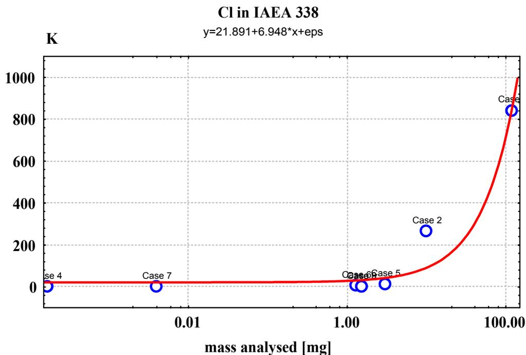
FIG. 1. Ingamels' sampling constant  $K_S$  versus sample mass used for repetitive analysis of Cl by different techniques in IAEA 338.
