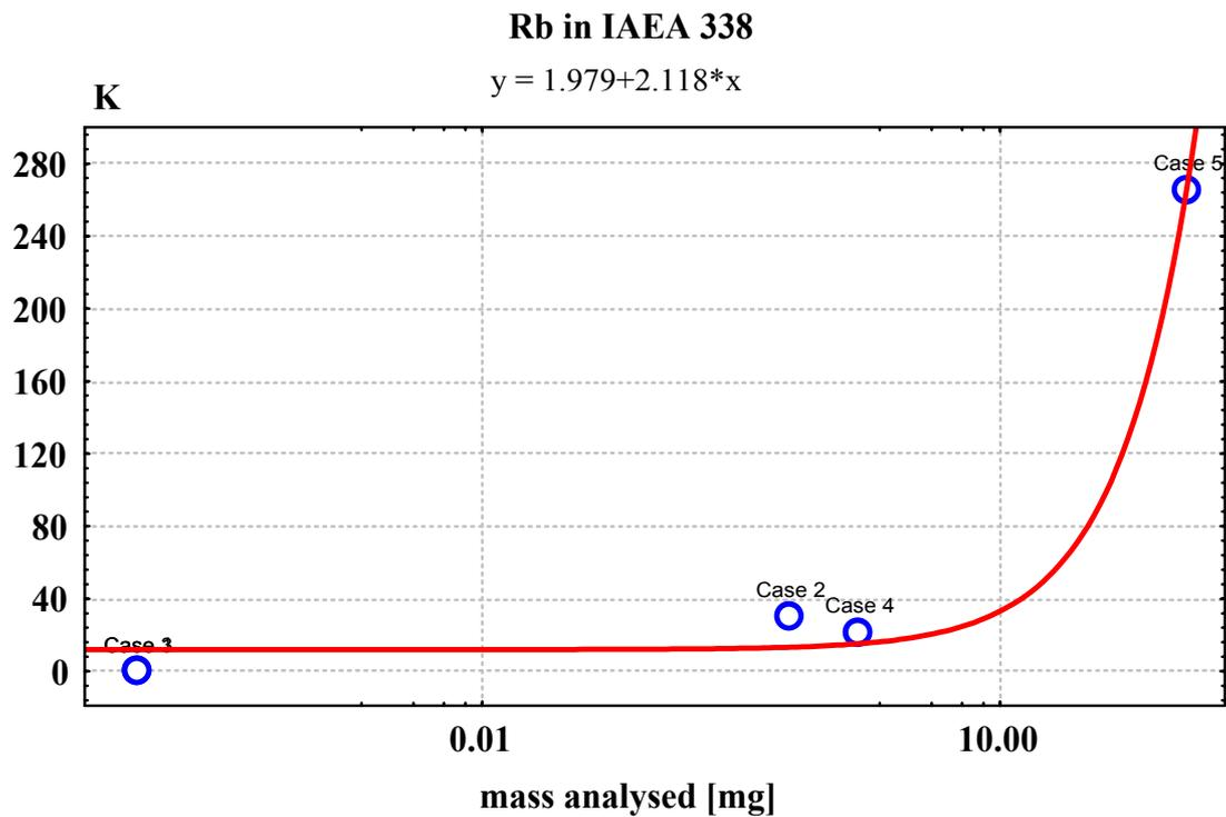
FIG. 9. Ingamels' sampling constant  $K_S$  versus sample mass used for repetitive analysis of Rb by different techniques in IAEA 338.
