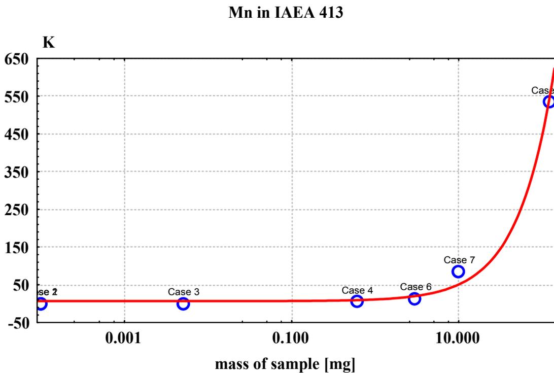
FIG. 14. Ingamels' sampling constant  $K_S$  versus sample mass used for repetitive analysis of Mn by different techniques in IAEA 413.
