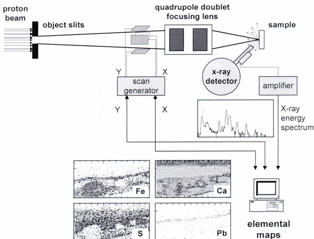
FIG 2. Schematic presentation of the IRB nuclear microprobe PIXE set-up.
