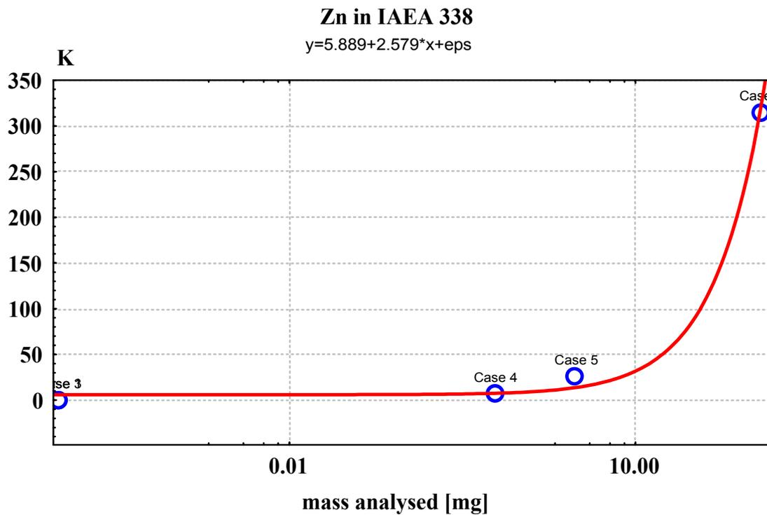
FIG. 7. Ingamels' sampling constant  $K_S$  versus sample mass used for repetitive analysis of Zn by different techniques in IAEA 338.
