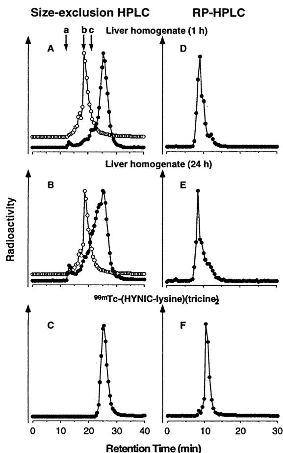
FIG. 5. Analysis of liver homogenates injected with  $^{99m}\text{Tc}-(\text{HYNIC-NGA})(\text{tricine})_2$ . Comparative studies using size exclusion HPLC (left) and RP-HPLC (right).
