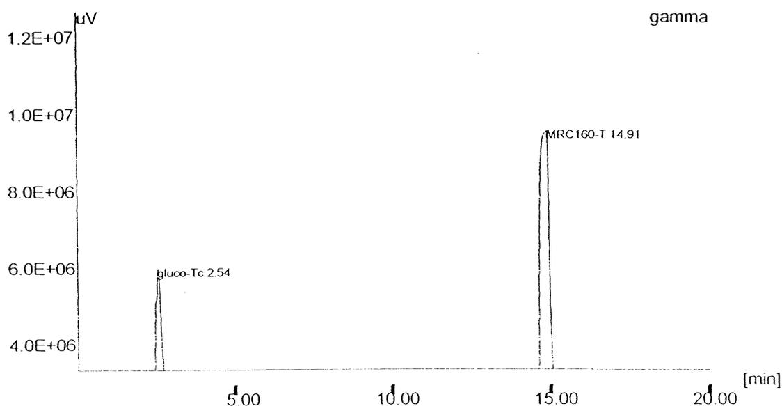
FIG. 3. Radiochromatogram of  $^{99m}\text{Tc}$ -MAG-3-RC-160 (Crest Pak C-18, 5  $\mu\text{m}$ , 4.6  $\times$  150 mm).
