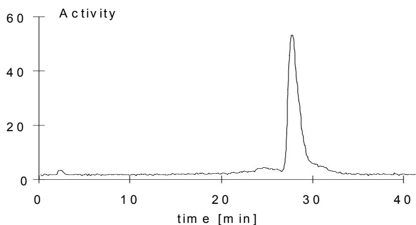
FIG. 2. A typical HPLC profile of  $^{99\text{m}}\text{Tc}$ -RC-160.
