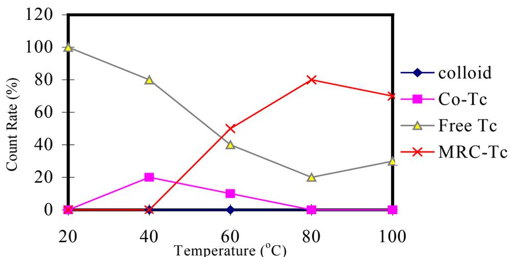
FIG. 6. Effect of temperature in labelling of MAG-3-RC-160 with  $^{99m}\text{Tc}$ .
