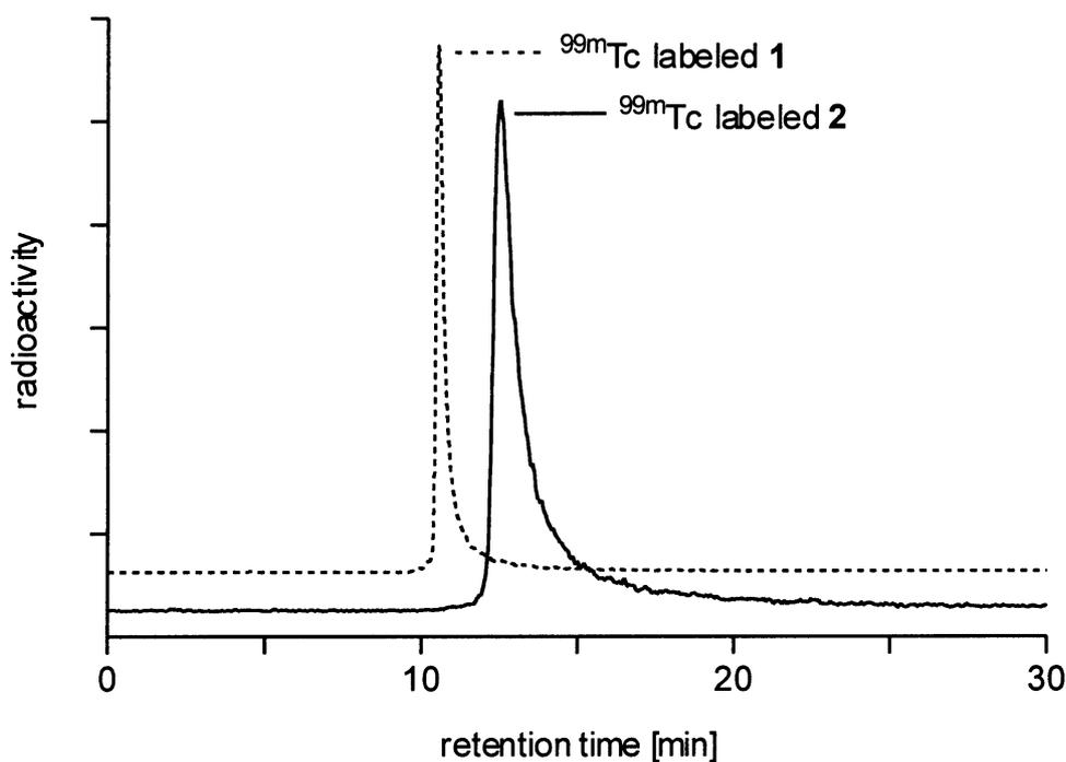
FIG. 1. Representative radiochromatograms of  $^{99m}\text{Tc}$  labelled **1** and **2**.
