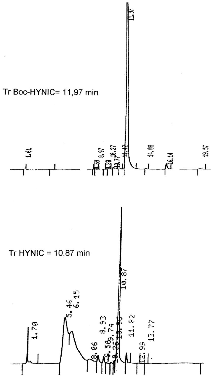
FIG. 5. HPLC profile of Boc-HYNIC and HYNIC (UV detection).
