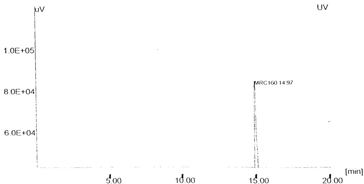
FIG. 2. HPLC chromatogram of deprotection MAG-3-RC160 (Crest Pak C-18, 5  $\mu\text{m}$ , 4.6 x 150 mm).
