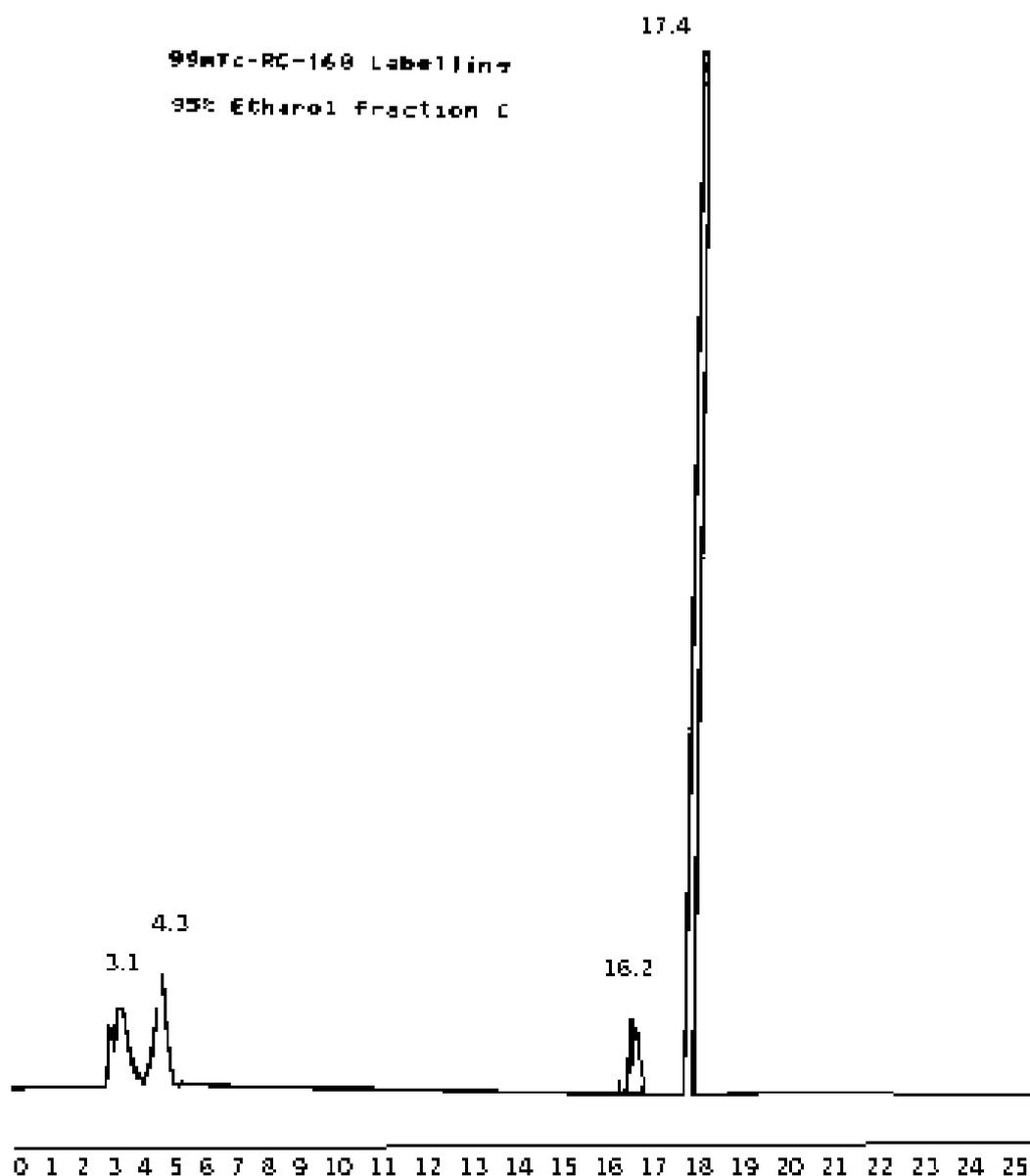
FIG. 2. HPLC Chromatogram of  $^{99m}\text{Tc}$ -RC160 in ethanol fraction C.
