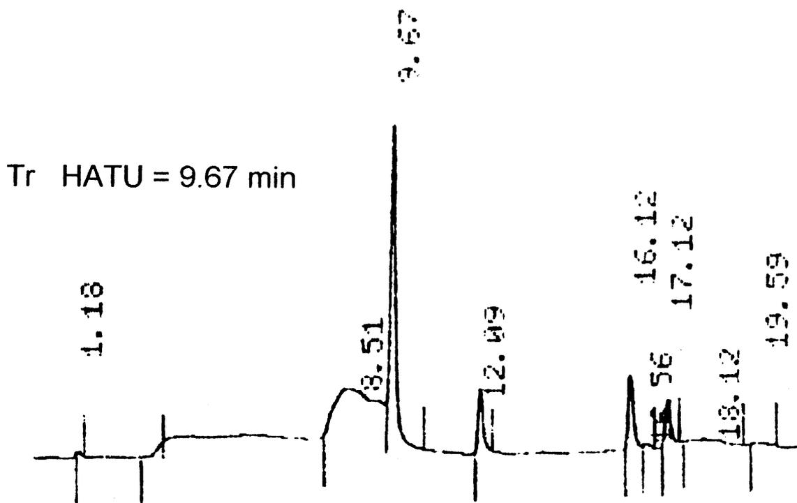
FIG. 7. HPLC profile of HATU (UV detection).
