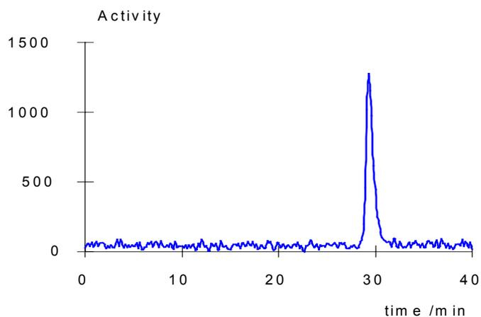
FIG. 4. Radioactivity profile of  $^{88}\text{Y}$ -DOTA-Tyr-3-Octetotide on HPLC.
