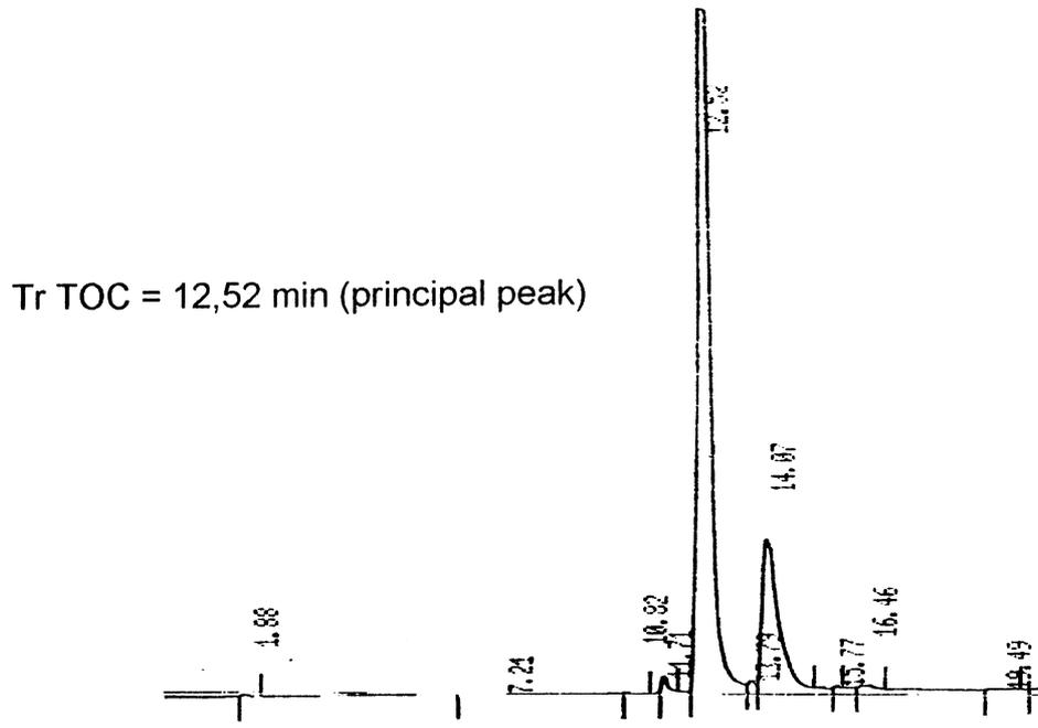
FIG. 6. HPLC profile of BOC-TOC and TOC (UV detection).
