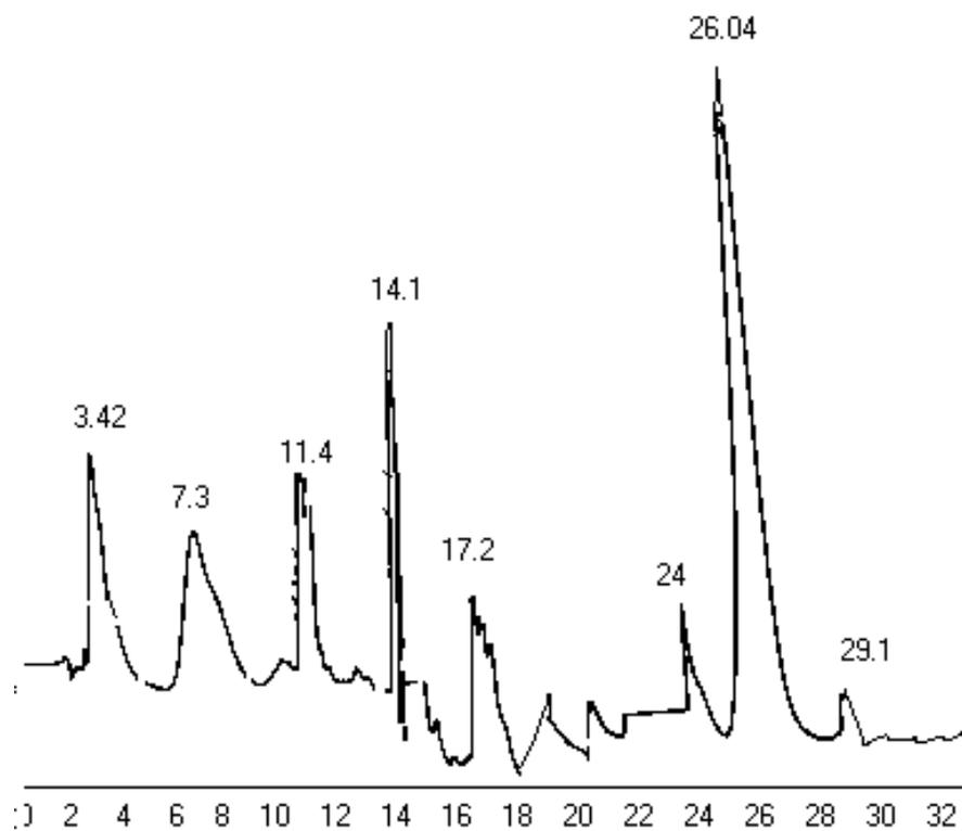
FIG. 3. HPLC chromatogram after conjugation reaction prior to purification (benzoyl MAG-3-Boc-RC-160 complex at 26 min).
