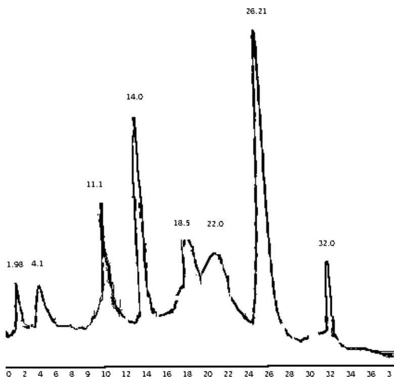
FIG. 4. HPLC chromatogram of conjugation reaction after purification (benzoyl MAG-3-Boc RC-160 complex at 26 min, Boc RC-160 at 22 min).
