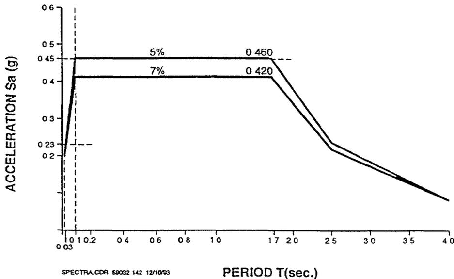
Figure 3 Kozloduy NPP Site Specific Response Spectrum
