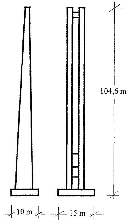
Figure 1. Flexible reinforced concrete structure: Ventilation chimney
