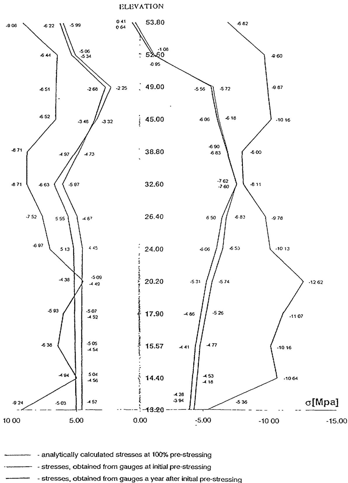
Fig. 3.7 Comparison of Stresses in Concrete Obtained from the Pre-stressing Monitoring and by the Analytical Study
