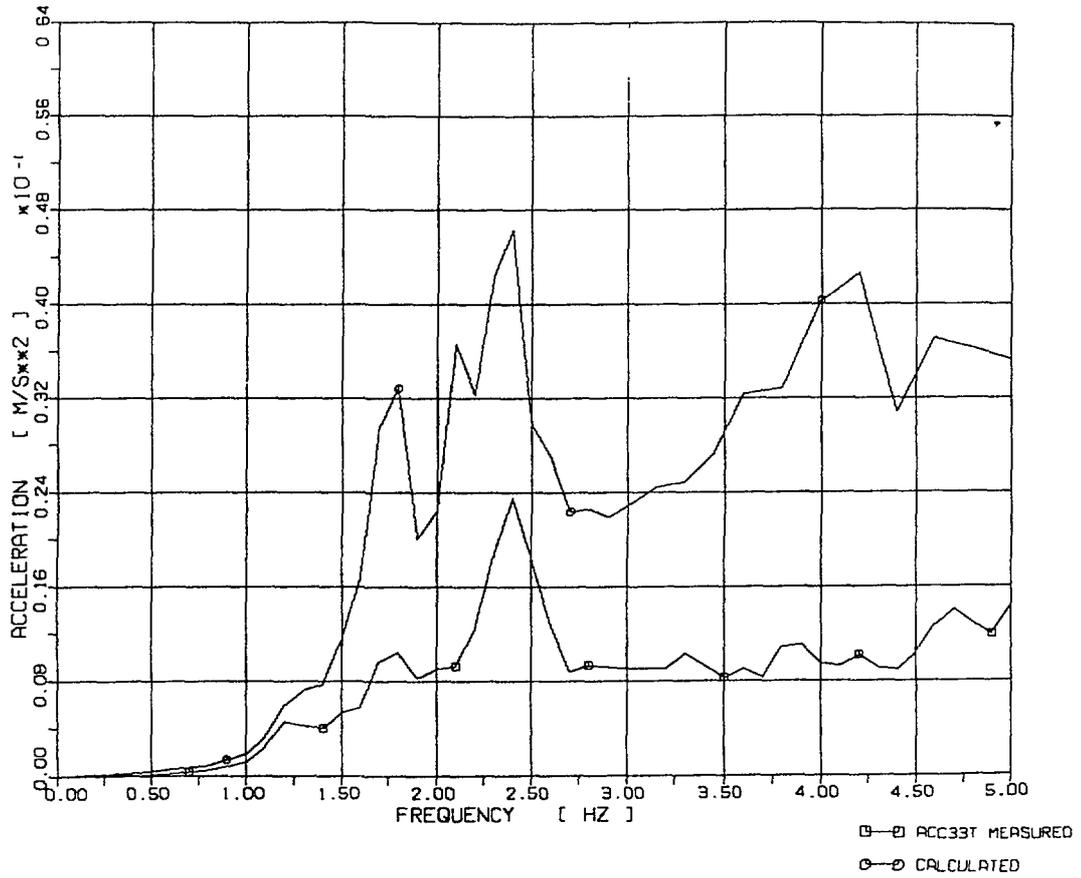
**Fig. 14 Comparison of Calculated and Measured Response Spectra, Elevation 18.9 m X2**
