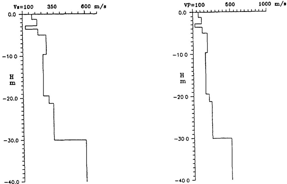
Fig.3. Velocity profiles of local geology
