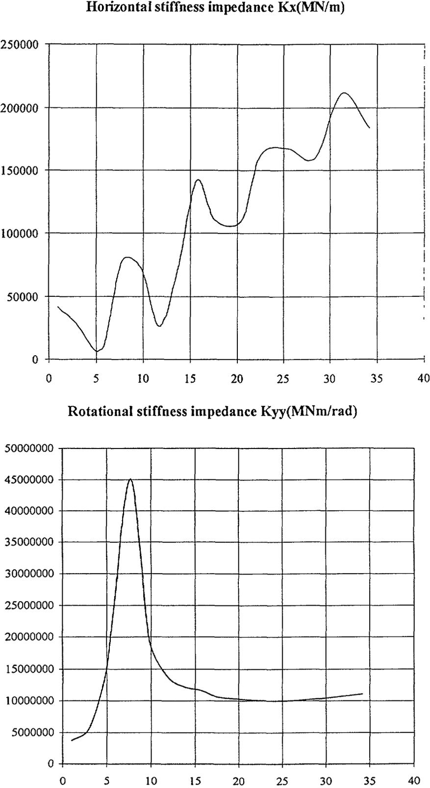
Figure 5 Examples of frequency dependent foundation stiffnesses
