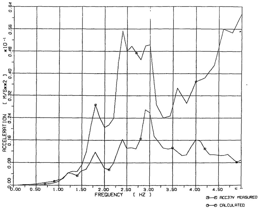
**Fig. 15 Comparison of Calculated and Measured Response Spectra, Elevation 18.9 m X3**
