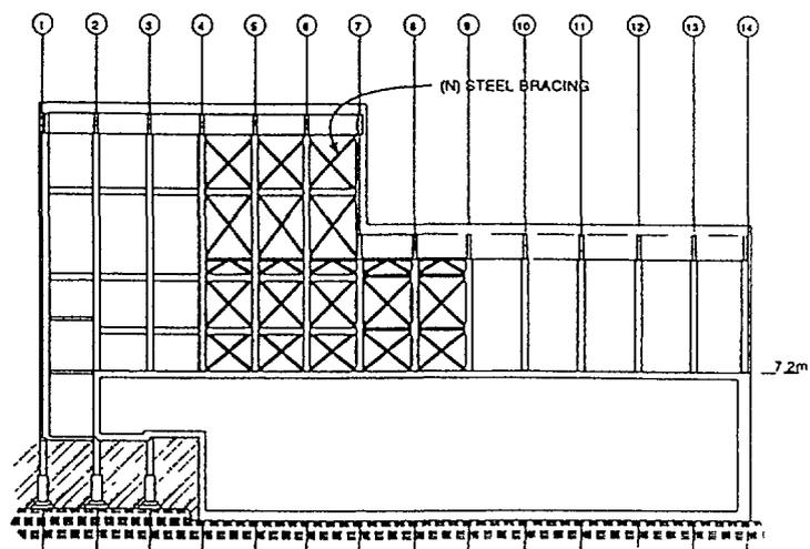
Figure 5 Longitudinal Vertical Steel Braces
