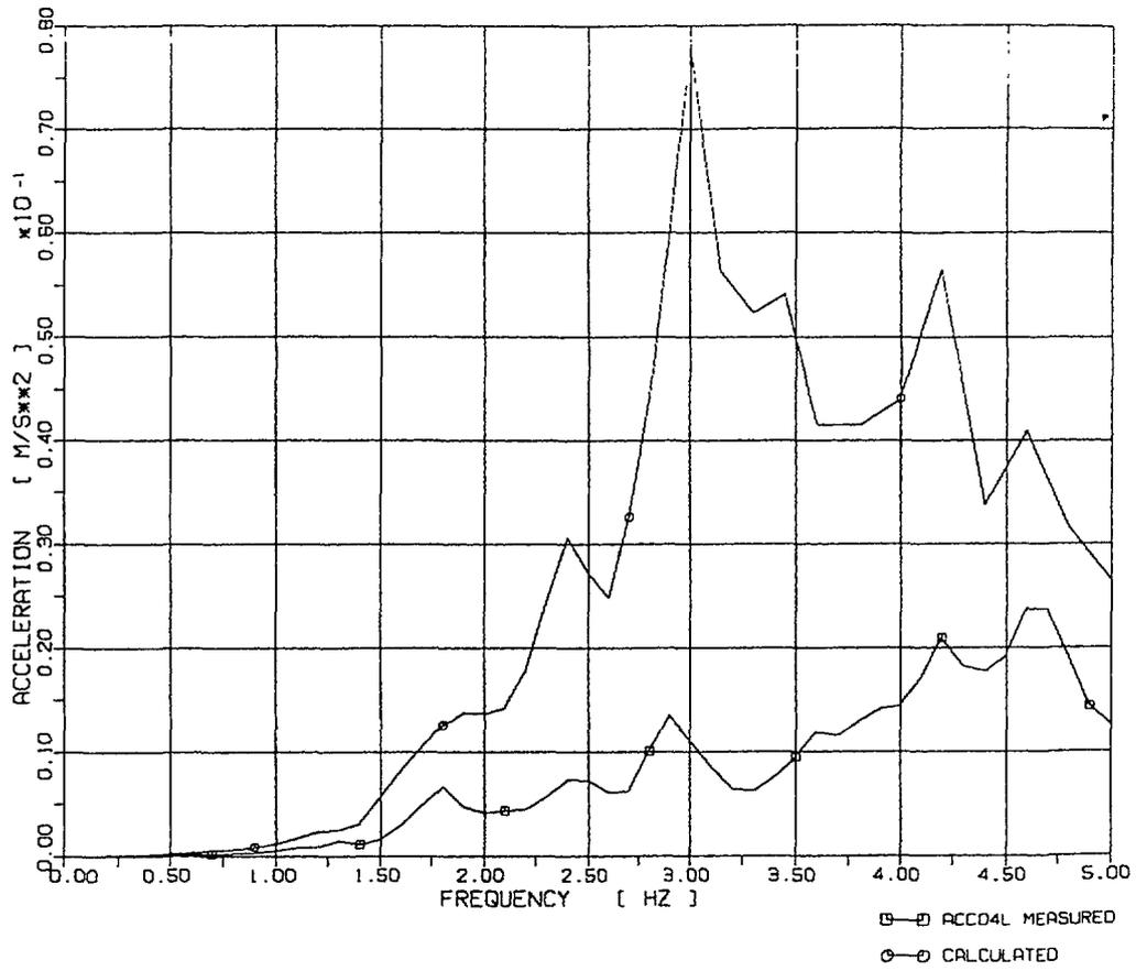
**Fig. 10 Comparison of Calculated and Measured Response Spectra, Foundation Level X1**
