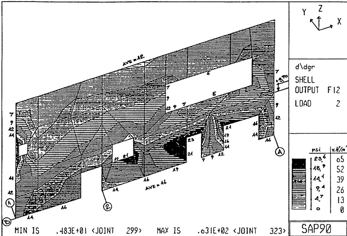
Figure 8: In Plane Shear Stress Iso Contour
