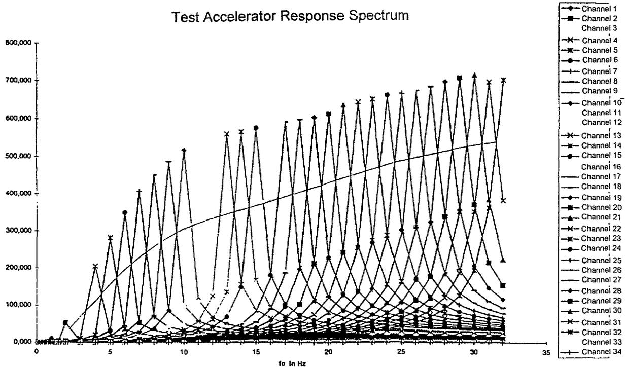
Figure 3: Enveloping of Single Frequency TRS
