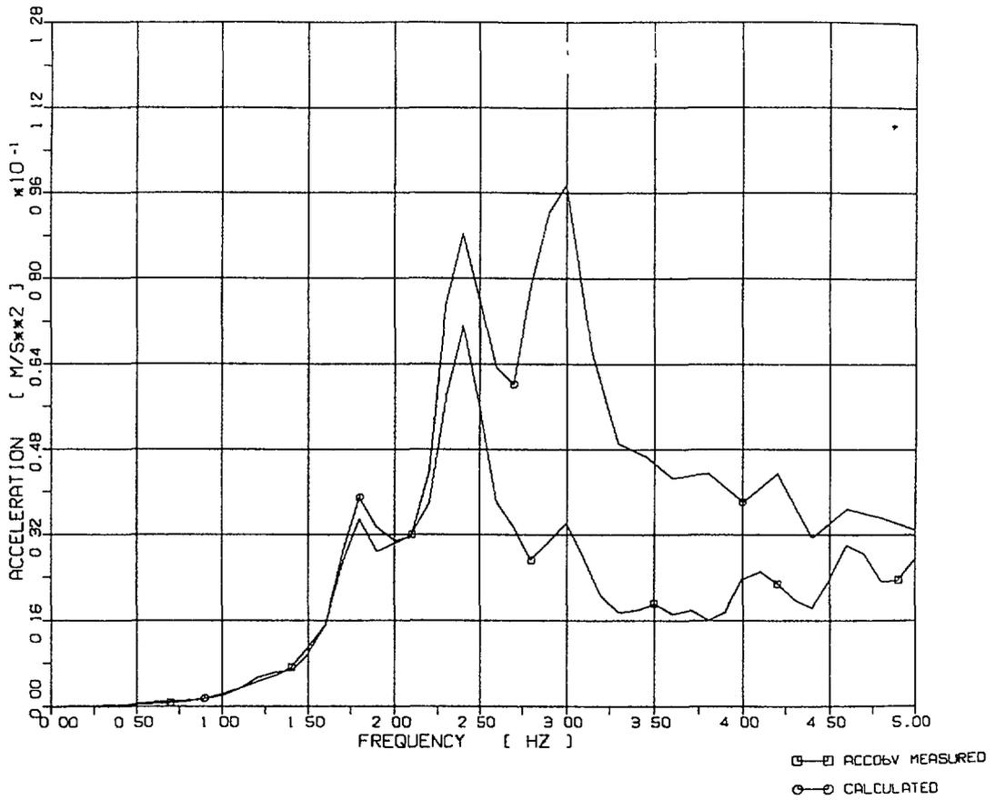
**Fig. 12 Comparison of Calculated and Measured Response Spectra, Foundation Level X3**
