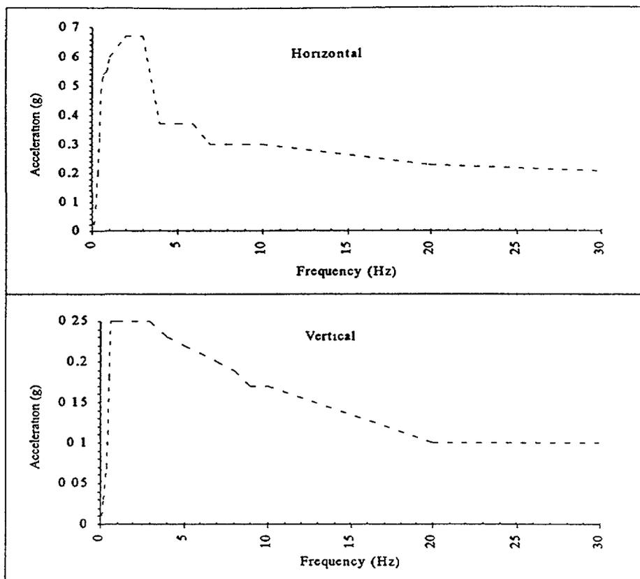
Fig 3 5 In-structure Response Spectra at Elevation +13 20
