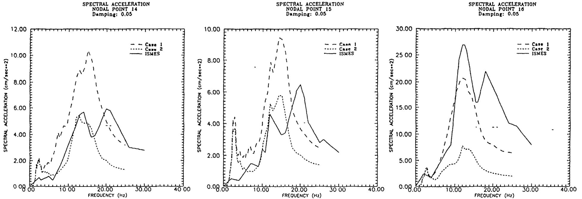
Fig.6. Comparison between analytical and measured response at foundation level
