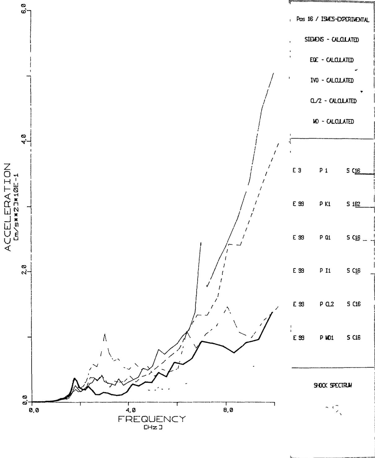
Fig. 14 Comparison between experimental and calculated response spectra at 2% damping ratio in position 16 (frequency range from 1 to 10 Hz)
