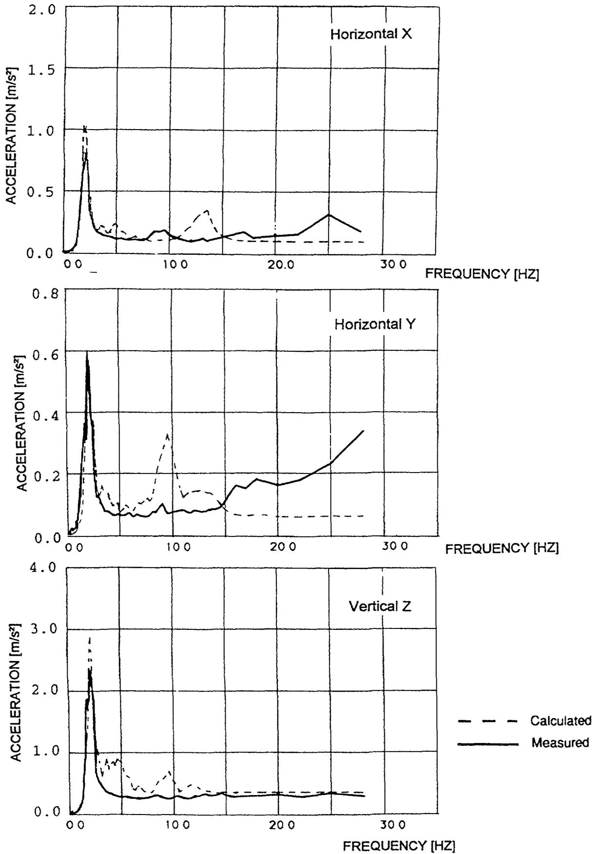
**Fig. 18 Comparison of Floor Response Spectra ( $D = 2\%$ ) at the Elevation 18.9 m (Test I / S, 500 kg)**
