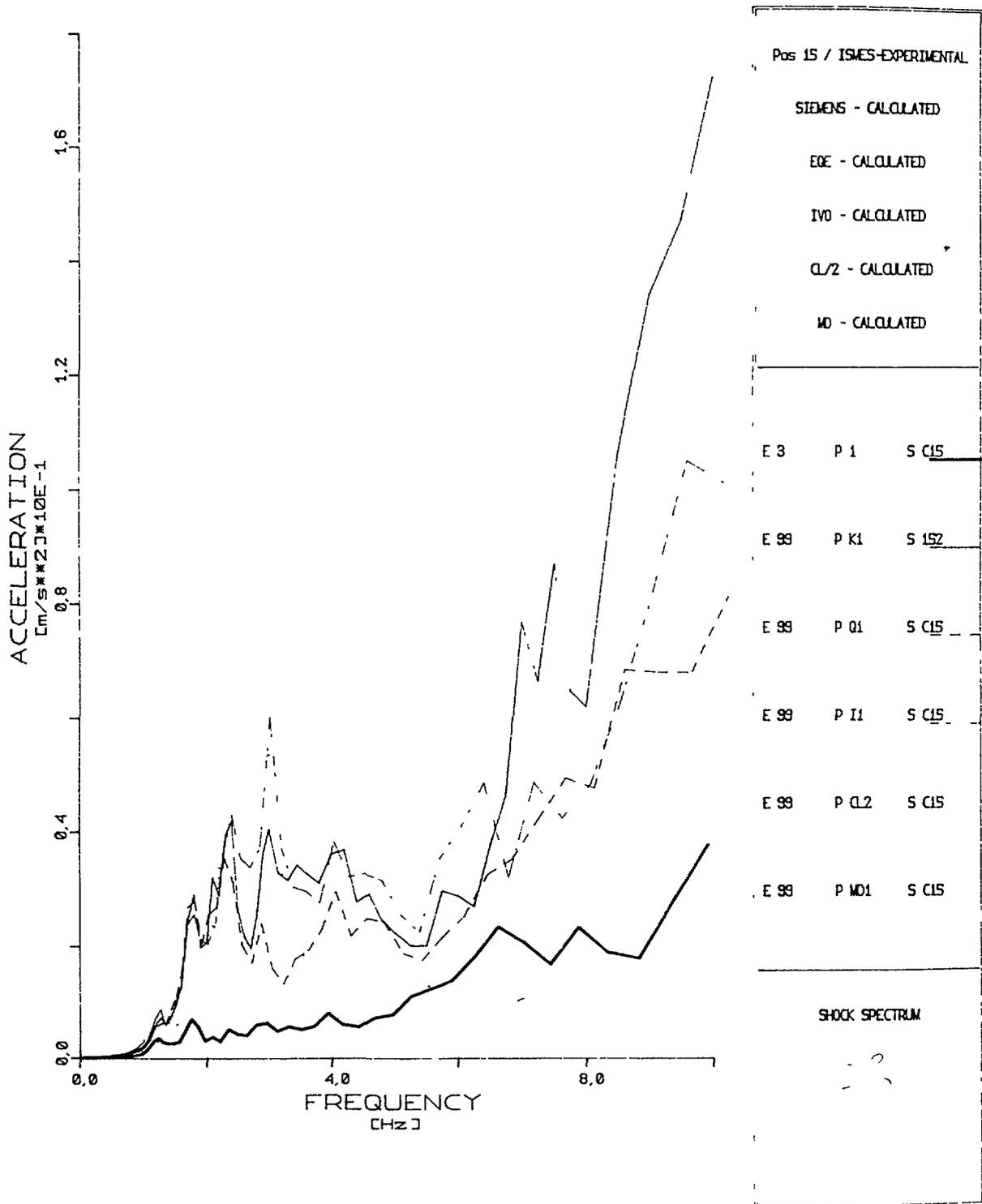
Fig. 13 Comparison between experimental and calculated response spectra at 2% damping ratio in position 15 (frequency range from 1 to 10 Hz)
