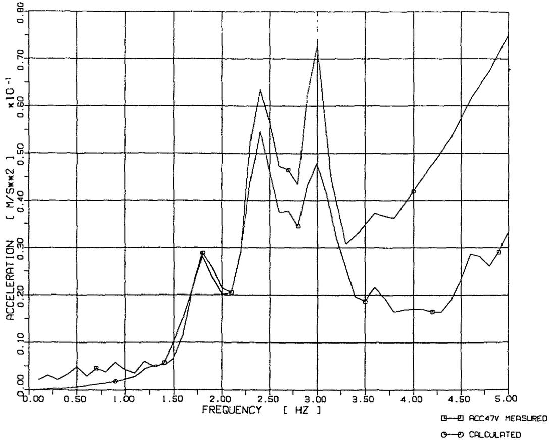
**Fig. 17 Comparison of Calculated and Measured Response Spectra, Elevation of Crane Support X3**
