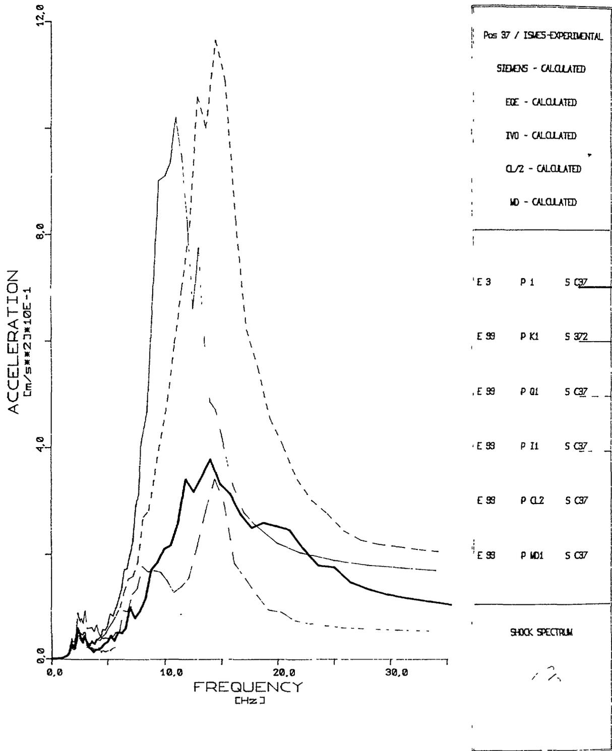
Fig. 11 Comparison between experimental and calculated response spectra at 2% damping ratio in position 37 (frequency range from 1 to 35 Hz)
