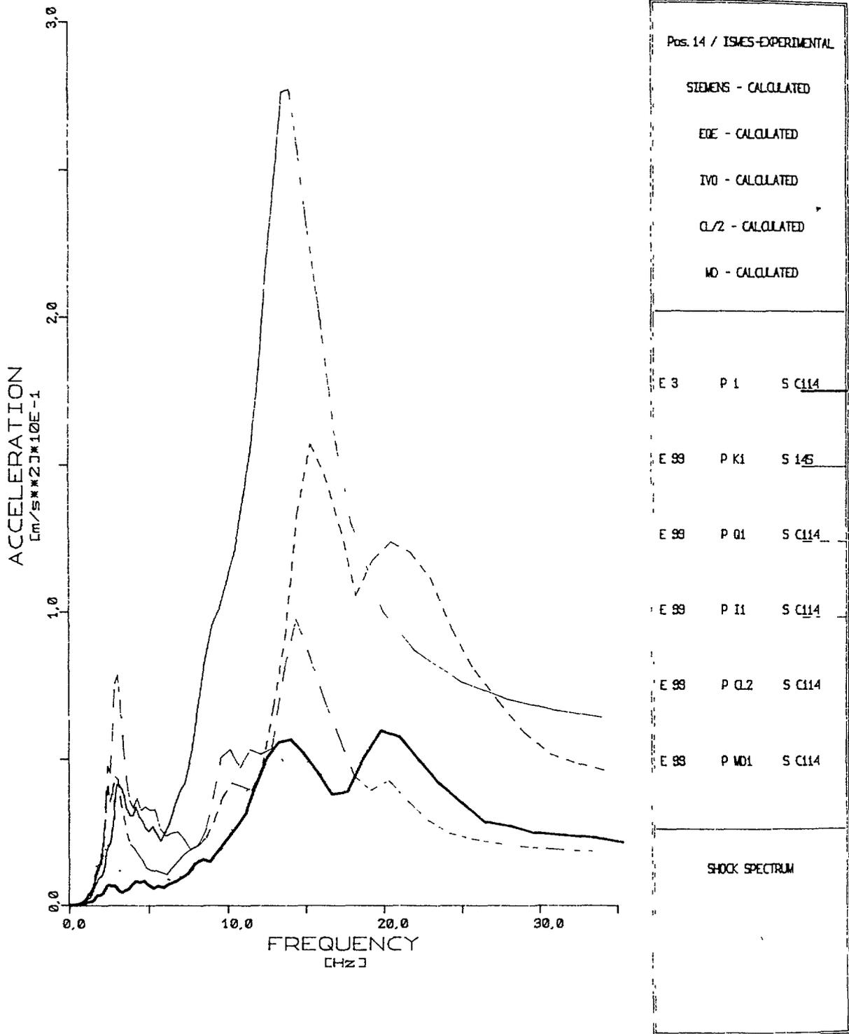
Fig. 6 Comparison between experimental and calculated response spectra at 5% damping in position 14 (frequency range from 1 to 35 H)
