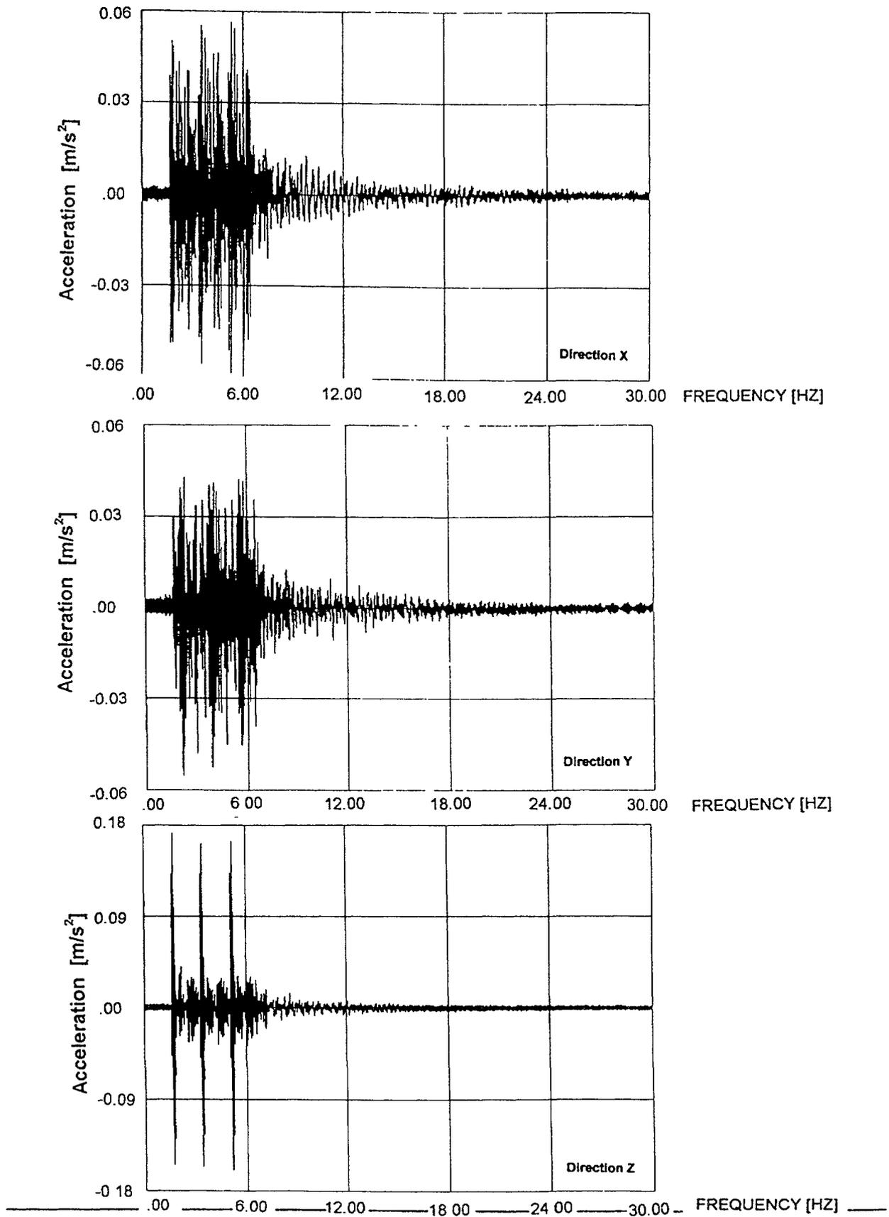
**Fig. 5 Free-Field Acceleration Time Histories nearby the Reactor Building (Test 12/94,FF 3x 100 kg with Delay)**
