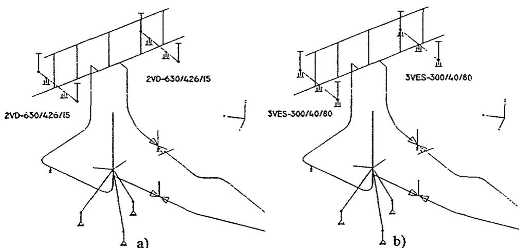
Figure 7 HVD location for Loop No 1 of PCLS
