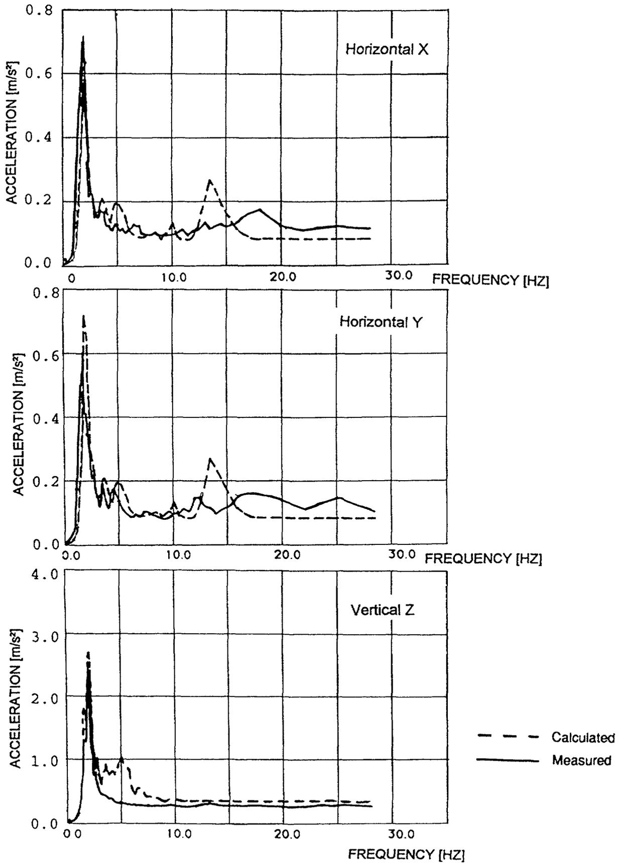
Fig. 19 Comparison of Response Spectra ( $D = 2\%$ ) at Foundation Level (Test I / S, 500 kg)
