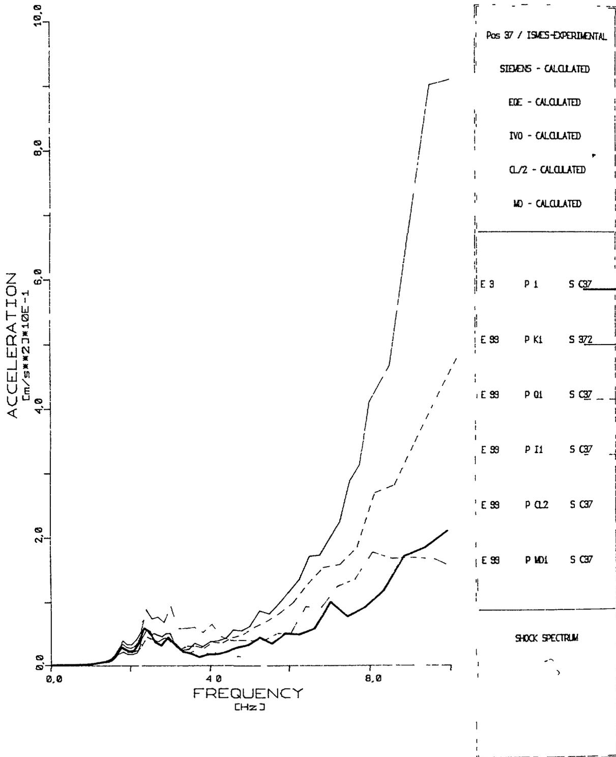
Fig. 17 Comparison between experimental and calculated response spectra at 2% damping ratio in position 37 (frequency range from 1 to Hz)
