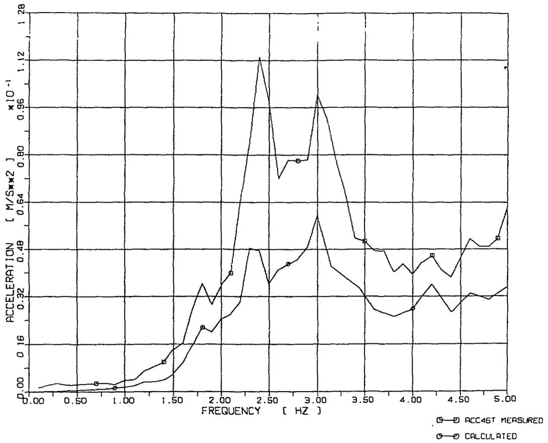
**Fig. 16 Comparison of Calculated and Measured Response Spectra, Elevation of Crane Support X2**
