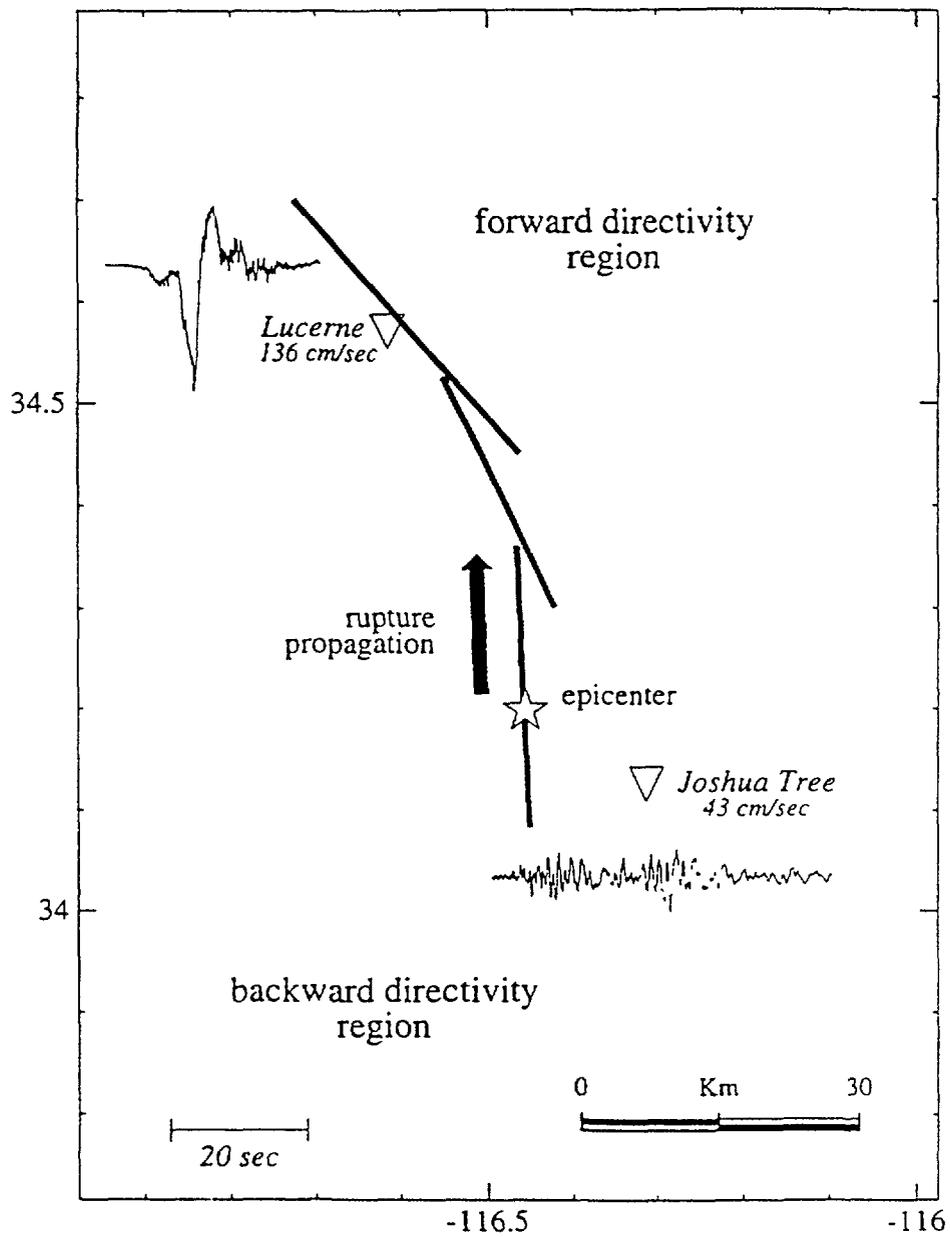
Fig 7 Map of the Landers region showing the main features of the 1992 Landers earthquake, which occurred on three fault segments. the epicenter and the location of the recording stations at Lucerne and Joshua tree ( From Somerville et al, 1997)
