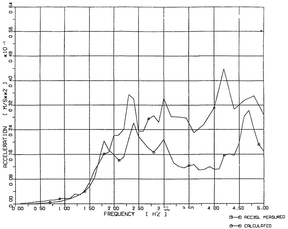
**Fig. 13 Comparison of Calculated and Measured Response Spectra, Elevation 18.9 m X1**
