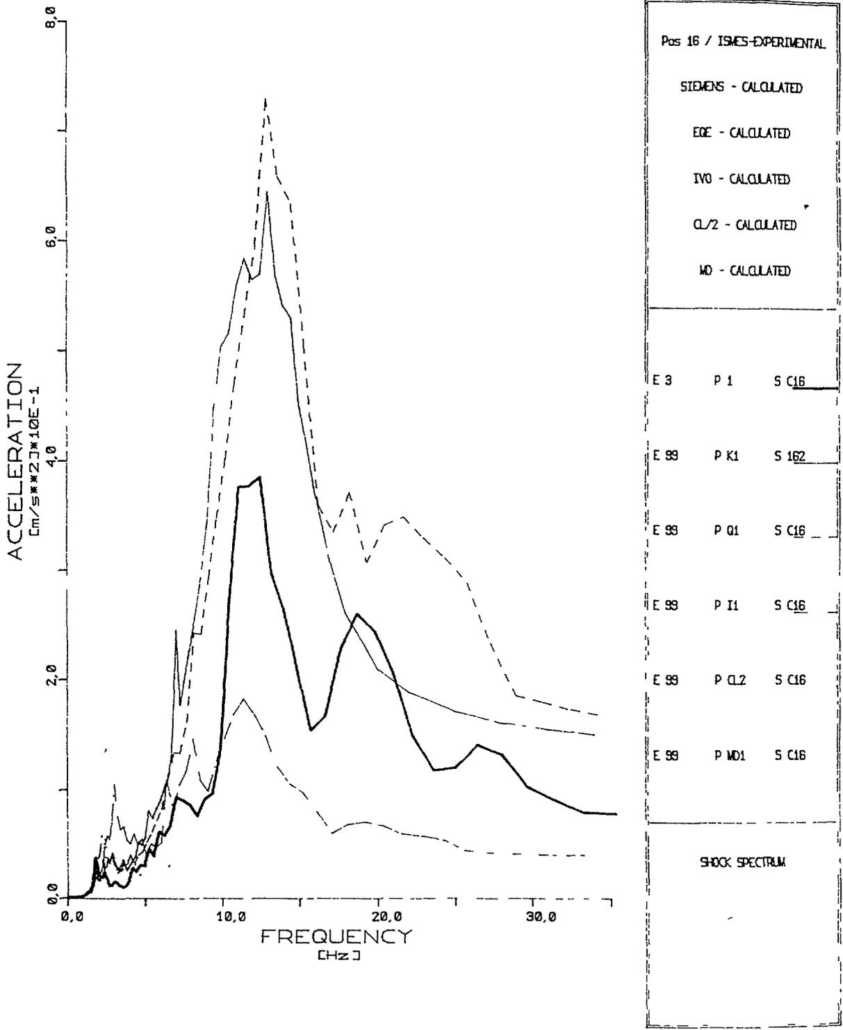
Fig. 8 Comparison between experimental and calculated response spectra at 2% damping in position 16 (frequency range from 1 to 35 Hz)
