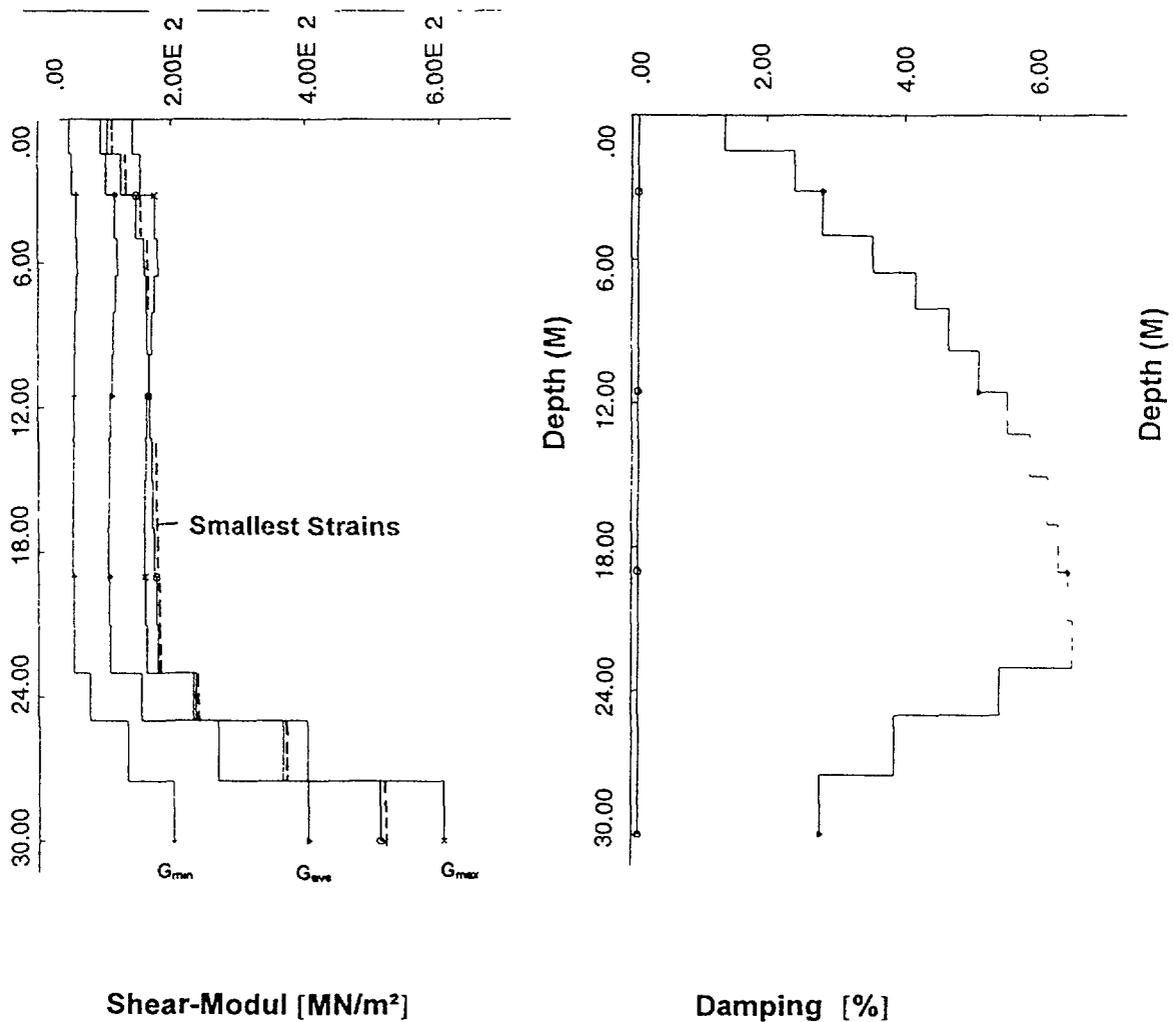
**Fig. 3 Strain Compatible Shear Module and Damping**
