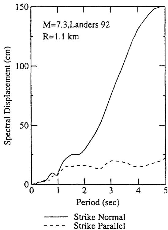
Fig 8 Directivity effects during 1992 Landers earthquake top records at stations in forward and backward directivity regions. bottom strike-normal and strike-parallel spectral displacements at Lucerne (From Somerville 'et al', 1997)
