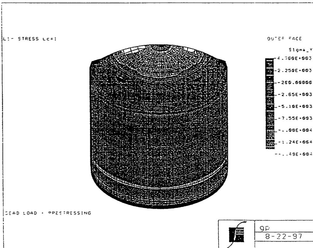
Fig. 4.3 Longitudinal Stresses at the Containment Due to Dead Load and Pre-stressing
