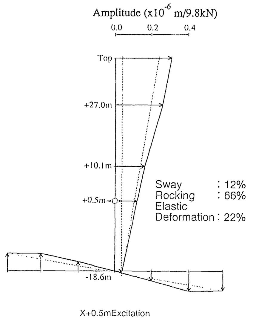
Fig.5 Vibration mode shapes of Atucha II reactor building ( $f=3.5\text{Hz}$ )
