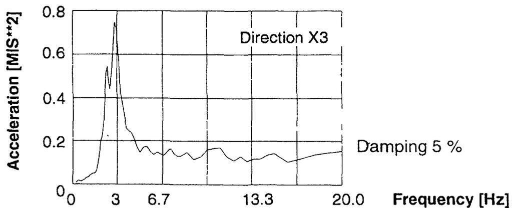
**Fig. 8 Free-Field Response Spectra at 240 m from the line Reactor Building (Test 90/91, 1x 500 kg without Delay)**
