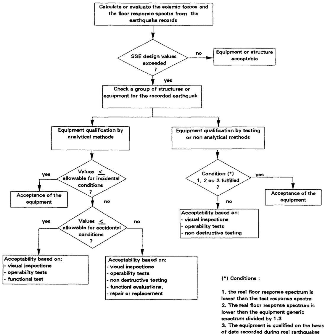
**Figure 6 - Long Term Evaluation Procedure**
