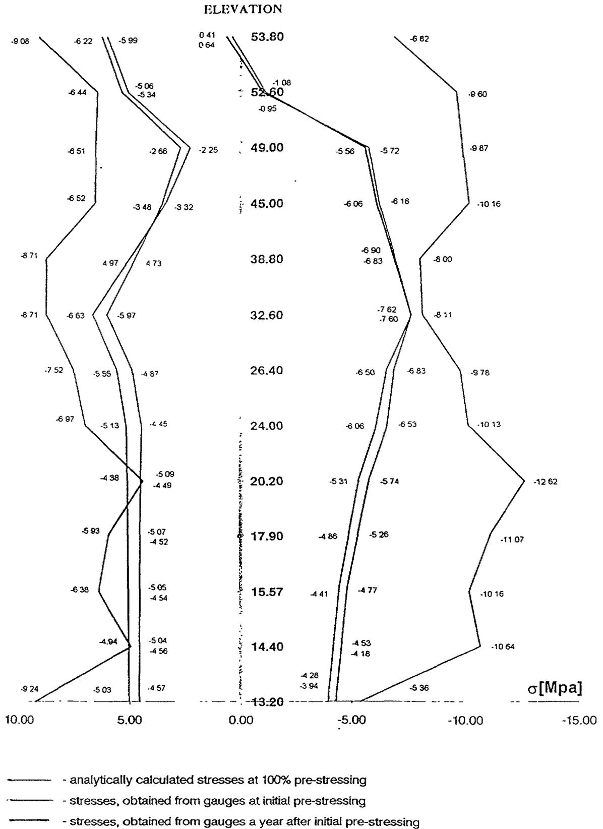
Fig. 3 8 Comparison of Stresses in Concrete Obtained from the Pre-stressing Monitoring and by the Analytical Study
