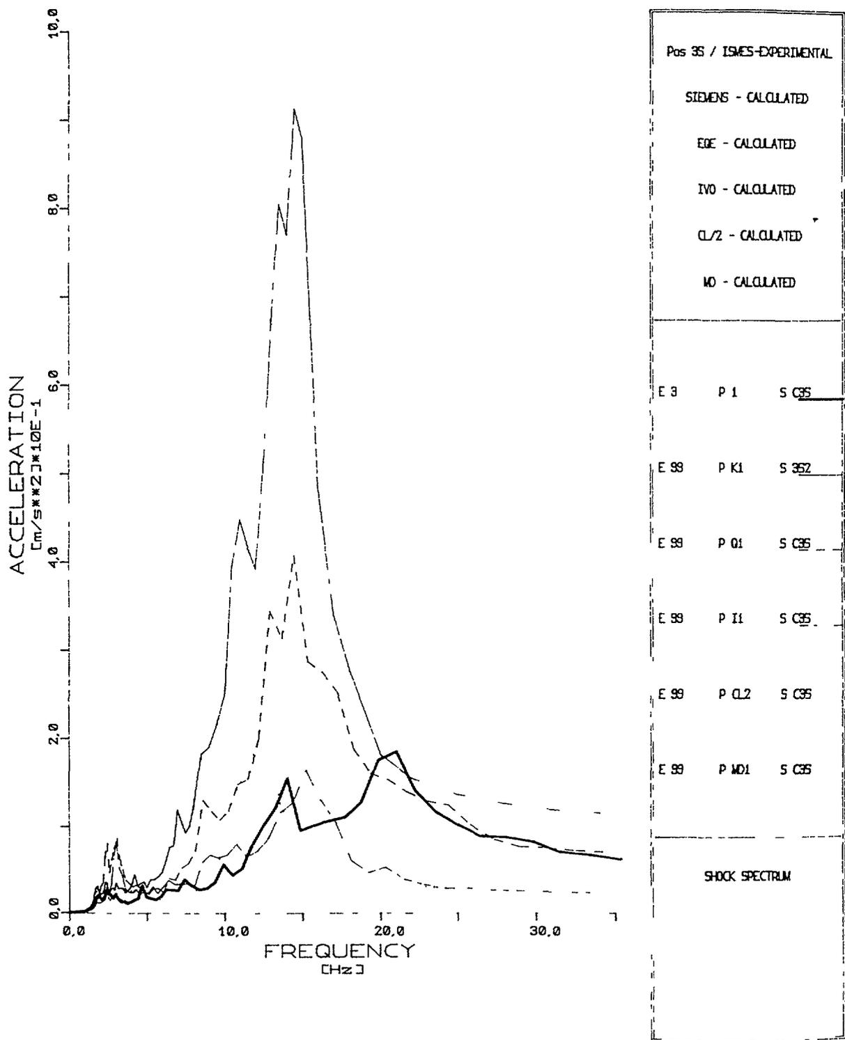
Fig. 9 Comparison between experimental and calculated response spectra at 2% damping in position 35 (frequency range from 1 to 35 Hz)
