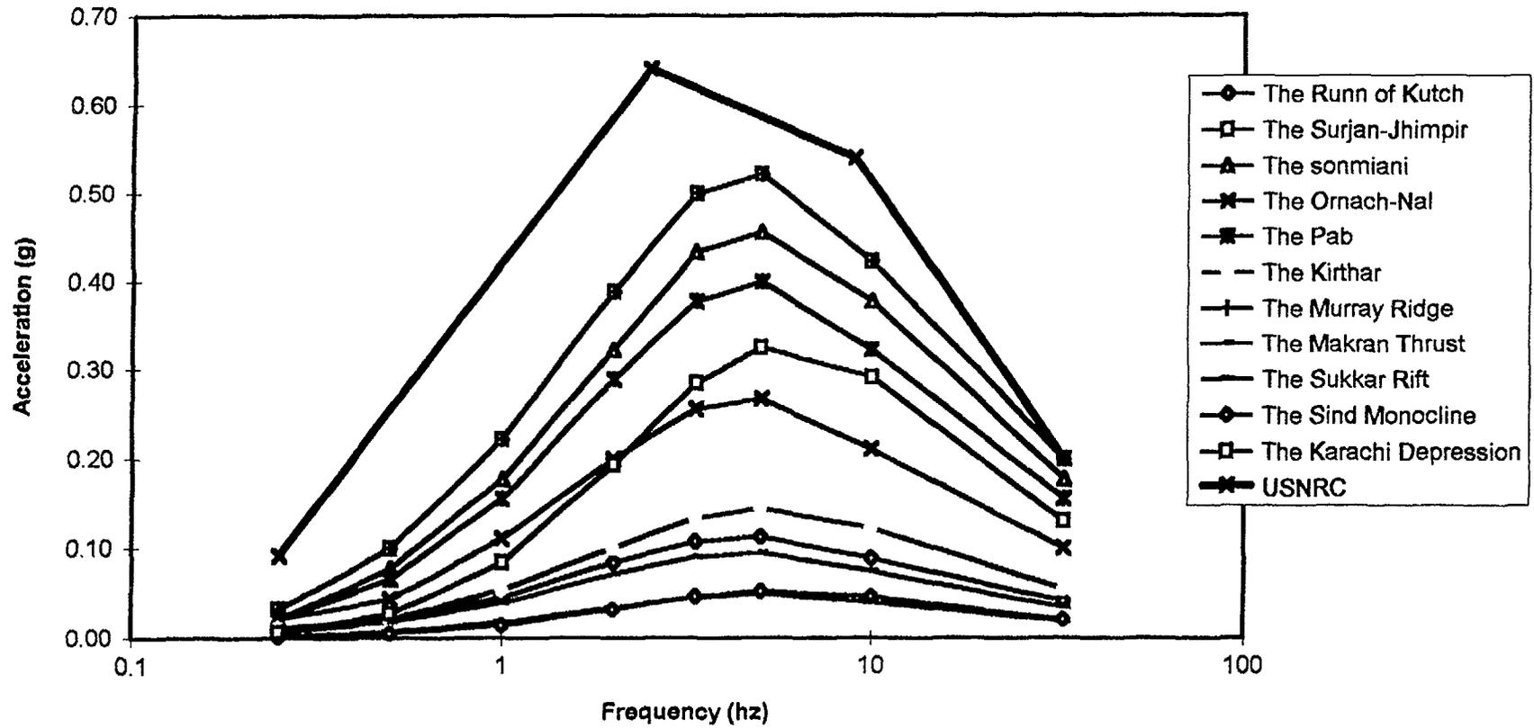
**FIG. 4 Peak Ground Acceleration at KANUPP due to maximum credible earthquakes at different zones**
