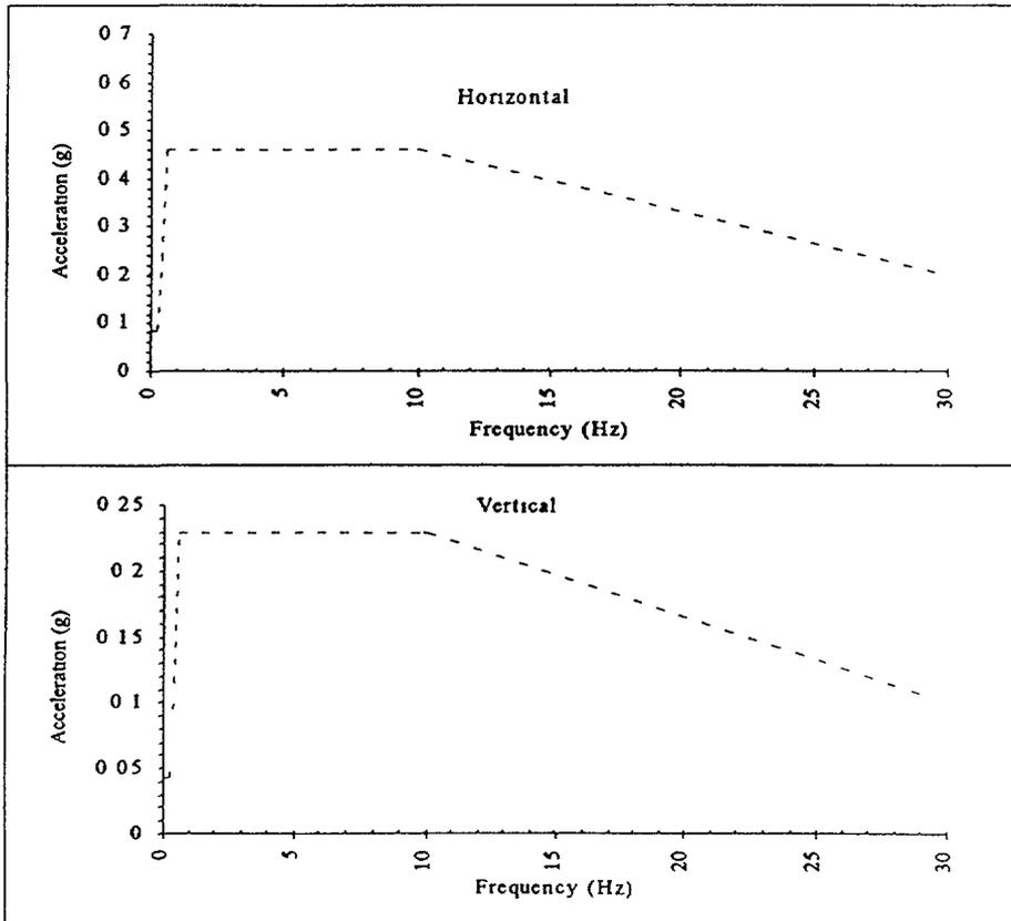
Fig 3 4 Free Field Response Spectra
