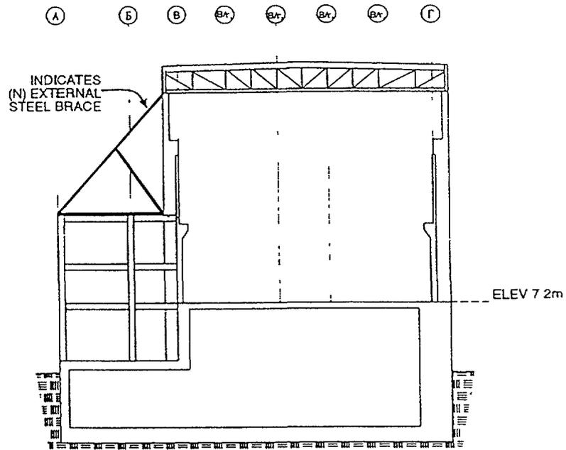
Figure 4 Transverse External Steel Brace at High-Bay Section
