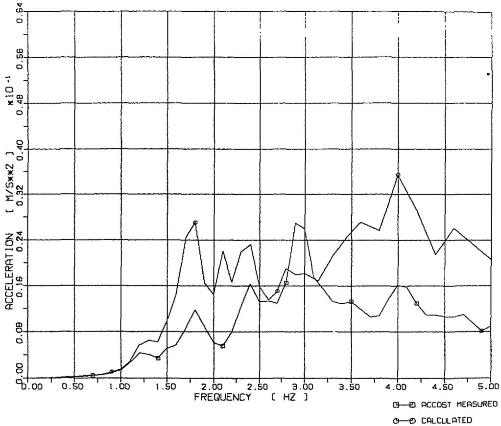
**Fig. 11 Comparison of Calculated and Measured Response Spectra, Foundation Level X2**
