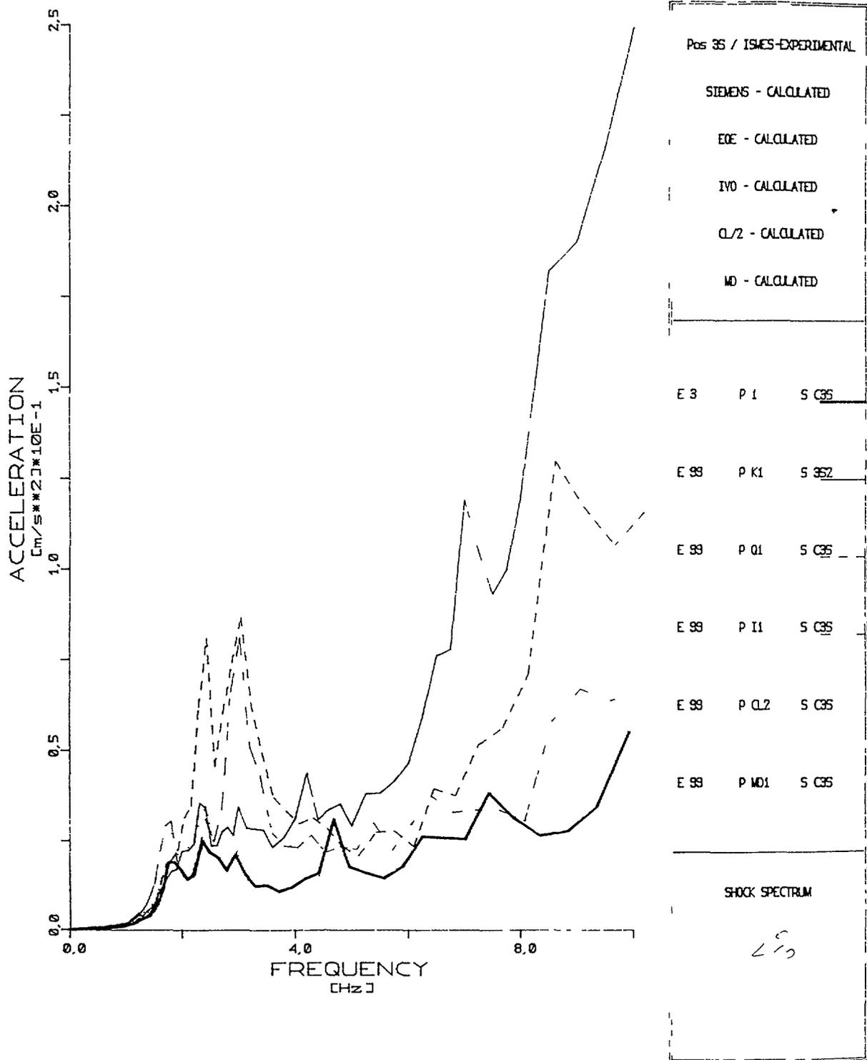
Fig. 15 Comparison between experimental and calculated response spectra at 2% damping ratio in position 35 (frequency range from 1 to 10 Hz)
