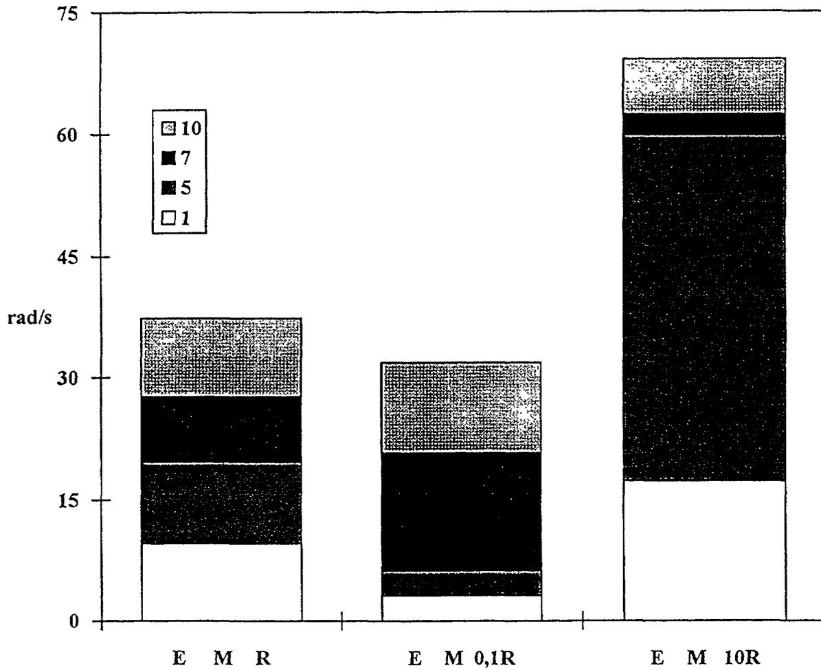
Figure 13. Location of the first ten natural circular frequencies at auxiliary building concrete block
