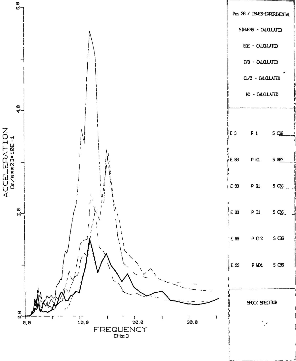
Fig. 10 Comparison between experimental and calculated response spectra at 2% damping ratio in position 36 (frequency range from 1 to 35 Hz)
