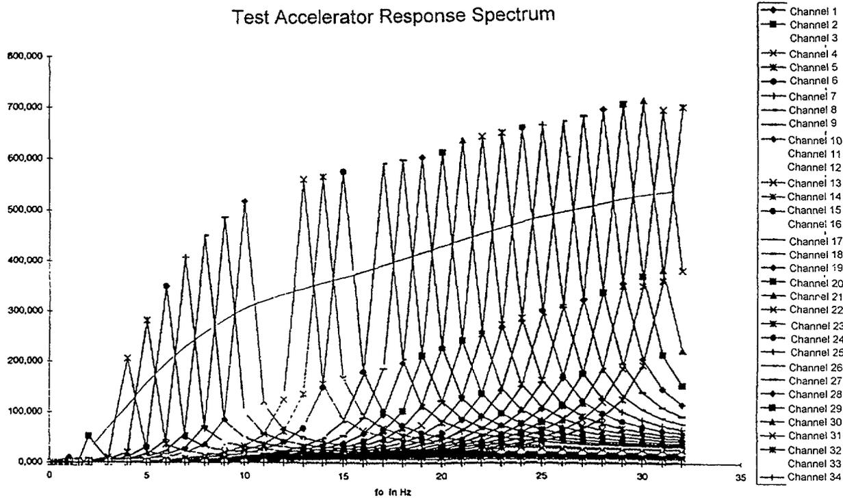
Figure 2: Enveloping of Single Frequency TRS
