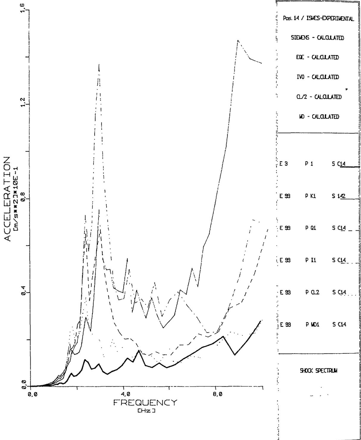
Fig. 12 Comparison between experimental and calculated response spectra at 2% damping ratio in position 14 (frequency range from 1 to 10 Hz)
