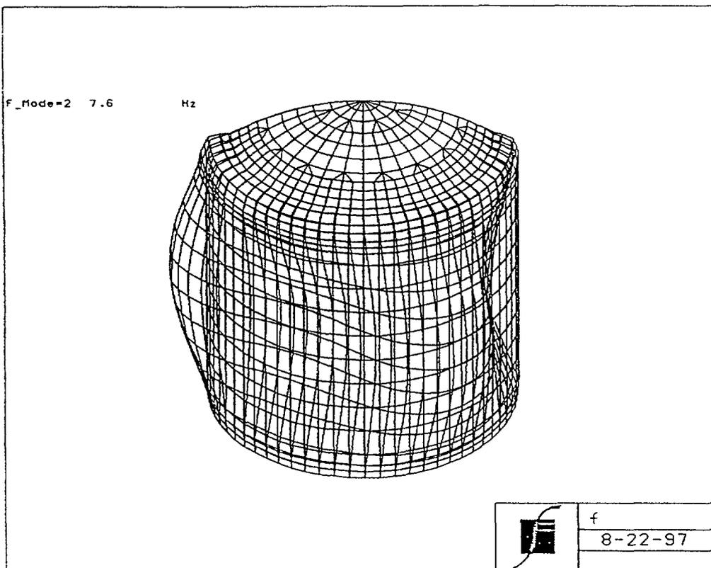
Fig. 3.6 Mode Shape 1, F1=4.6 Hz, Mode Shape 2, F2=7.6 Hz
