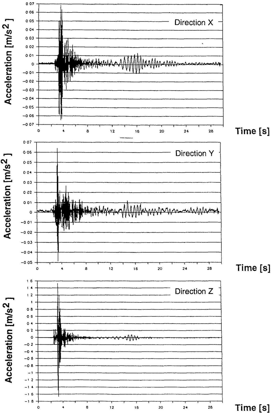
Fig. 7 Free-Field Acceleration Time Histories at 240 m from the Reactor Building (Test 90/91, 1x 500 kg without Delay)
