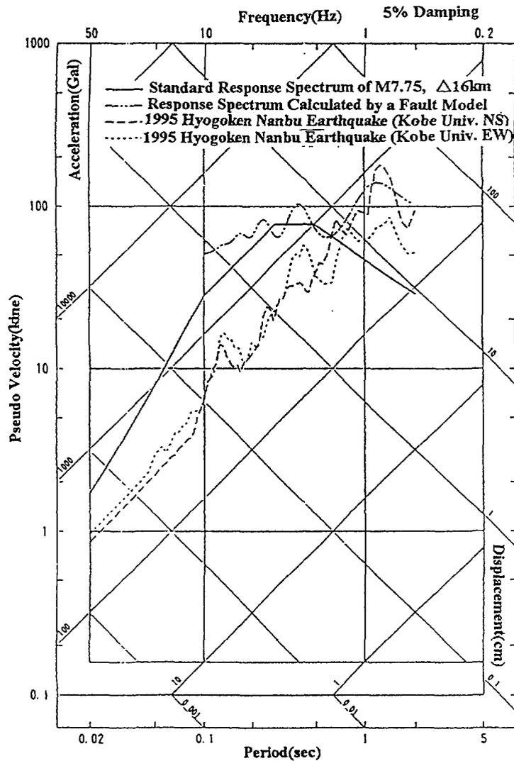
Fig.8 Comparison of a Standard Design Response Spectrum with the Response Spectra of Observed Earthquake Records and the Response Spectrum calculated using a Fault Model.
