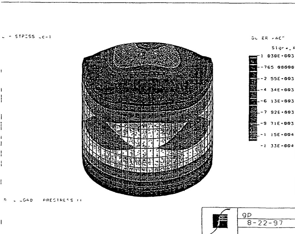
Fig 4.2 Hoop Stresses at the Containment Due to Dead Load and Pre-stressing
