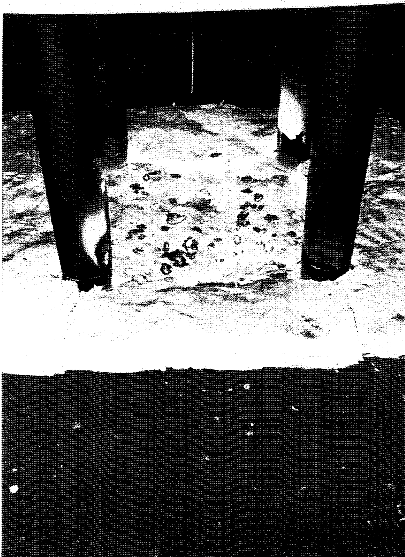
FIG. I-6. The melt surface between four carbon electrodes during ISV trial. (Photograph courtesy of Geosafe Australia.)
