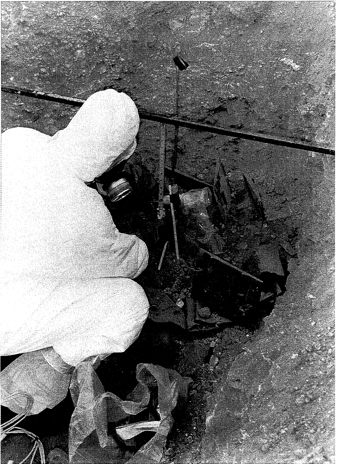
FIG. I-7. Plutonium contaminated steel plate being positioned for an intermediate scale ISV trial. (Photograph courtesy of Geosafe Australia.)
