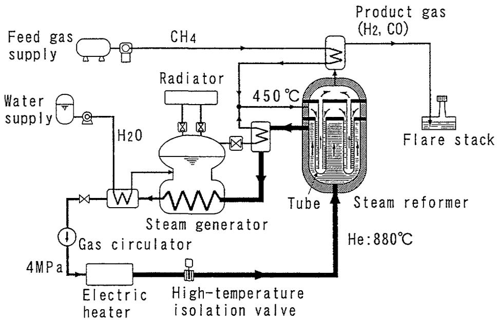
Fig. 4 Flow scheme of out-of-pile test facility.
