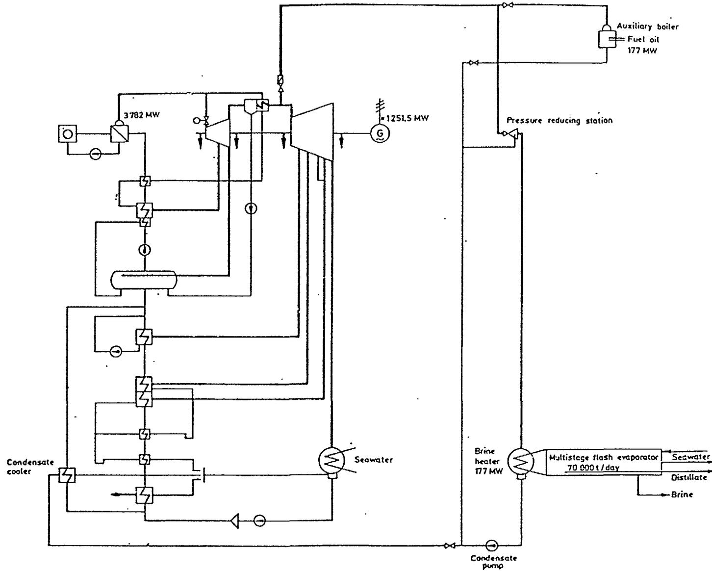
Fig. 2. Combination of a nuclear power plant (PWR) with a desalination plant (MSF) (Option B).
