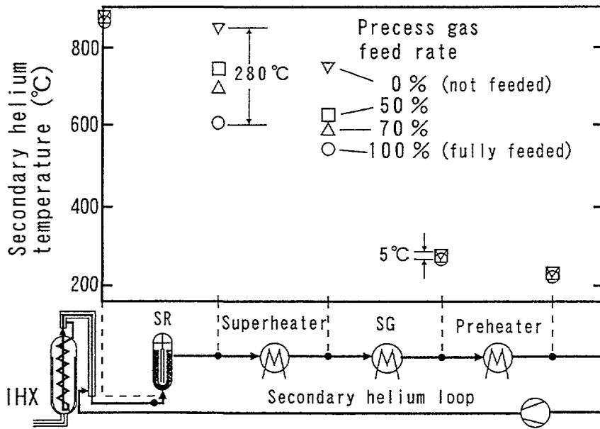
Fig. 3 Change of secondary helium gas temperature at main components for process gas feed rate of 0 to 100%.
