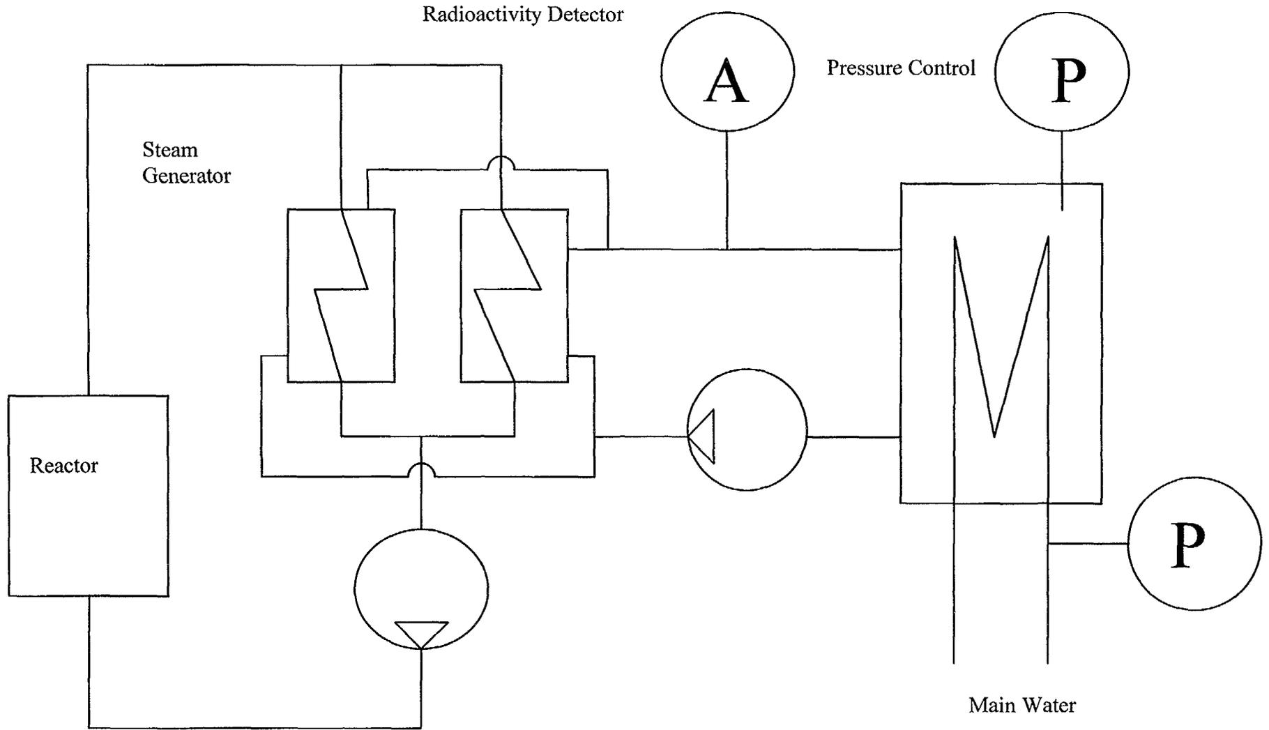
Fig.1 Schematic Diagram of the First NPP's Heat Utilization
