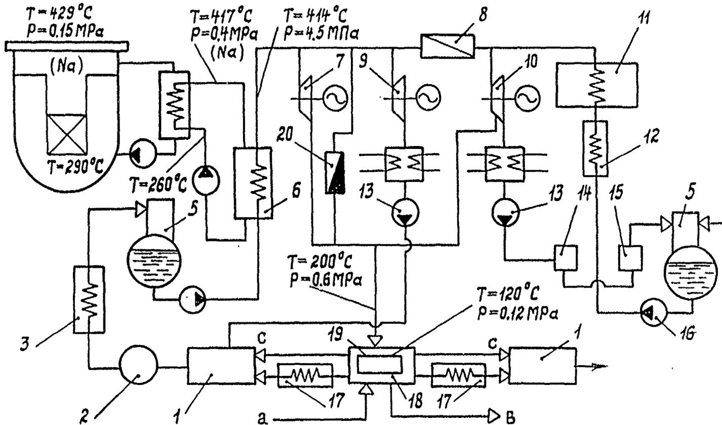
1 - water preparation facilities, 2 - vacuum deaerators, 3 - desalted water heater, 4 - feed pumps,
