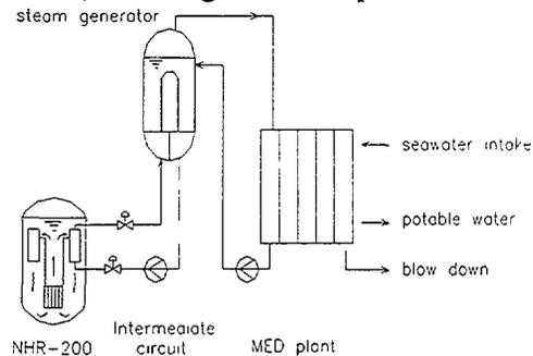
Fig 2 Simplified system diagram of water production only
