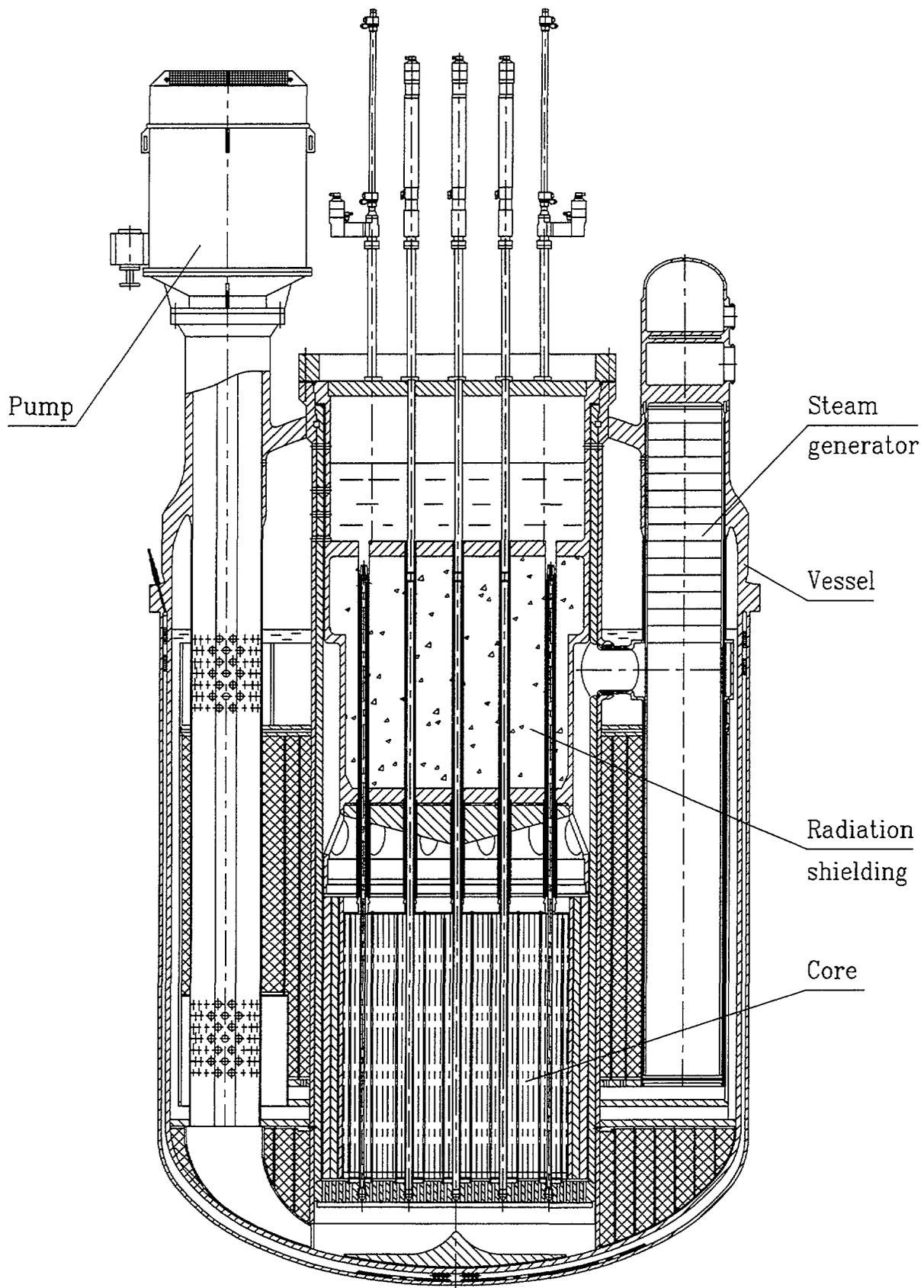
Figure 1. Reactor plant of enhanced safety with liquid-metal coolant.
