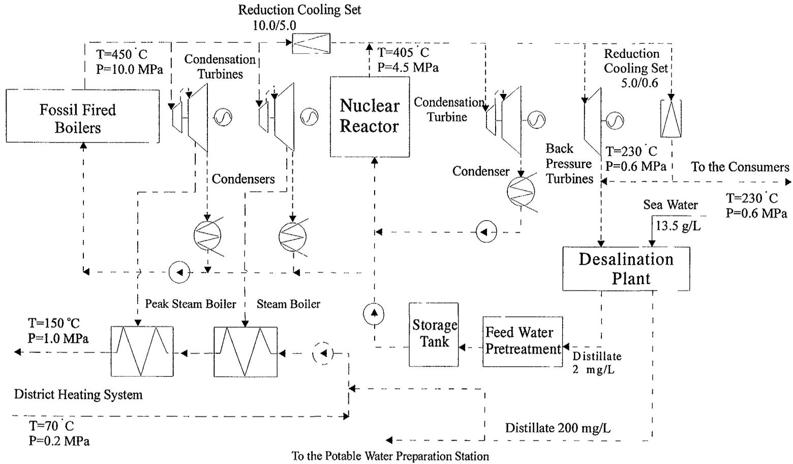
FIG. 7. Principle flow diagram of Mangyshlak Atomic Energy Complex.
