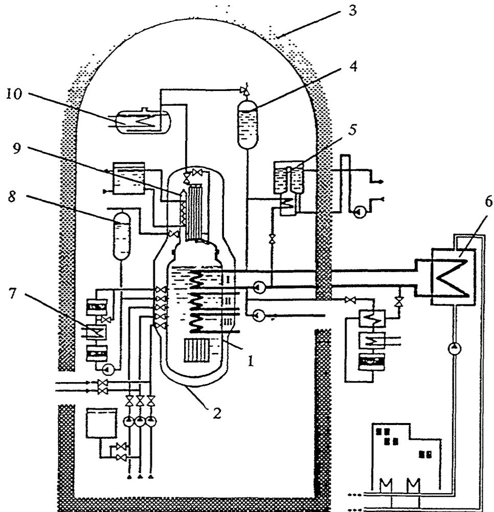
1 - reactor, 2 - guard vessel, 3 - containment, 4 - pressurizer, 5 - RHR HX,
