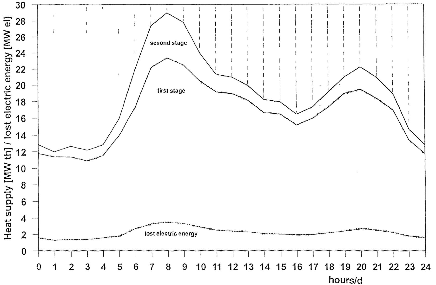
Fig. 10 Heat Supply on March 5, 1991. The Contribution of the first stage (1) of Heat Extraction is reaching 60 percent
