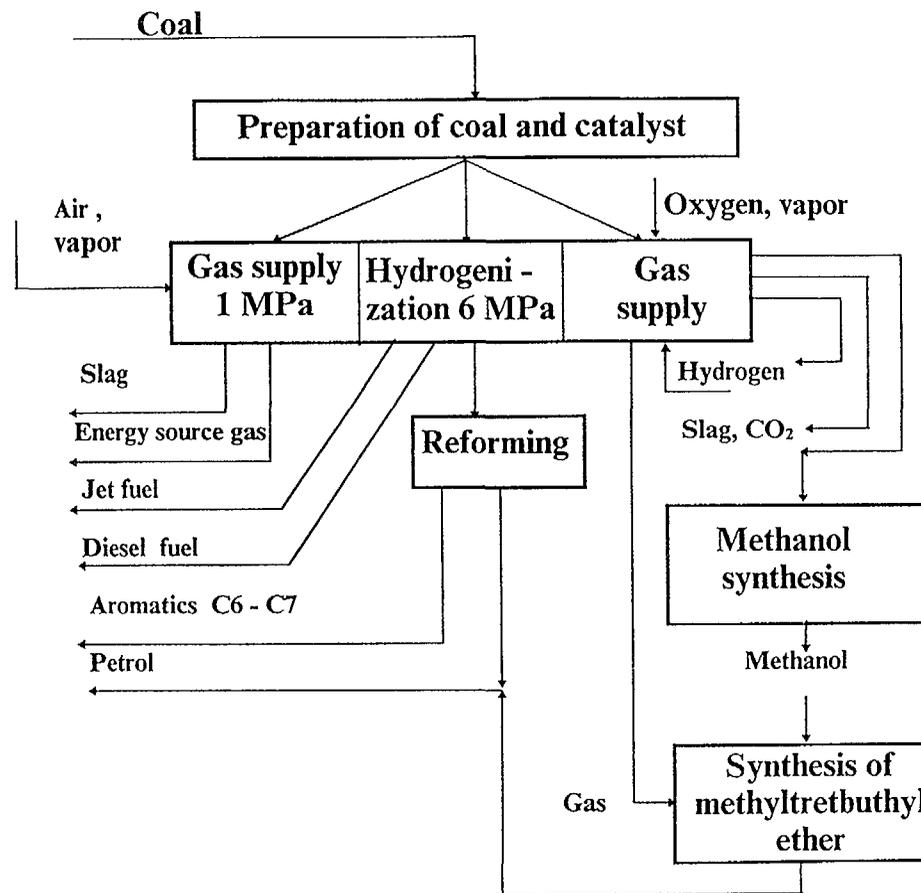
Fig. 3 Flow chart of obtaining fuel and chemical products from coal
