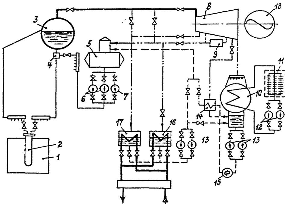
1 - reactor, 2 - fuel channel, 3 - steam drum, 4 - mixing device, 5 - deaerator, 6 - feed pumps, 7 - emergency feed pump, 8 - turbine, 9 -separator, 10 - condenser, 11 - air coolers, 12 - circulating pumps, 13 - condensate pumps, 14 - low pressure reheater, 15 - ion-exchange filter, 16 - main grid heater, 17 - peak heater, 18 - generator.
