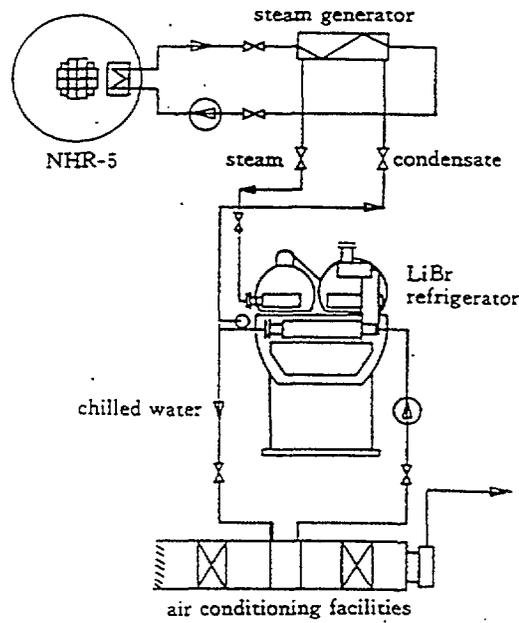
Fig. 11 Schematic diagram of an NHR air-conditioning system
