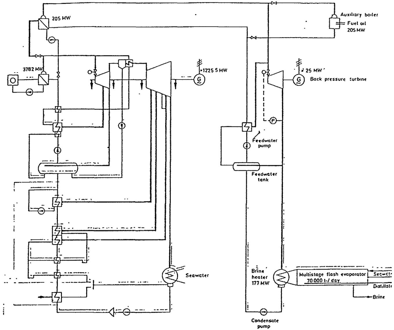
Fig. 1. Combination of a nuclear power plant (PWR) with a desalination plant (MSF) (Option A).
