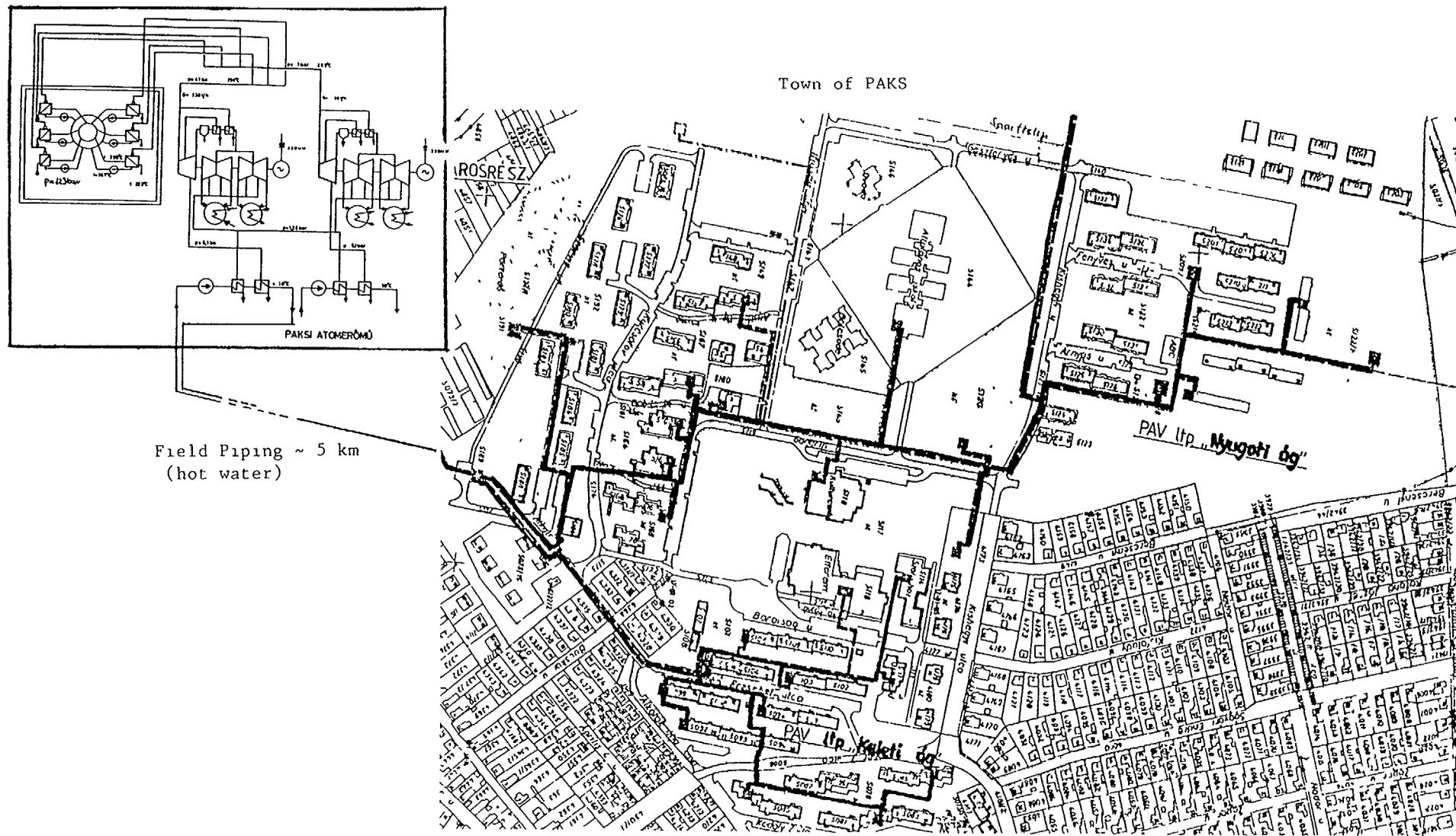
FIG 2 Schematic diagram of a nuclear district heating network in Paks, Hungary
