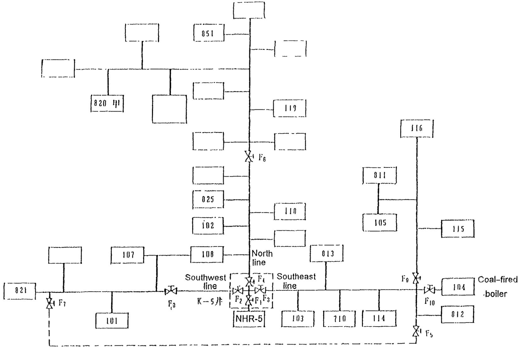
Fig 10 Diagram of heating grid of the NHR-5
