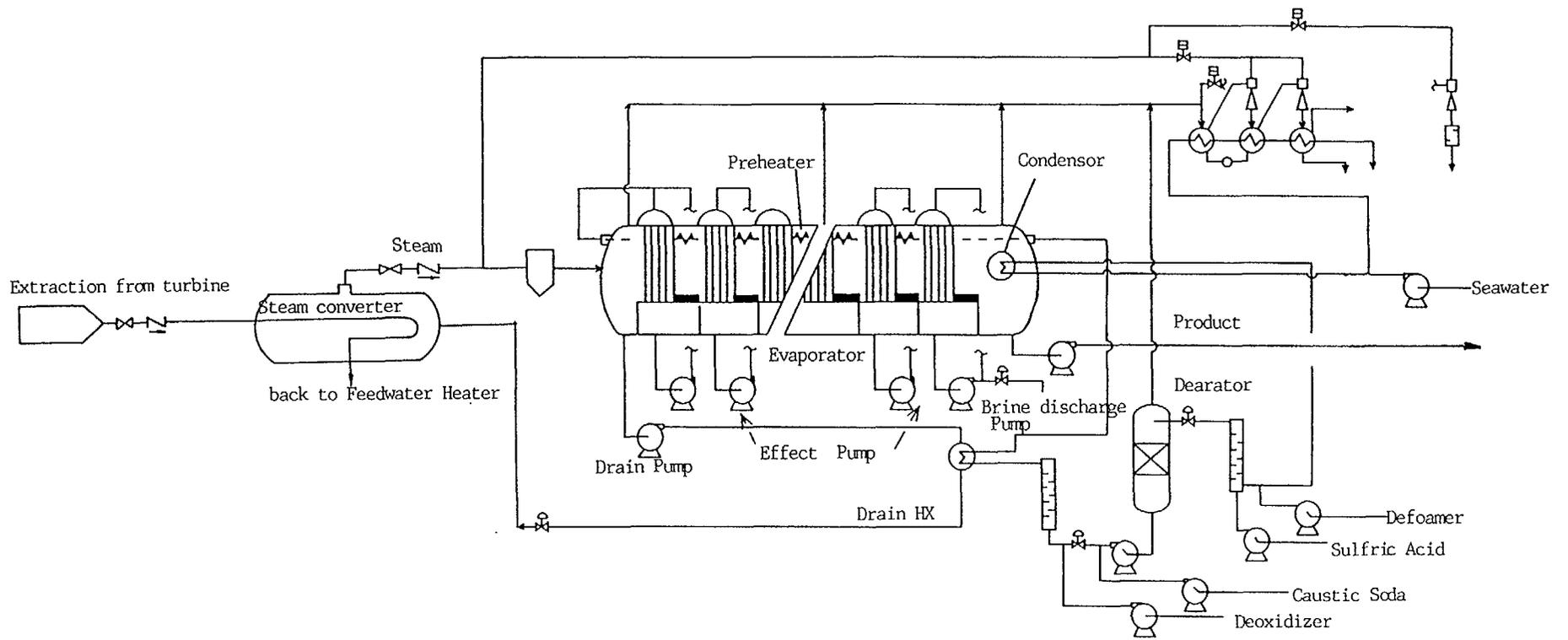
FIG. 8. Schematic illustration of connection between NSSS and desalination facility at Ohi, Japan.
