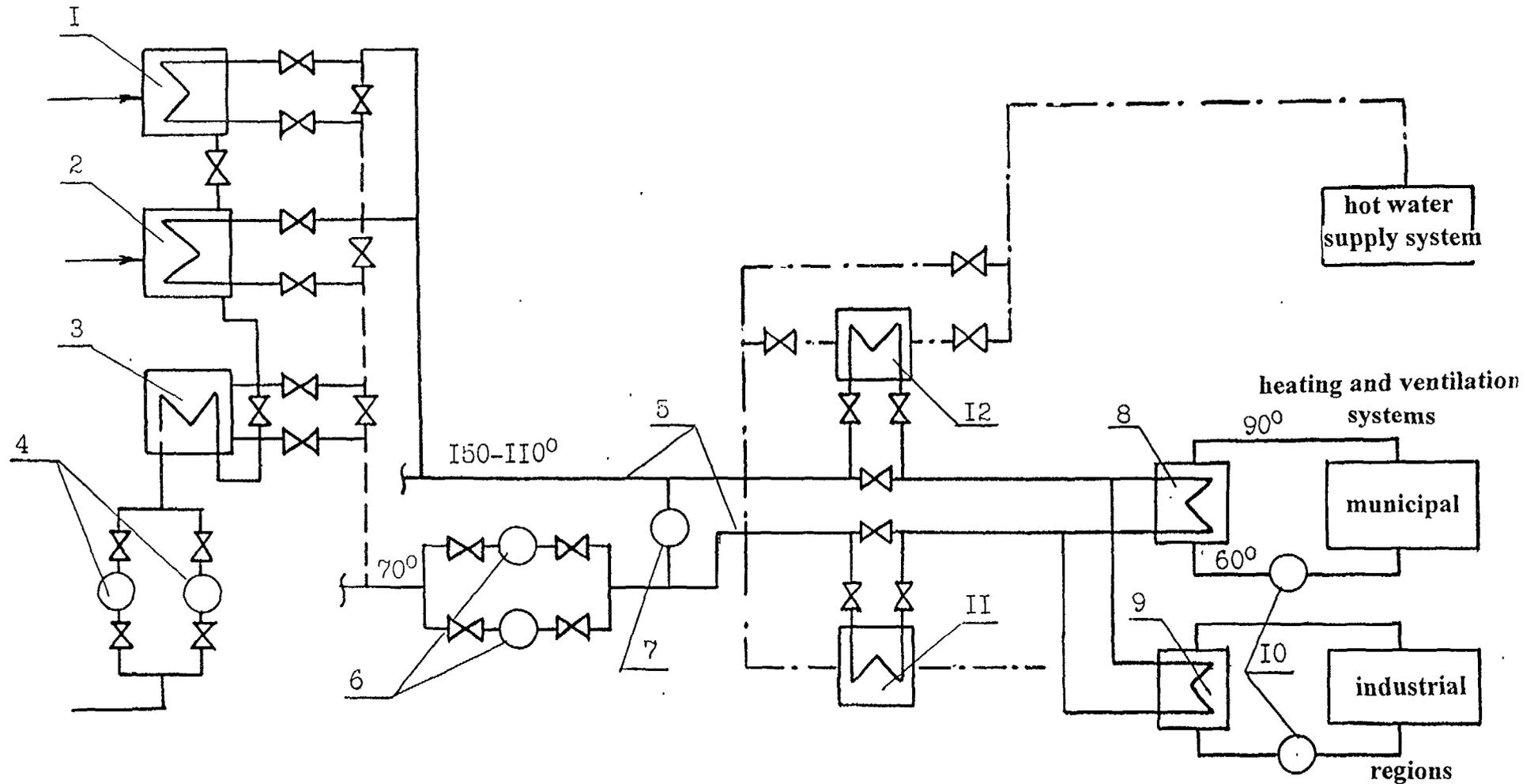
1, 2 - peak and basic heat supply exchangers to heat water in the intermediate loop, 3 - condensate cooler, 4 - condensate pumps, 5 - intermediate loop, 6 - intermediate loop pumps, 7 - pump of the temperature adjustment, 8,9 - heat exchangers of the heating and ventilation systems of municipal and industrial regions, 10 - pumps of the heating systems, 11, 12 - heat exchangers of 1 and 2 levels of the hot water supply system
