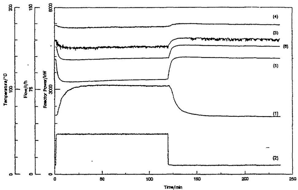
1. Reactor power    2. Flow rate through intermediate heat exchanger
