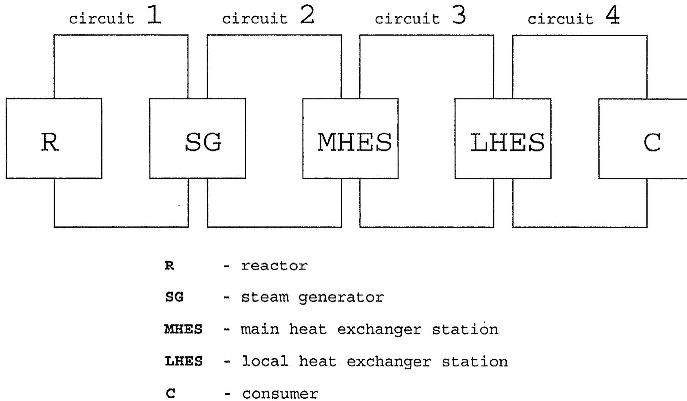
**Fig. 1** Scheme of heat circuits in the NPP and district heating system
