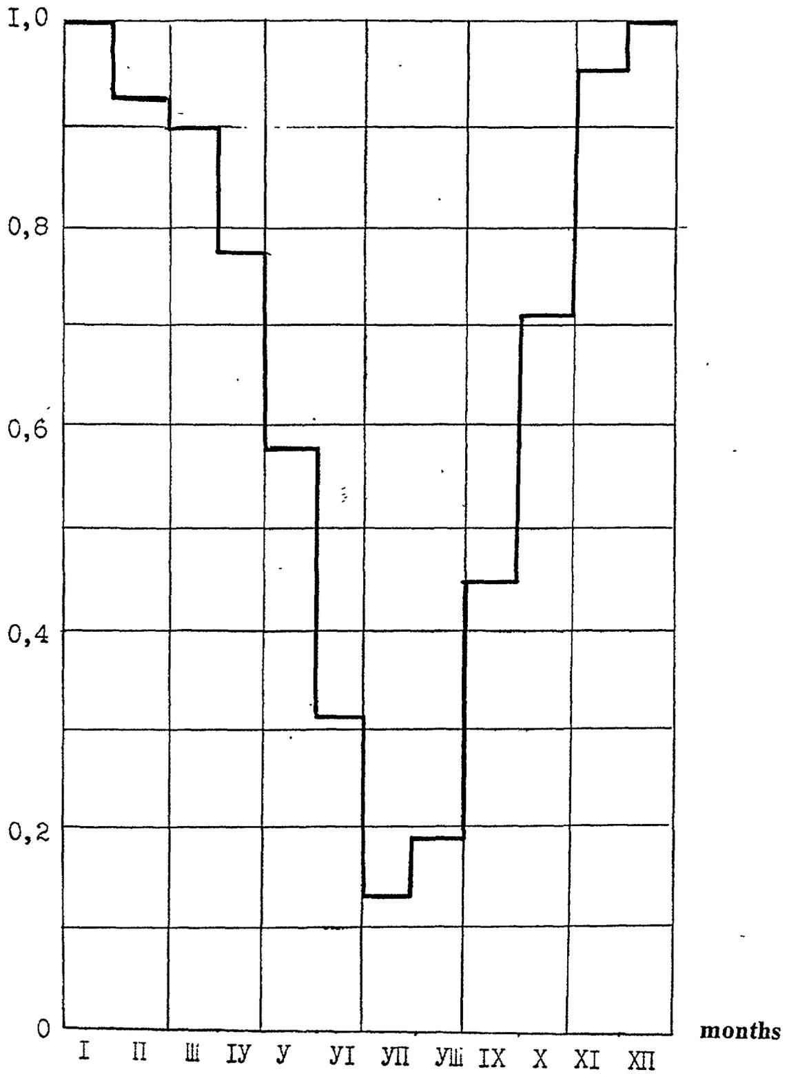
Fig. 4. Annual chart of the heat supply by Bilibino power plant.
