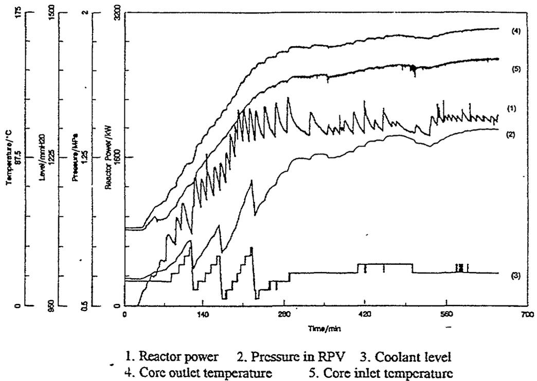
Fig. 8 The start up process of NHR-5
