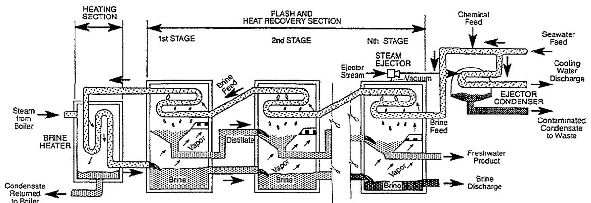
FIG. 3. Diagram of a multi-stage flash (MSF) distillation plant.
