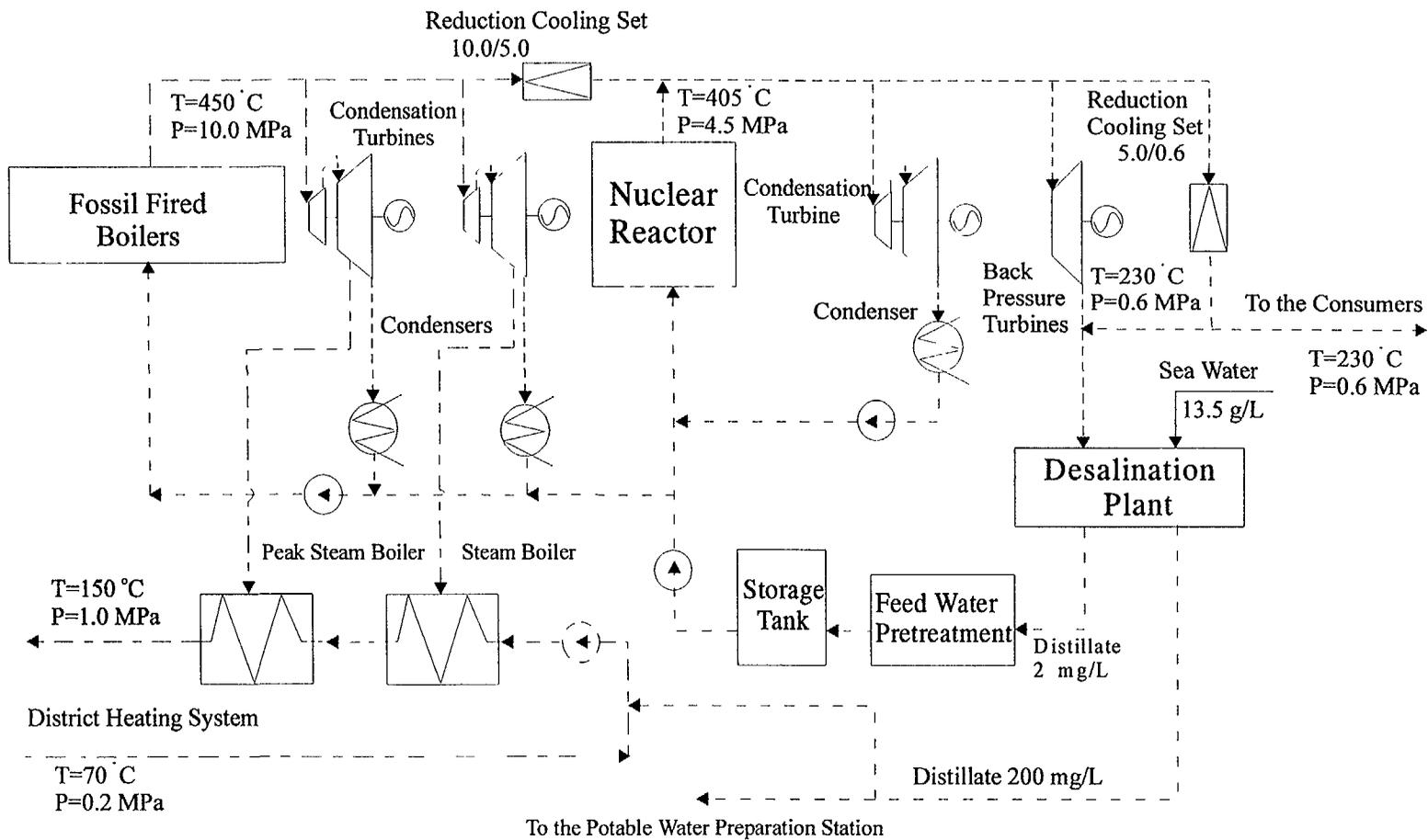
Fig.1. Principle Flow Diagram of Mangyshlak Atomic Energy Complex
