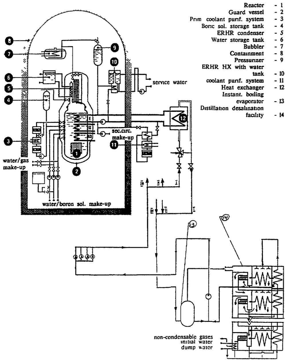
Fig. 1 AST-500 NHR-based Desalination Facility Principal Flow Diagram
