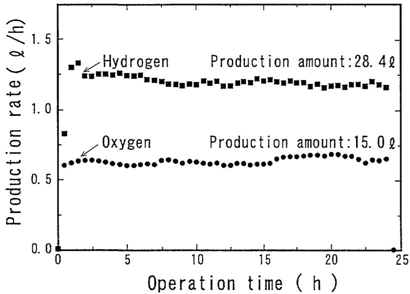
Fig. 6 Results of continuous production of hydrogen and oxygen with laboratory-scale test.
