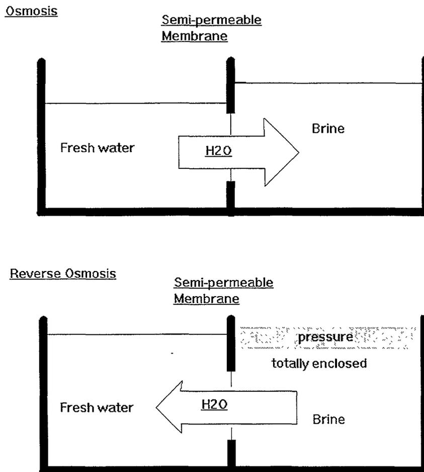
FIG. 5. Principle of reverse osmosis process.
