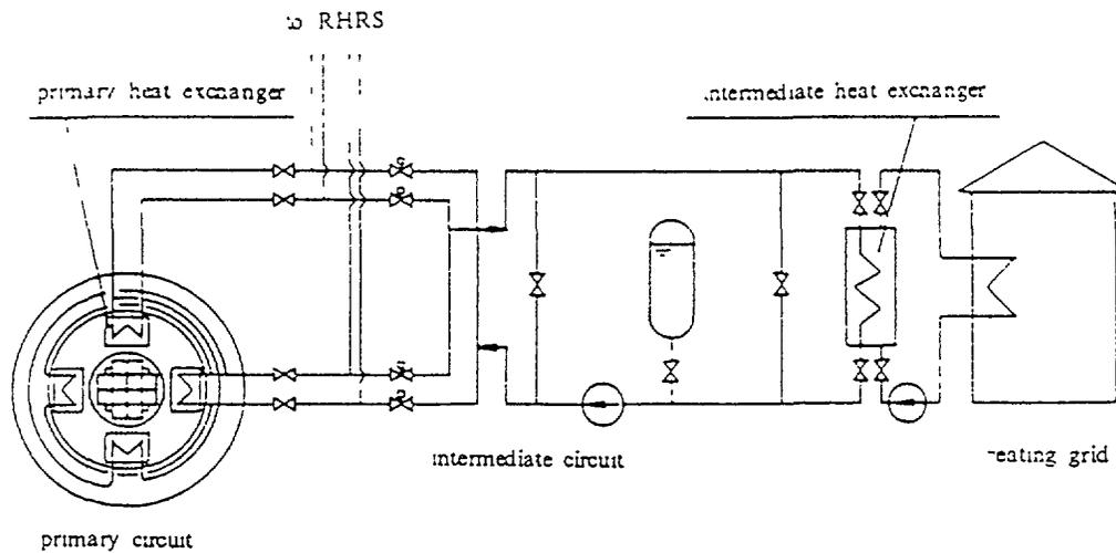
Fig.2 Schematic Diagram of NHR-5 Heat Supply System
