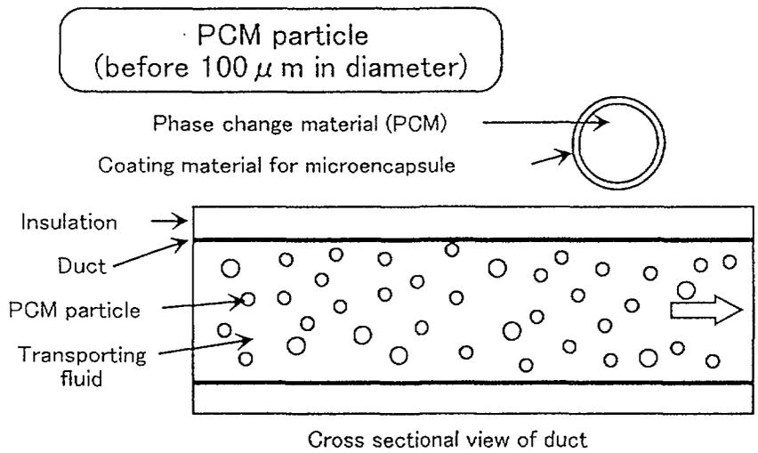
Fig. 7 Concept of slurry heat transport media composed of microencapsulated phase change material.
