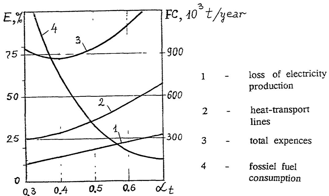
Fig.5 Reduced expenses in NPP-based CHS (E) and fossil fuel consumption(FC) vrs. nuclear heat contribution factor  $\alpha_t$
