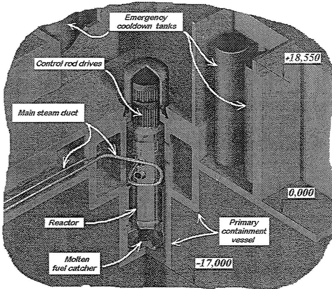
FIG. 1. VK-300 reactor equipment underground layout.
