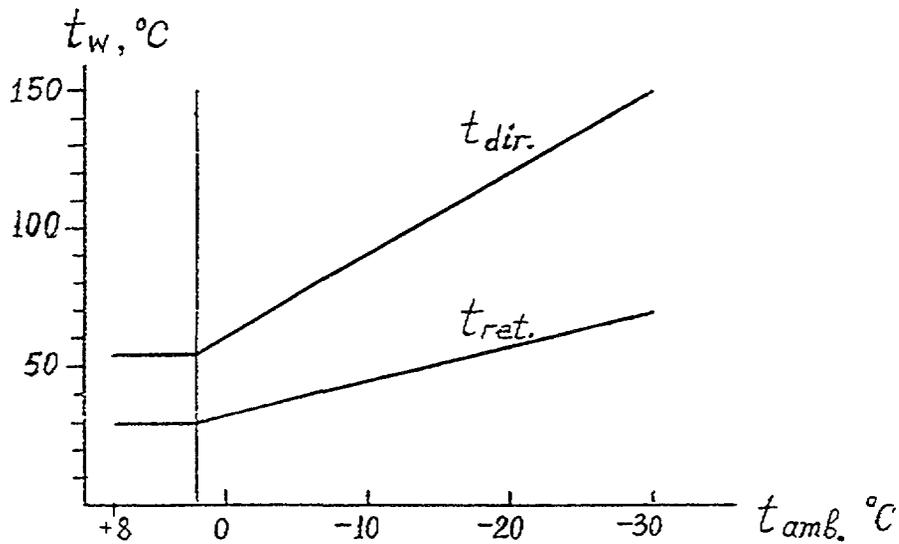
Fig. 2. Heating grid water temperature variation vrs. ambient air temperature
