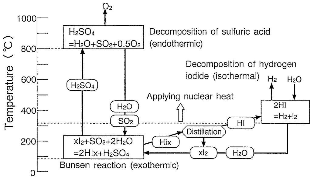
Fig. 5 Reaction scheme of thermochemical IS process.
