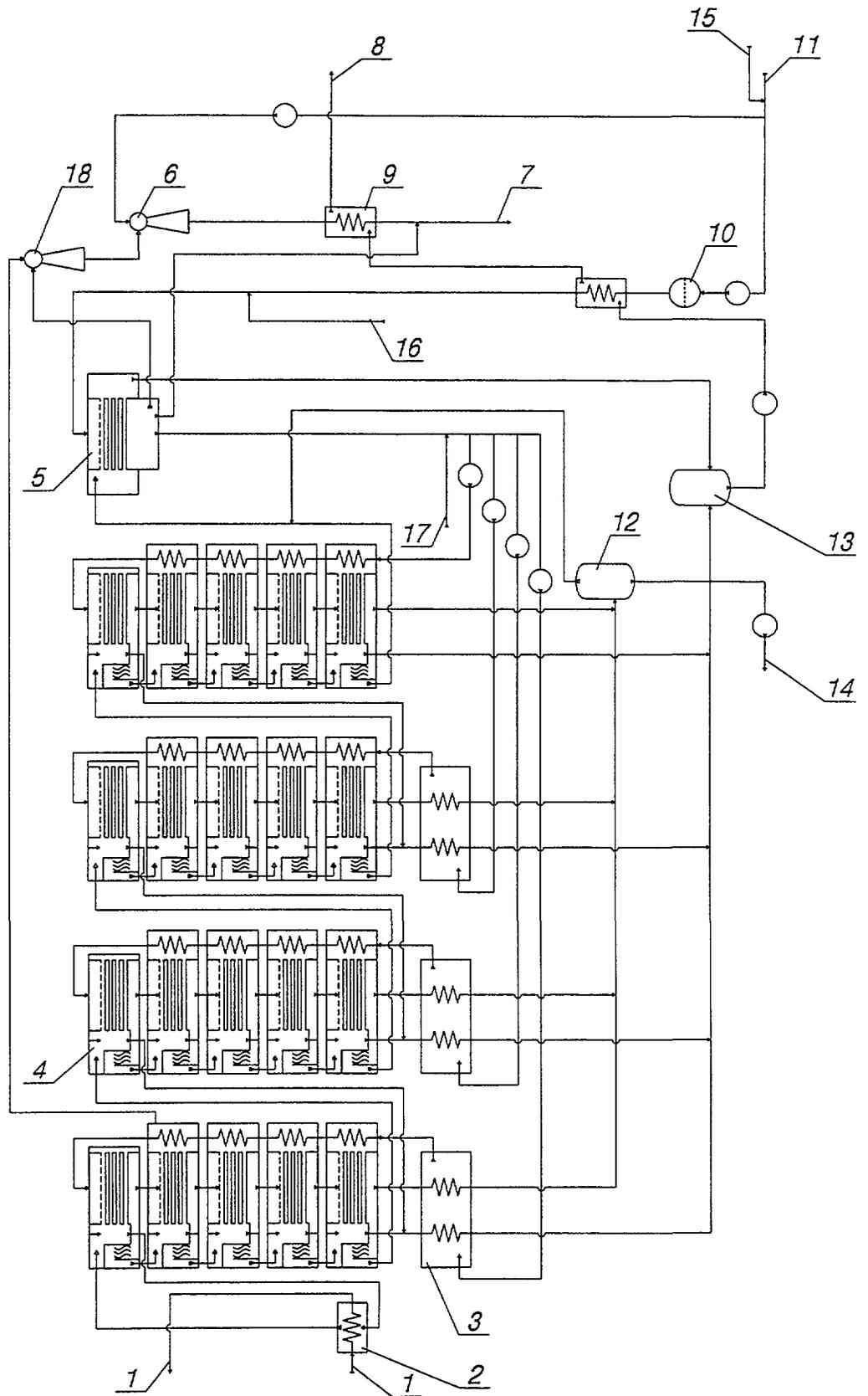
1 - coolant; 2 - steam generator; 3 - preheater; 4 - evaporation stage; 5 - deaerator; 6 - water - jet ejector; 7 - sea water; 8 - distillate to the consumer; 9 - distillate cooler; 10 - filter; 11 - sea water; 12 - sea water concentrate tank; 13 - distillate tank; 14 - sea water with increased salt concentration; 15 - chlorination; 16 - anti - fouling additive inlet; 17 - sodium sulfite inlet; 18 - gas - jet ejector
