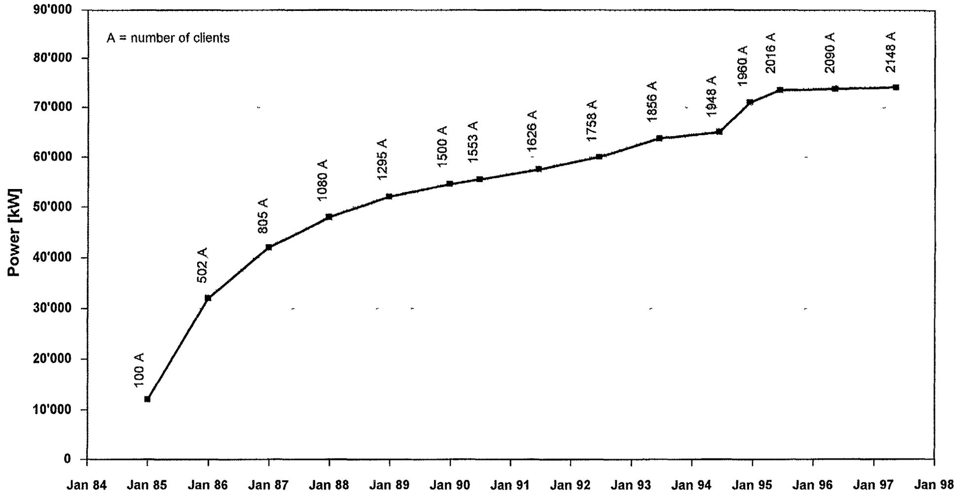
Fig. 7 Housing connections and contracted Heat Load
