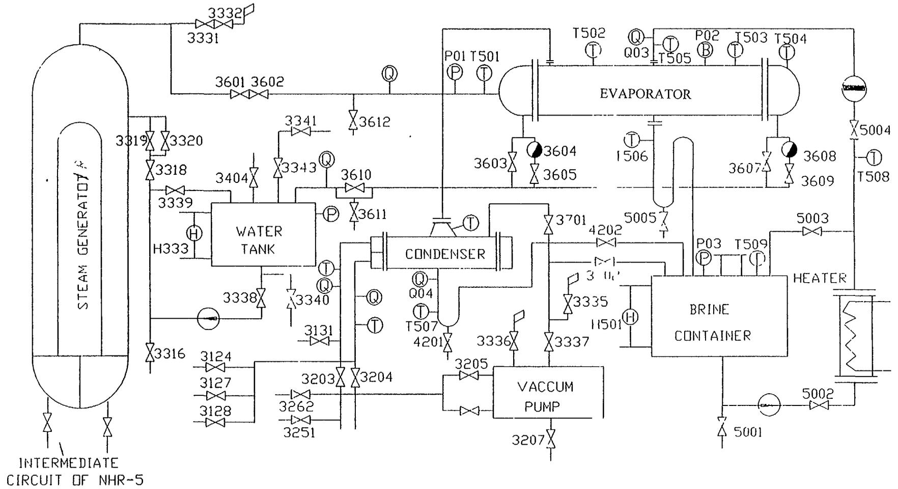
Fig. 12 Flow chart of sea water desalination
