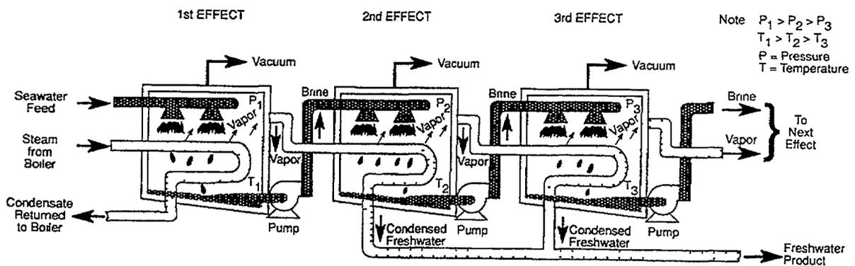
FIG 4 Diagram of a multiple effect distillation (MED) plant
