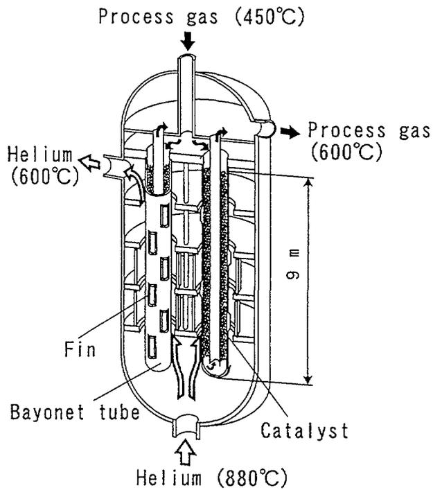
Fig. 2 Schematic view of HTTR steam reformer.
