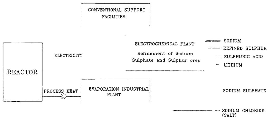
Figure 2. Scheme of the CAREM utilisation in the “Industrial Plant” approach.
