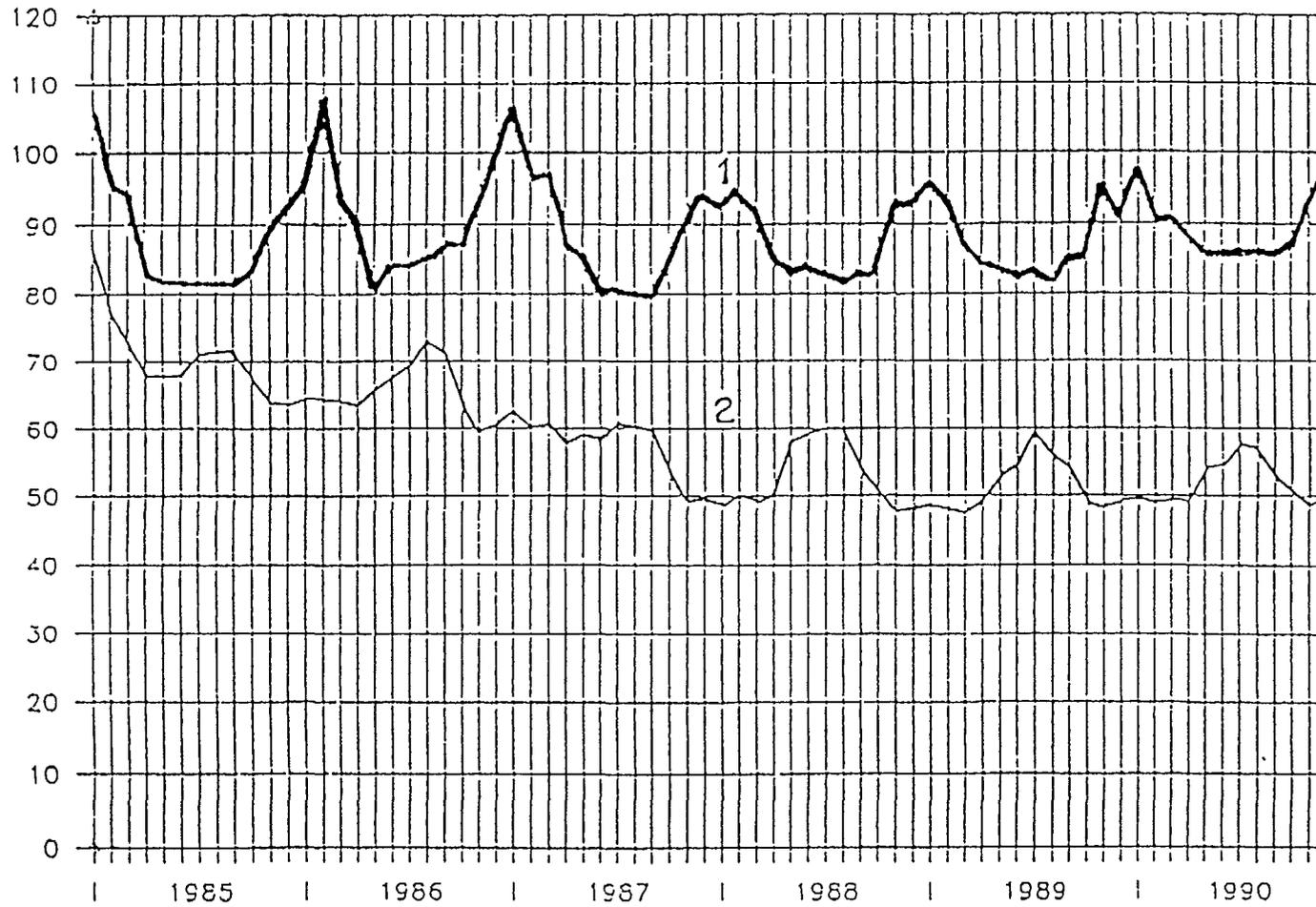
Fig. 11 Decreasing tendency of the return flow (2) temperatures in the Refuna network
