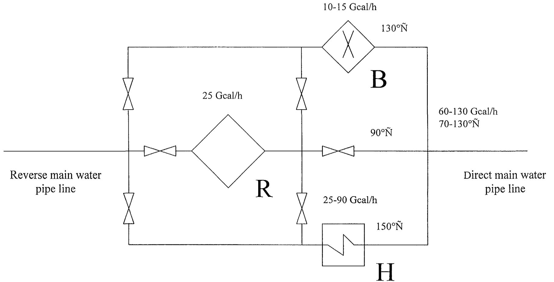
Fig 5 Schematic diagram of coupling of NHP RUTA-30 to IPPE's Heating System
