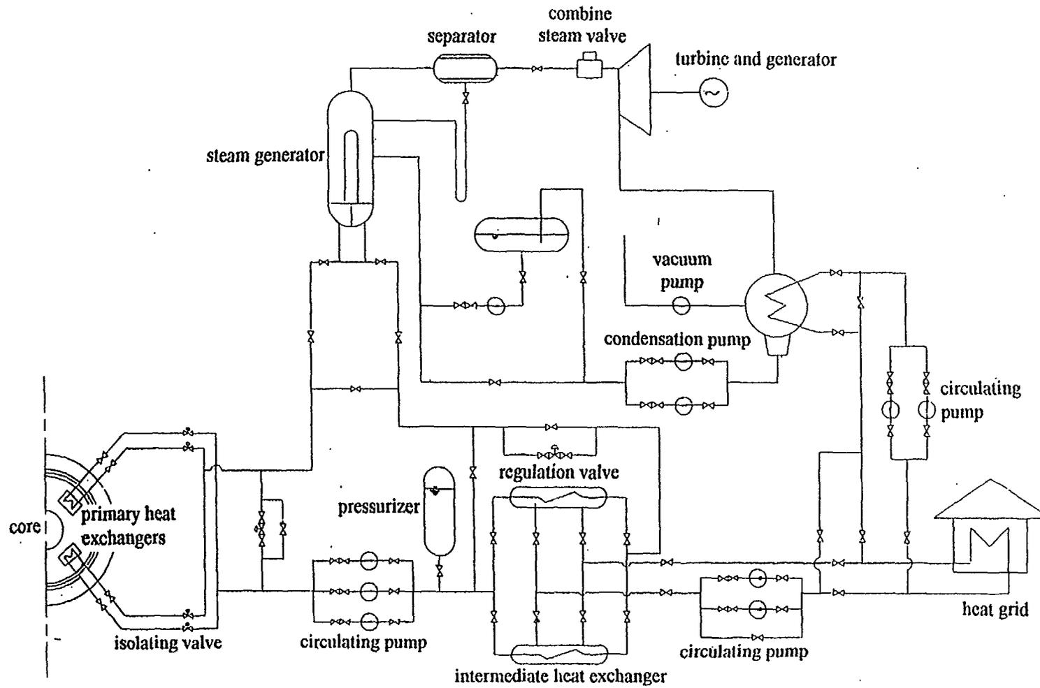
Fig. 9 Steam-power conversion system of NHR-5
