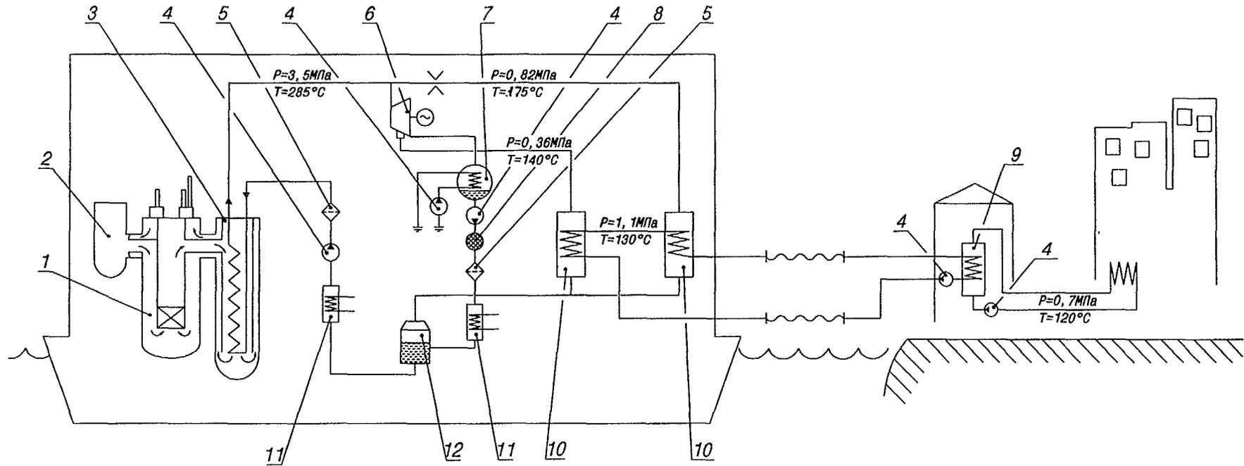
1 - reactor; 2 - reactor coolant pump; 3 - steam generator; 4 - pump; 5 - mechanical filter; 6 - turbo-generator; 7 - condenser; 8 - ion-exchange filter; 9 - district heating system heater; 10 - intermediate circuit heater; 11 - feed water heater; 12 - deaerator
