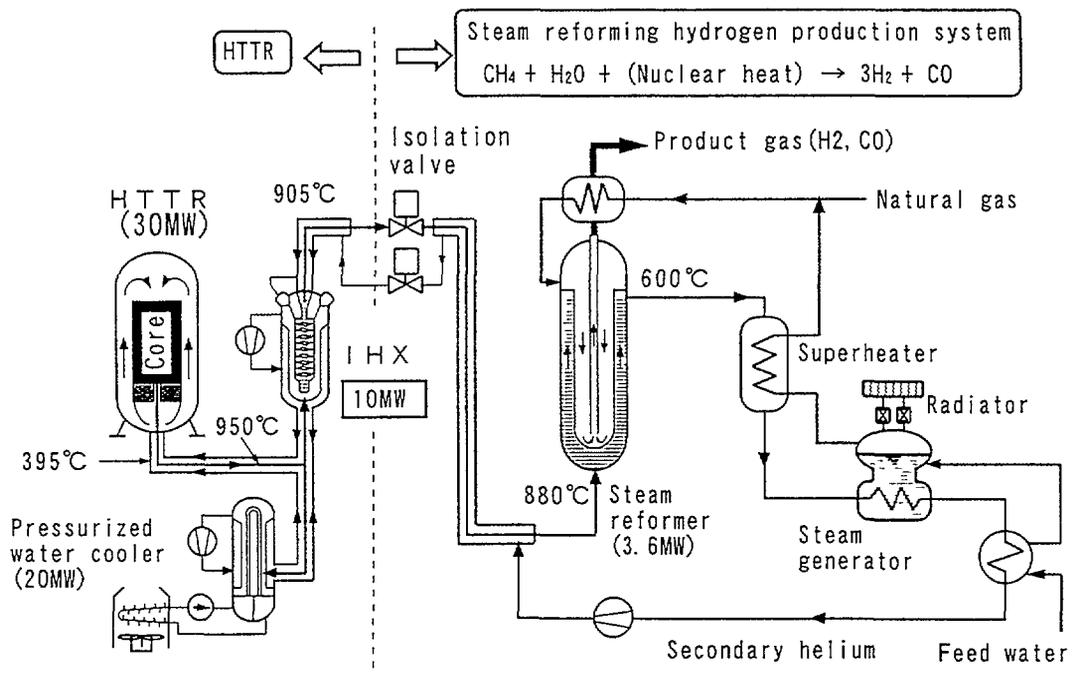
Fig. 1 Flow scheme of the HTTR steam reforming hydrogen production system.
