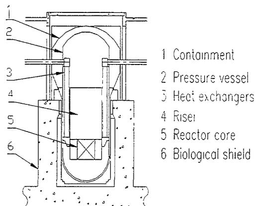
Fig.1 Reactor structure of NHR-200
