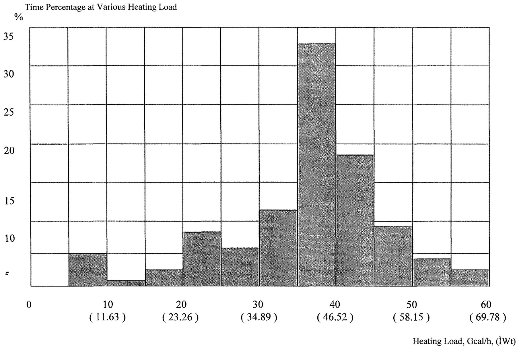
Fig.4 Time Distribution of Heating Load During Heating Period
