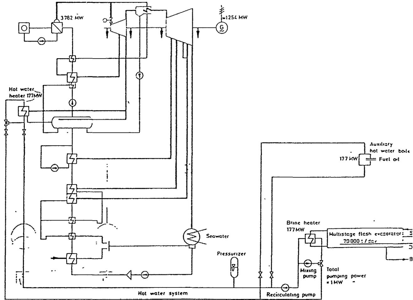
Fig. 3 Combination of a nuclear power plant (PWR) with a desalination plant (MSF) (Option C).
