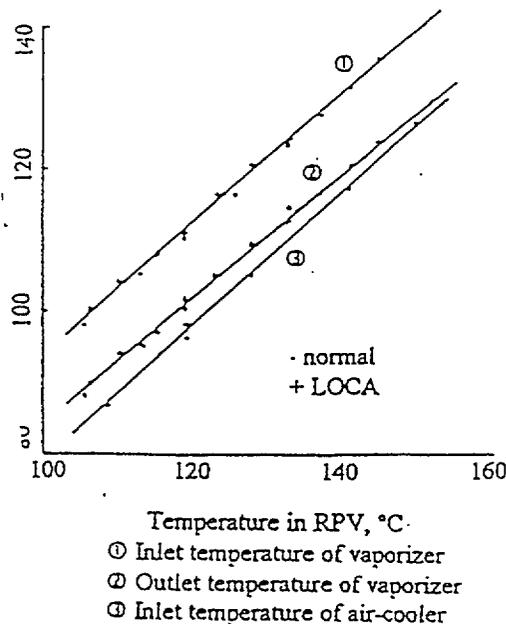
Fig. 7 The comparison of normal and abnormal operation condition of NHR-5
