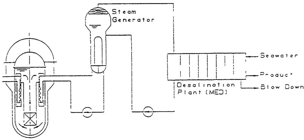
Fig.3 Schematic Diagram of NHR Coupled with H-MED
