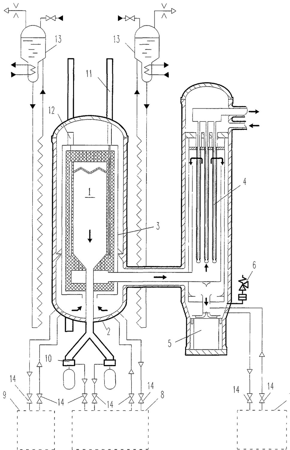
1 - core; 2 - vessel system; 3 - leak tight core shell; 4 - intermediate heat exchanger;
