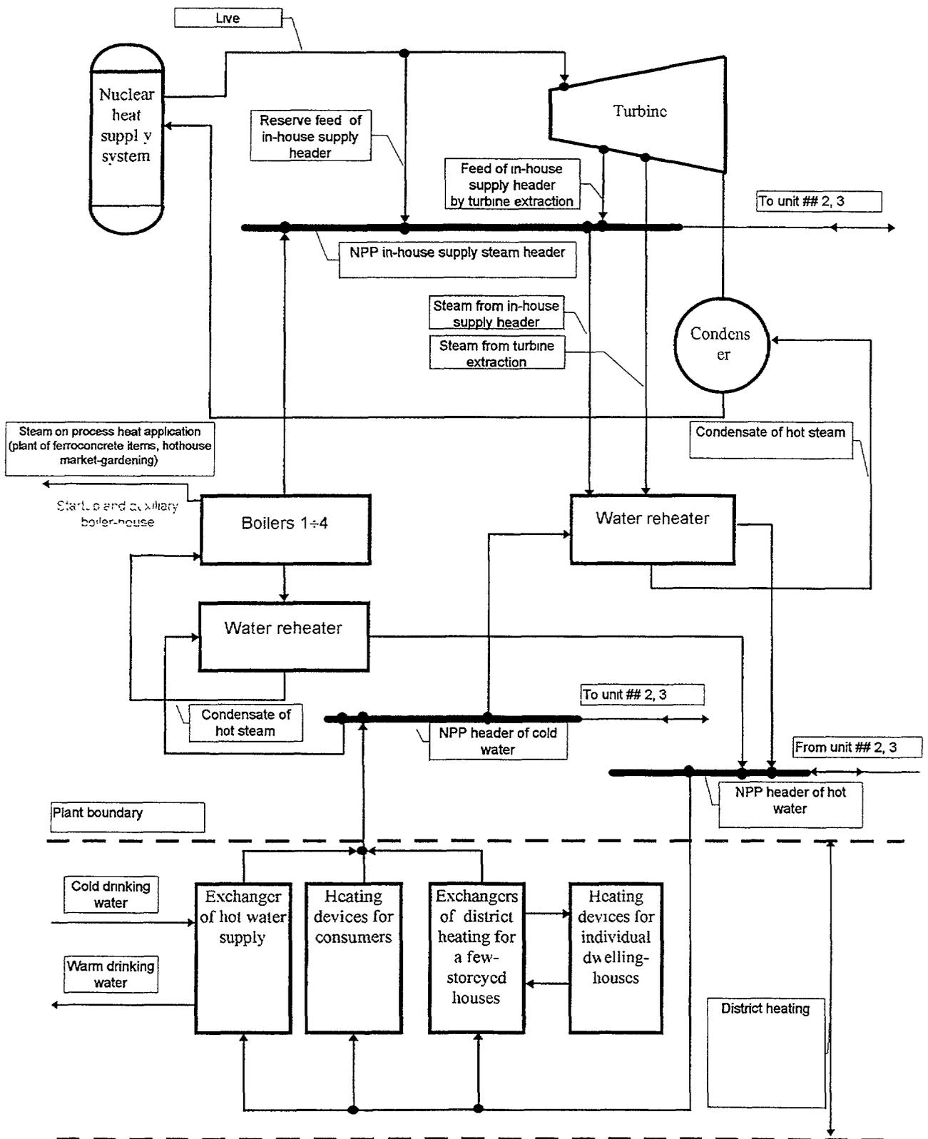
Fig. 6. Scheme of nuclear heat application from the South Ukraine NPP Unit No. 1 (source: V.K. Khokhlov, NNEG "Energoatom", Kiev, Ukraine).
