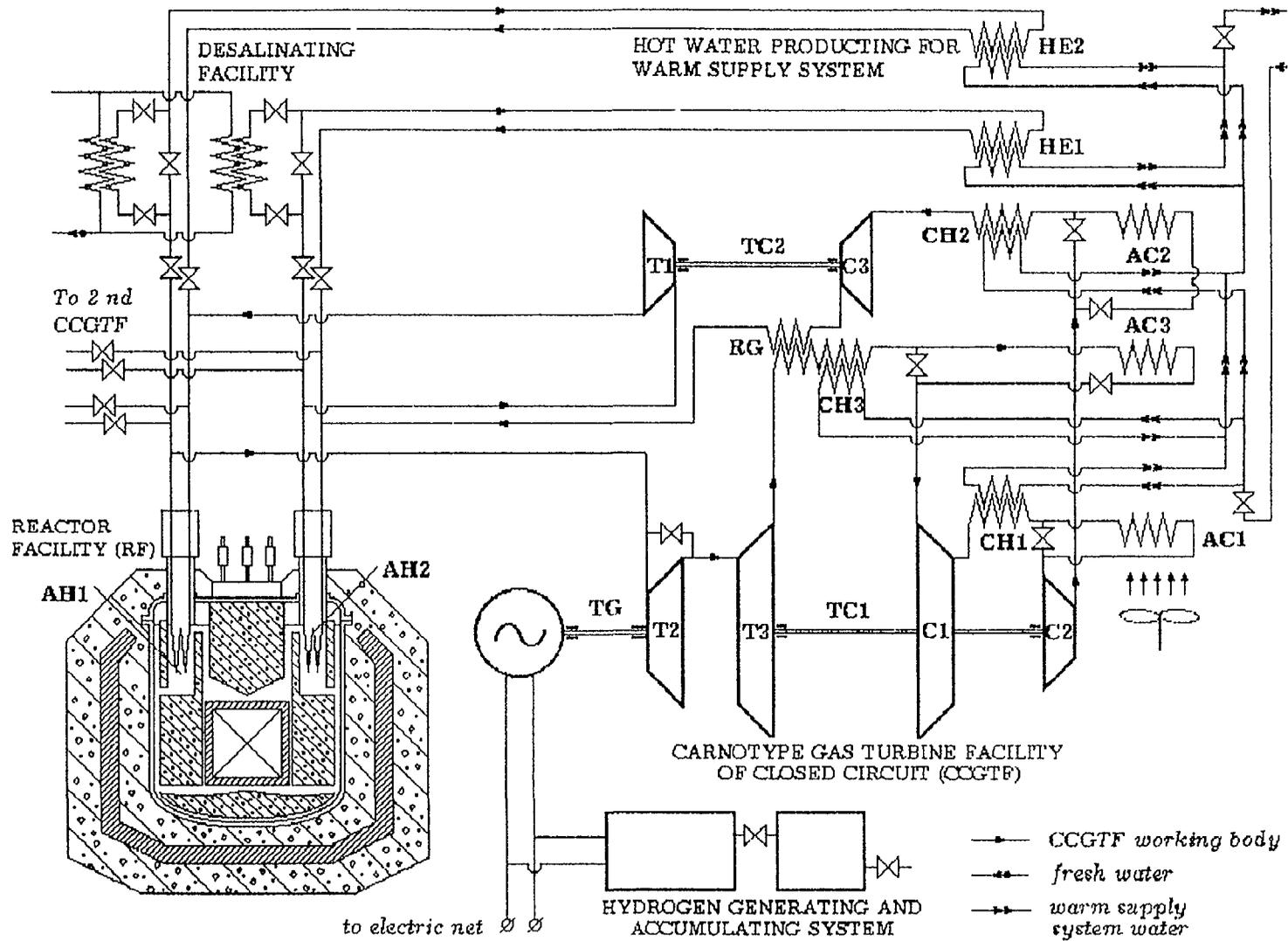
Fig. 1. TNPTP block principle scheme.
