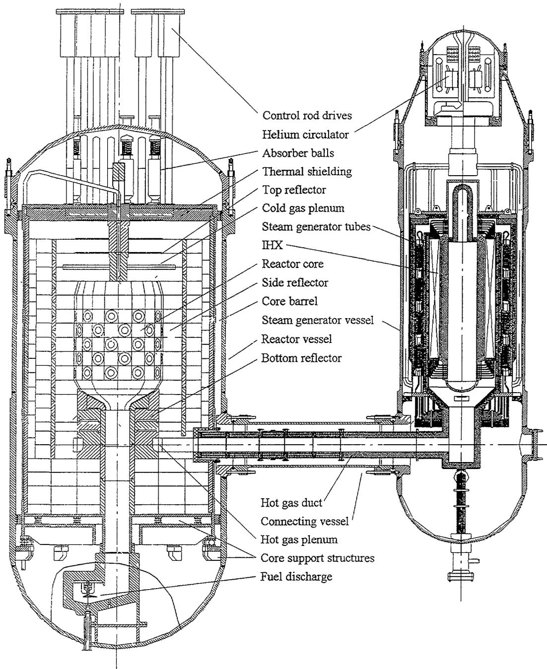
*Fig. 2. The HTR-10 reactor and steam generator.*
