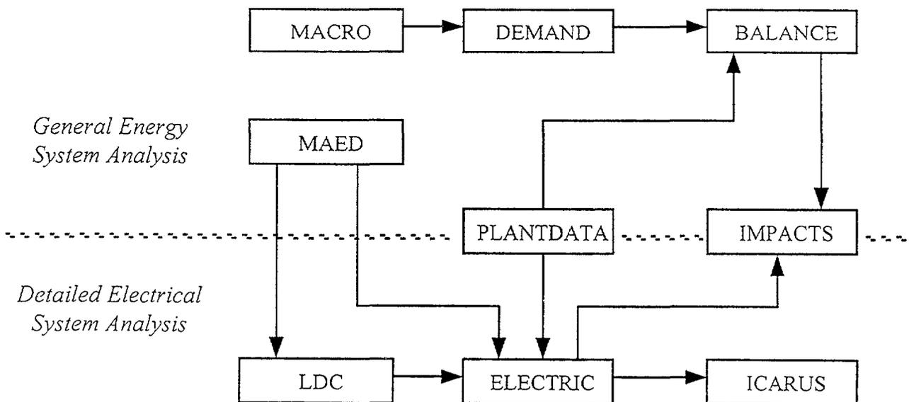
Figure 2. The IAEA ENPEP software package structure
