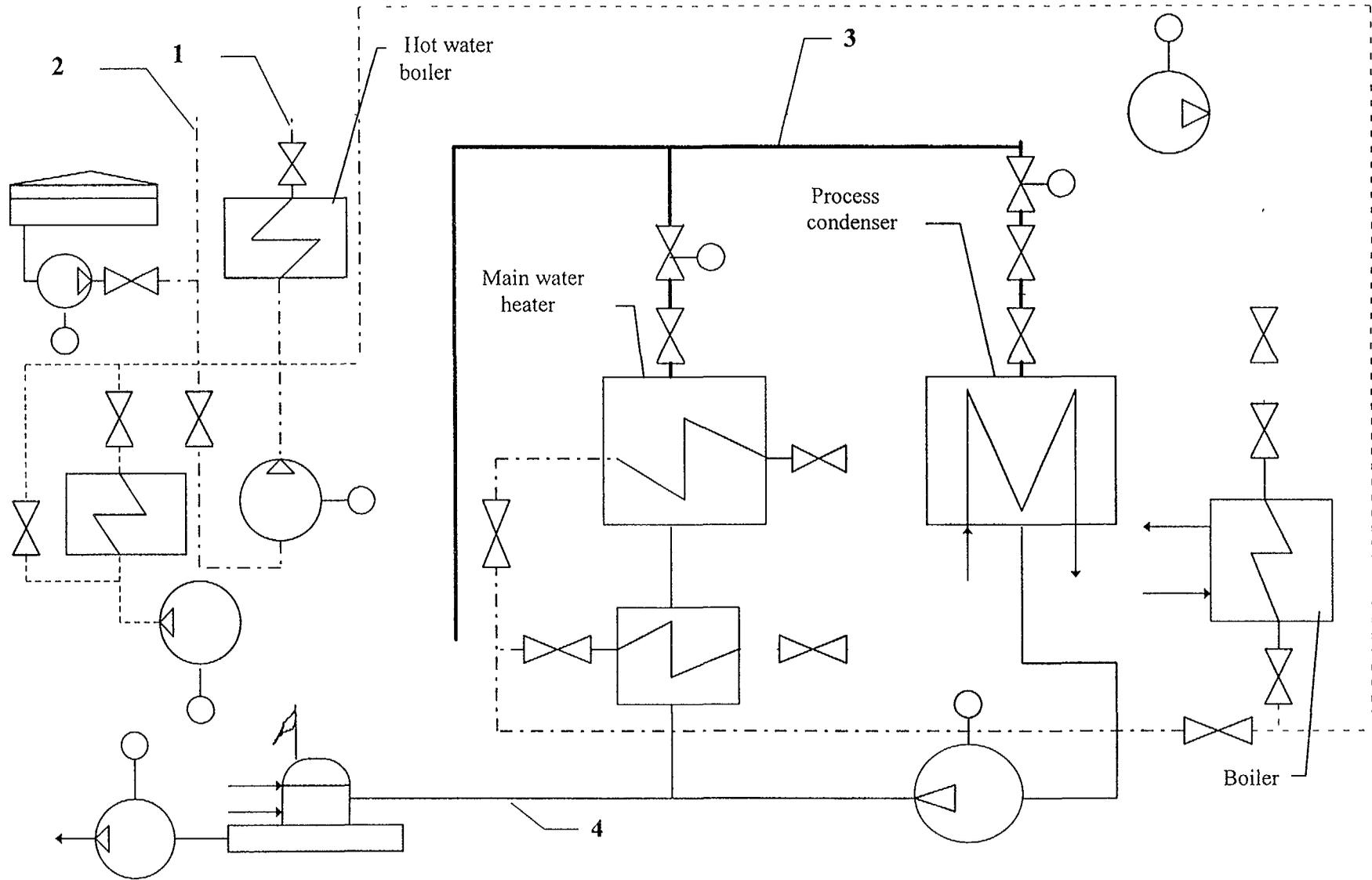
Fig.2 Heat supply system using NPP's steam
