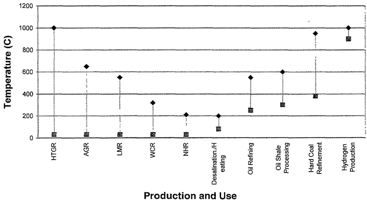
FIG. 1. Temperature ranges in production and use of nuclear heat.
