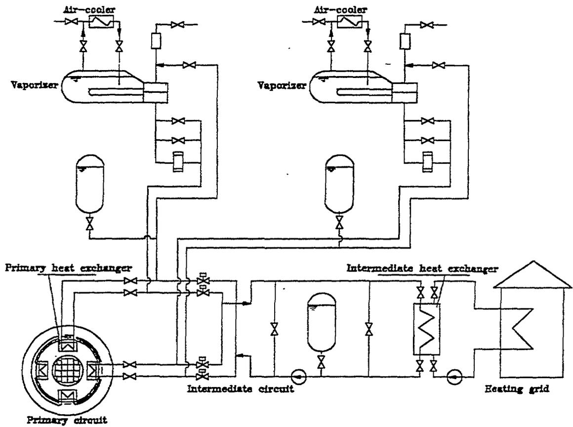
Fig. 3 Main heat transfer system and residual heat removal system
