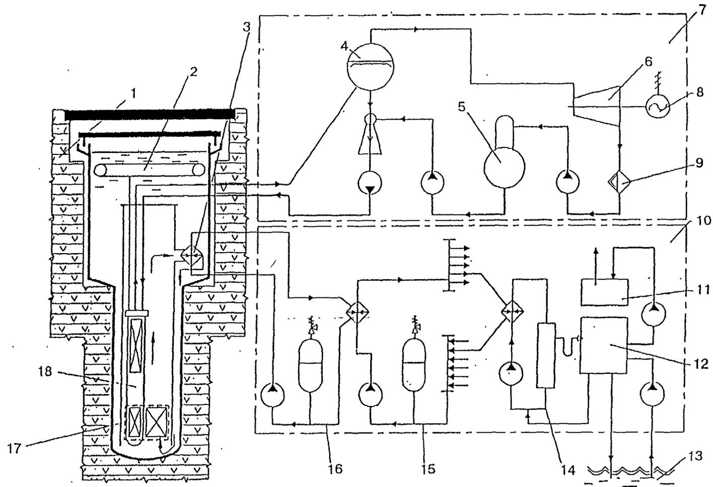
1 - reactor island, 2 - pressurizer, 3 - primary heat exchanger, 4 - separator, 5 - deaerator, 6 - turbine, 7 - turbine island, 8 - generator, 9 - condenser, 10 - desalinating island, 11 - fresh water storage, 12 - water distillation plant, 13 - sea, 14 - vaporization circuit, 15 - third circuit, 16 - secondary circuit, 17 - core, 18 - modular channel
