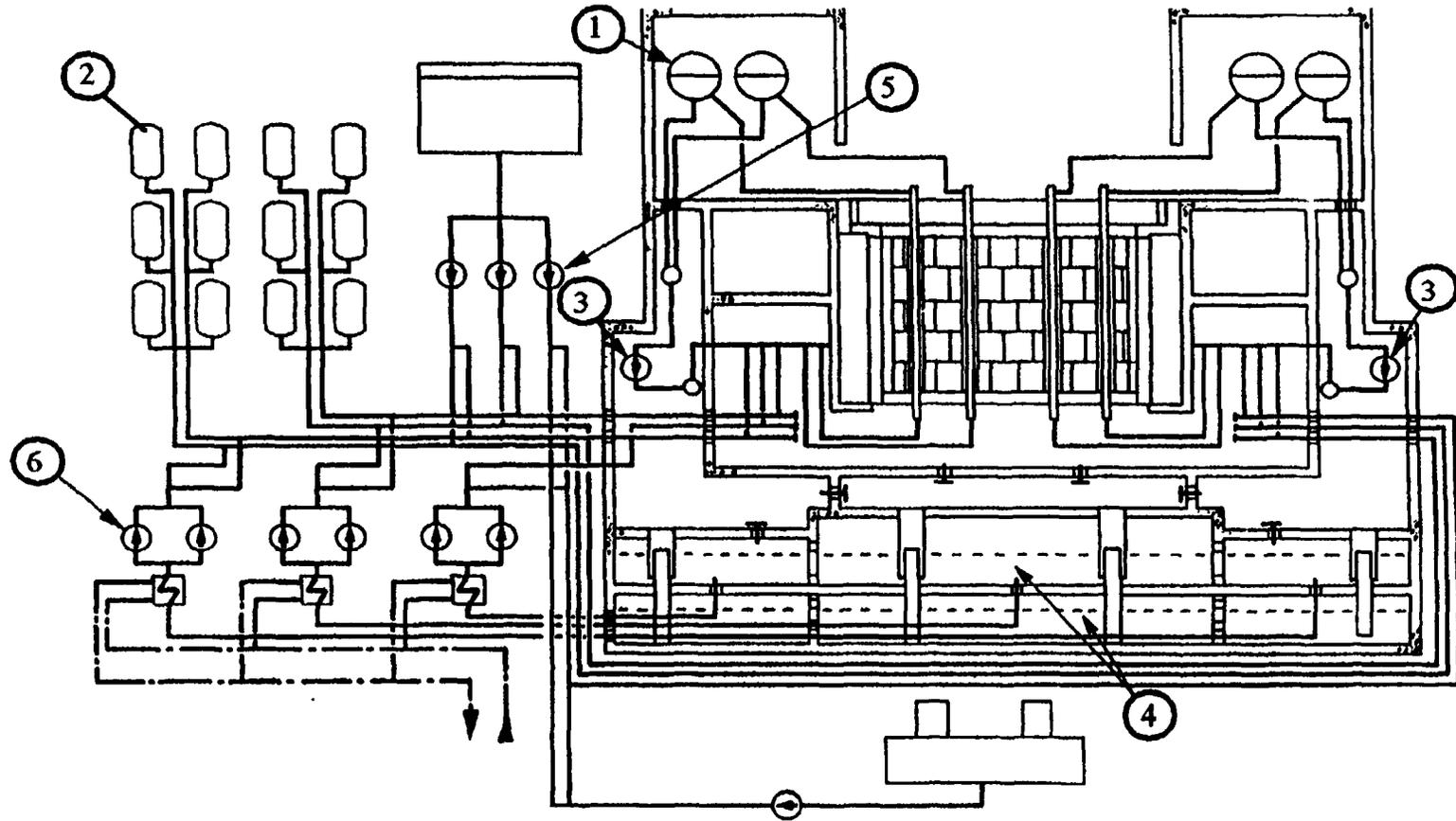
**FIG.3. Accident Localization System**
