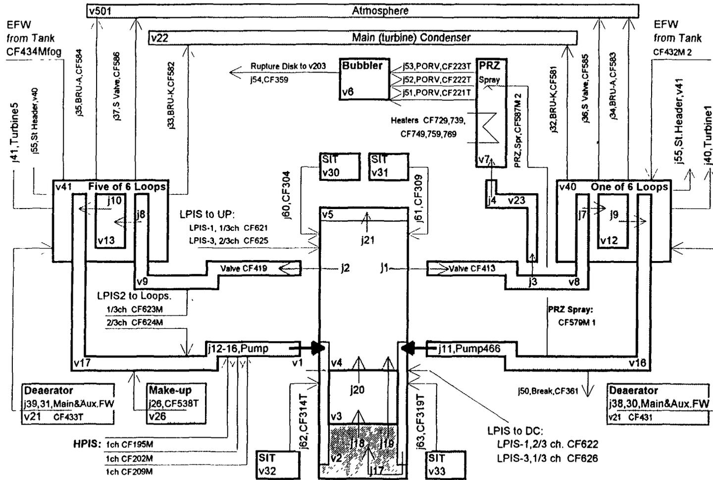
Fig. 1 MELCOR Primary Circuit Nodalization and Flow-Path
