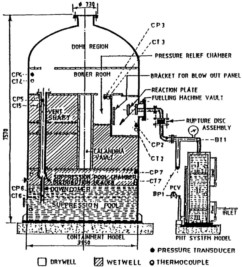
Fig. 2: One-Tenth Scale Vapour Suppression Pool Containment Experimental (VSPE) Facility
