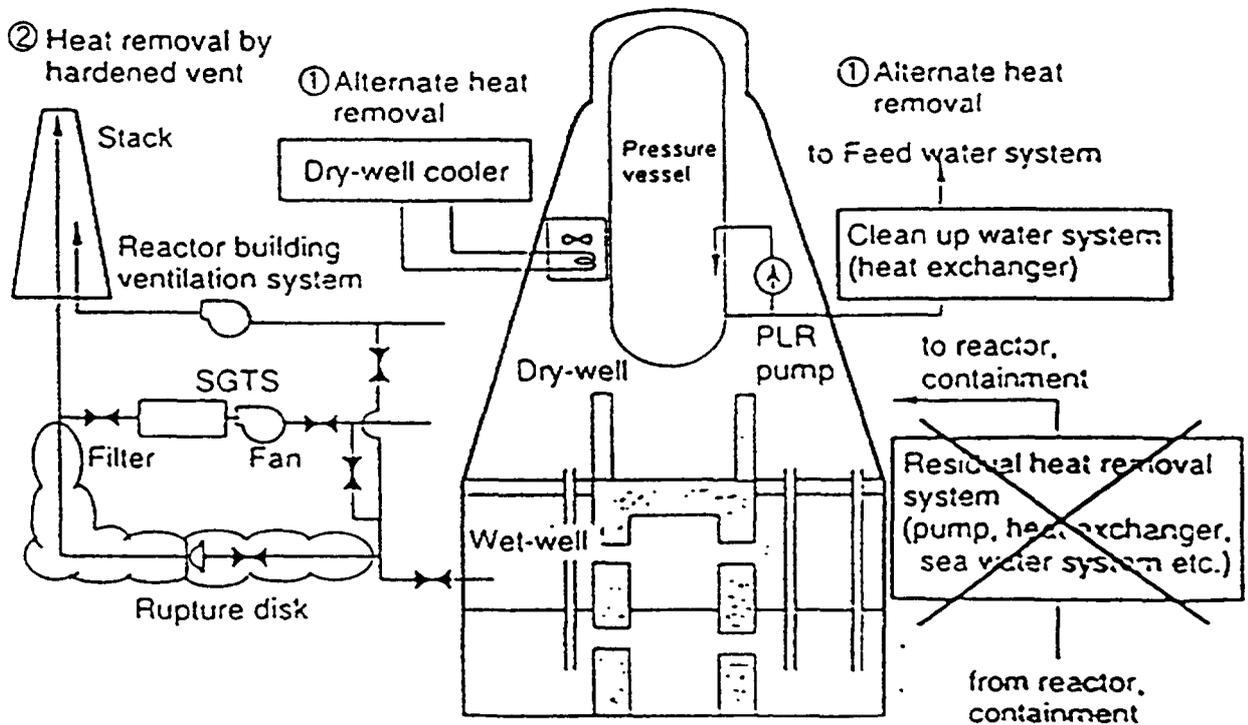
Fig. 4(b) Equipment for containment heat removal [1]
