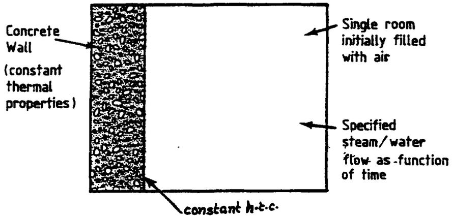
Fig. 6: CSNI Numerical Benchmark Test Model
