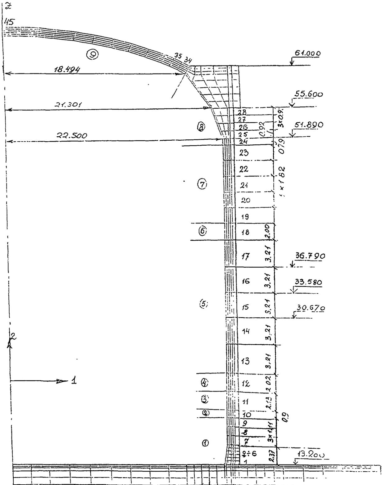
Fig. 4. Finite Element Model of the Containment.
