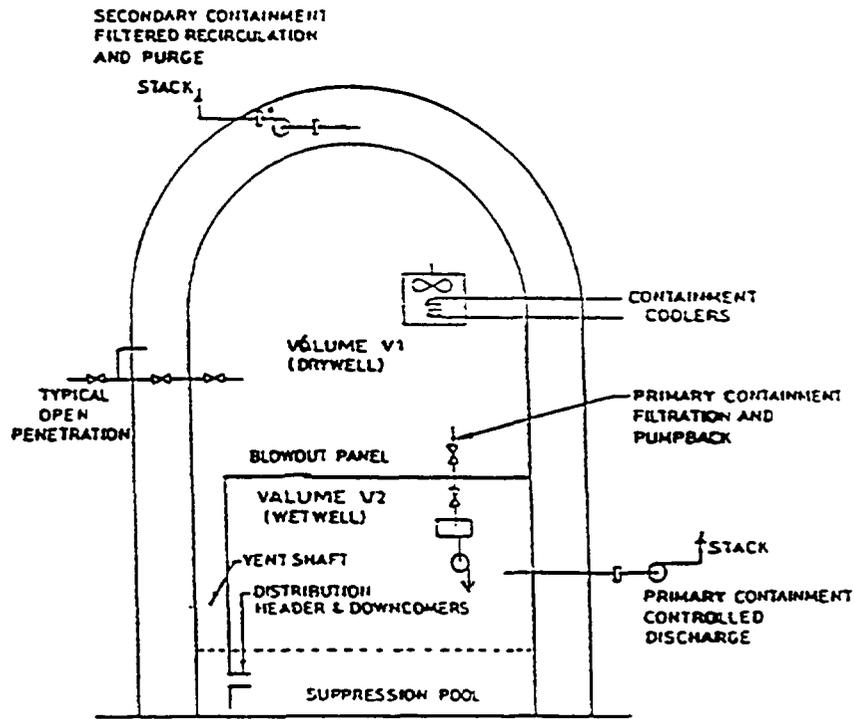
FIG. 2. Schematic of containment and associated safety features in a standardized design.
