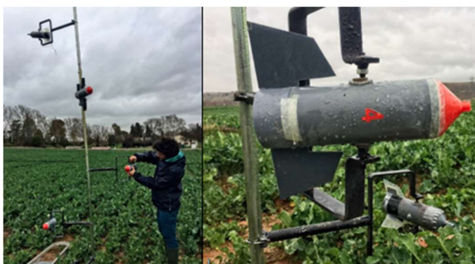
Photo 1. set-ups of the Integrated Horizontal Flux Method (IHF) for on-site ammonia measurements. (photo credit: A. Sanz Cobeña (UPM)).
