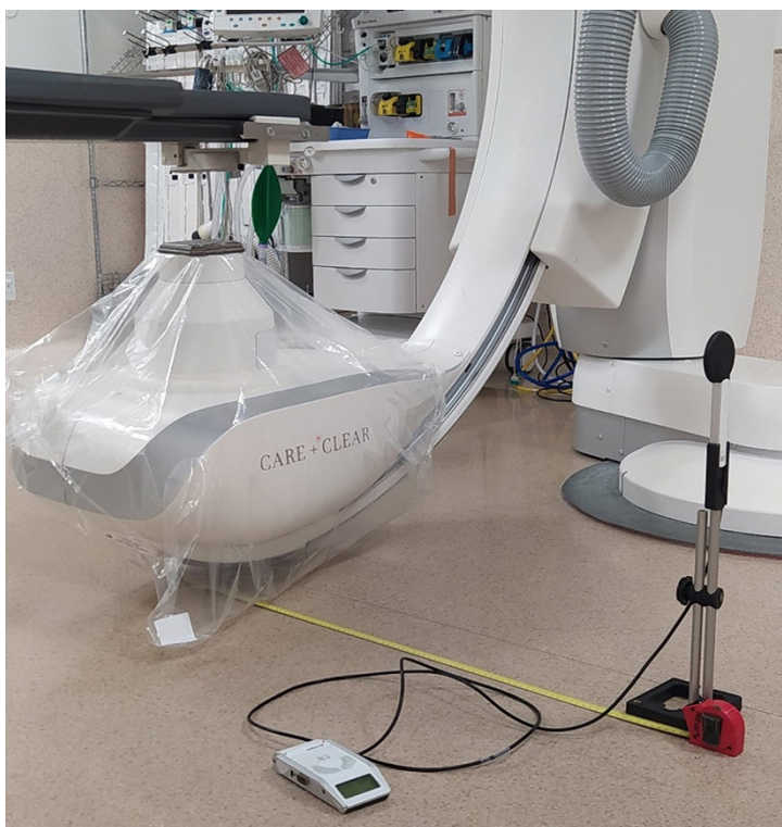
FIG. 34. Leakage radiation measurement set-up.
