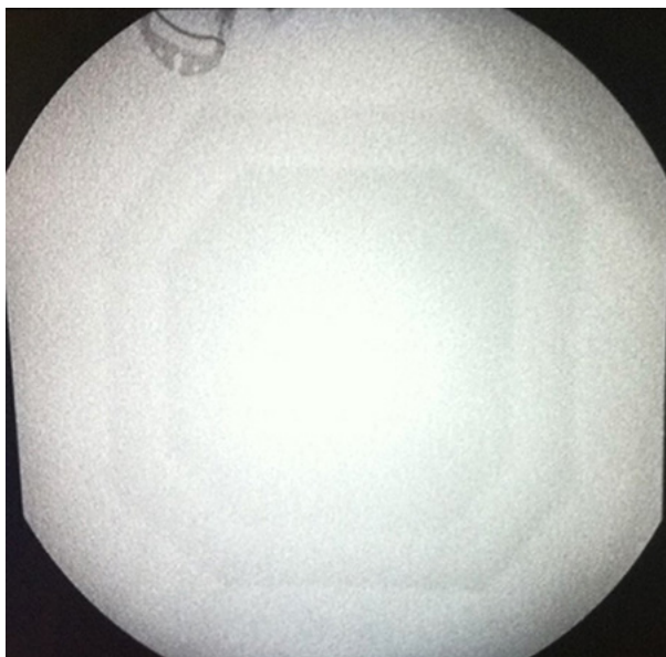
FIG. 25. Example of an artefact: smaller FOVs are visible on the image.
