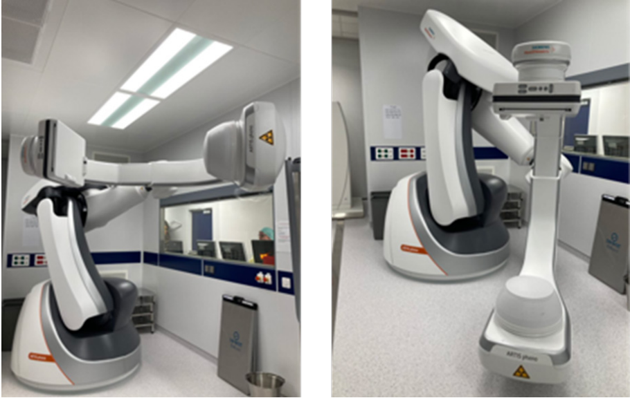
FIG. 13. Examples of gantry movements of a robotic system.
