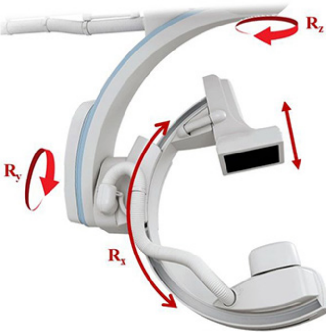
FIG. 11. Geometry of a C-arm gantry and its degree of freedom. R_x corresponds to the angulation of the C-arm and R_y to the rotation; R_z is the L-arm rotation as mentioned in Ref. [10].
