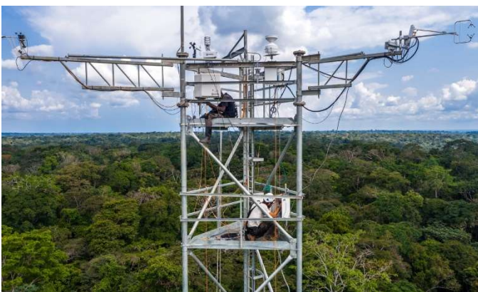
Figure 2. Cosmic ray neutron sensor with two moderated and two bare sensors. (photo credit: Daelman, R., 2023)
