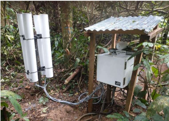
Figure 1. Cosmic ray neutron sensor CRS 2000/B (Hydroinnova LLC) (photo credit: Daelman, R., 2023)
