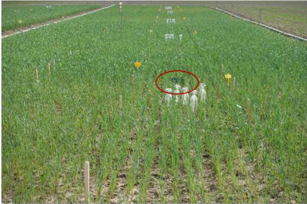
Figure 1. Nitrous oxide chambers in the field. (photo credit: Mirkhani, R., 2022)
