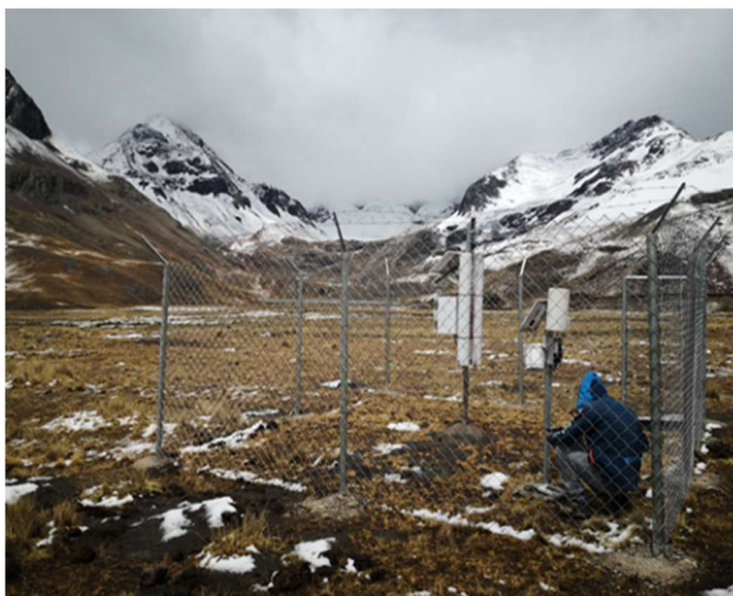
Figure 1. Cosmic Ray Neutron Sensor and low-cost weather station installed in the Huayna Potosi watershed in Bolivia (left) (photo credit: Ramírez, E., 2023), soil moisture data from CRNS (right).
