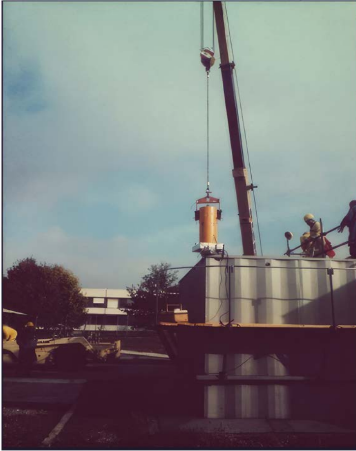
FIG. IV-4. Outdoor handling of SNF: shielded on-site transport unit attached to a crane, with grey open SNF loading basin containing the transport and storage cask (courtesy of U. Lichnovsky, FRM II, Germany).
