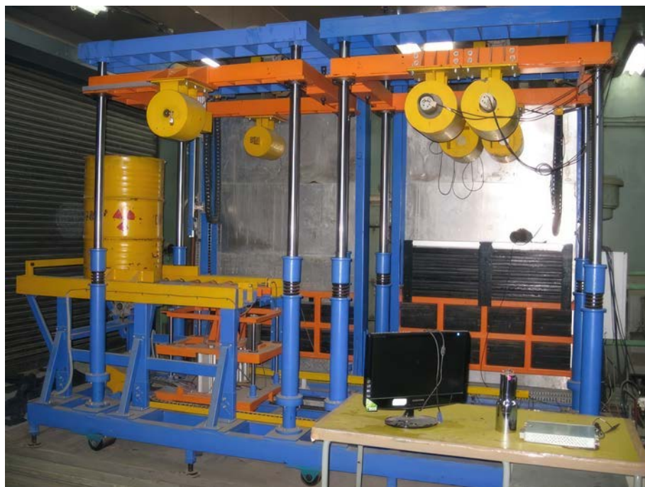
FIG. I-7. Solid radioactive waste drum scanning system (courtesy of R. Ranjan, BARC, India).
