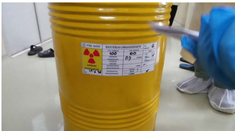
FIG. 15. Example of labelled drum containing ICSDs (courtesy of the National Nuclear Energy Agency, Indonesia).
