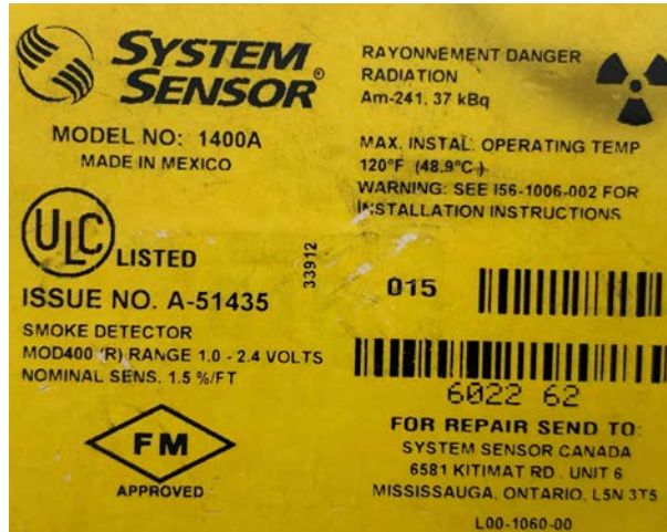
FIG. 3. ICSD Model System Sensor 1400A yellow label with the trefoil symbol and the words 'radioactive material Am-241'.
