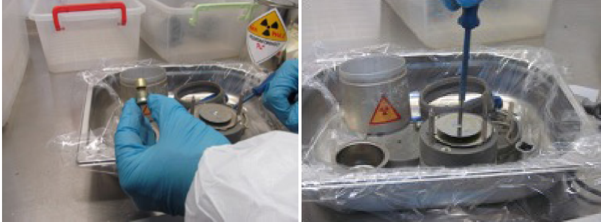
FIG. 13. Example small tray work area design to minimize the loss of DSRS during dismantling.
