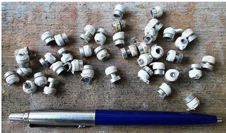
FIG. 16. Tens of ^{241}\text{Am} sources within their holders removed from ICSDs.
