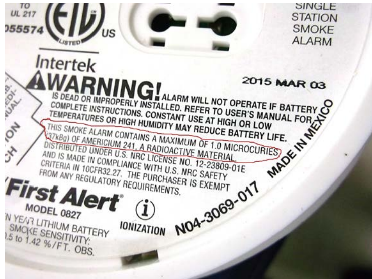
FIG. 5. ICSD Model First Alert 0827 with white label showing a circled 'i' ionization symbol and the words 'americium 241, a radioactive material'.
