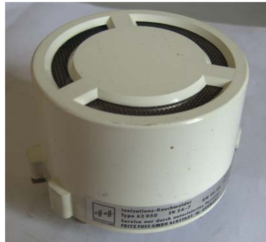
(b) One model that uses a ^{226}\text{Ra} or ^{241}\text{Am} SRS.
