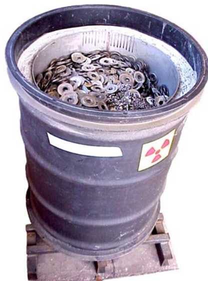
FIG. 28. A 440 L drum filled with ^{241}\text{Am} sources recovered from ICSDs [7].
