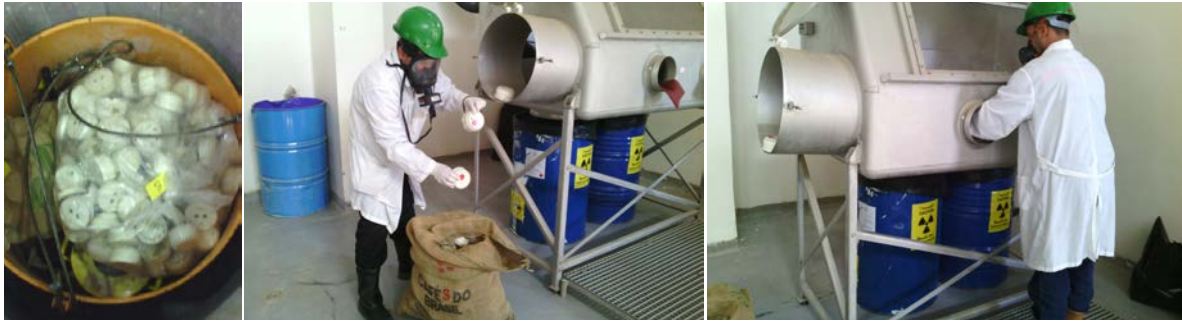
FIG. XVIII-1. Collecting disused ICSDs and dismantling.
