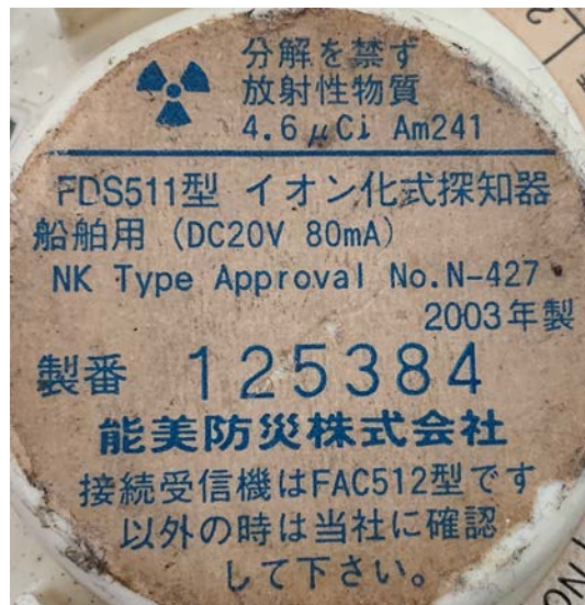
FIG. 6. ICSD model FDS511 with white label showing the trefoil symbol and indicating the presence of 'radioactive substances... Am241'.
