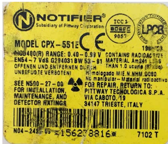
FIG. 2. ICSD Model Notifier CPX-551E yellow label with trefoil symbol and the words ‘radioactive material Am241’.
