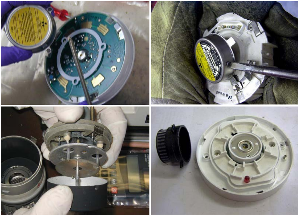
FIG. 19. Opening the ionization chamber.
