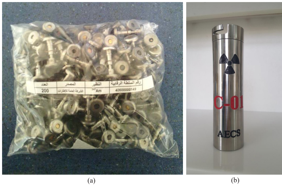
FIG. XVIII-2. (a) Disused 241 Am sources recovered from ICSDs and (b) Syrian stainless steel capsule for DSRS conditioning.
