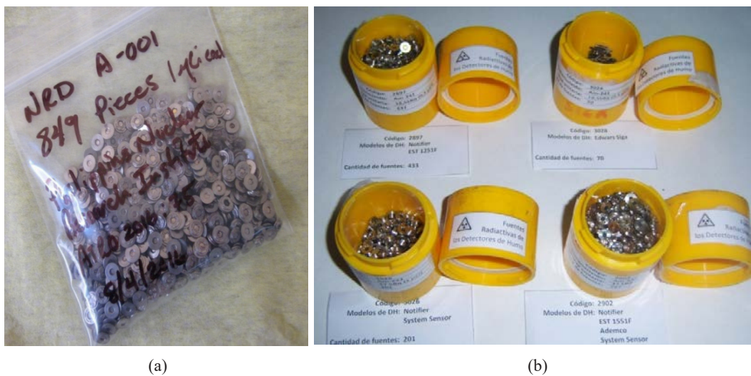
FIG. 21. Examples of collection containers for DSRS: (a) appropriate collection containers after a dismantling campaign (courtesy of the Centre for Radiation Protection and Hygiene, Cuba) and (b) temporary collection container during dismantling (courtesy of the Philippine Nuclear Research Institute, Philippines).
