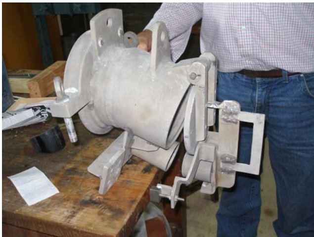
FIG. II-9. Flapper (flap valve) inspection.
