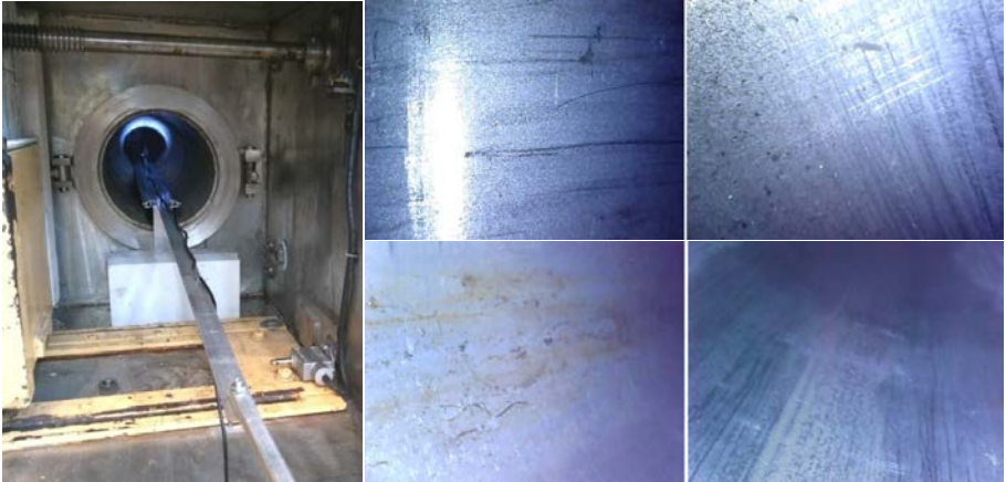
FIG. II-8. Visual inspection of neutron beam tubes.
