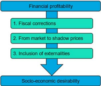
FIG. 16. Step by step procedure to move from a financial to a socioeconomic analysis.
