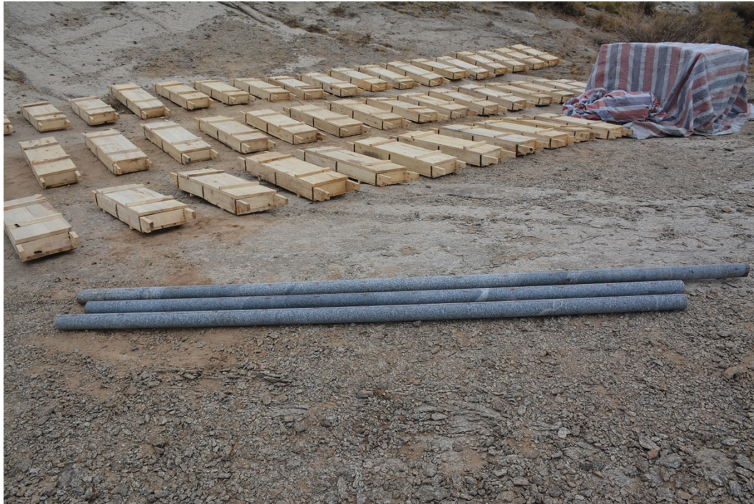
FIG. 36. Three contiguous ca. 3 m long intact cores of granite ready for cutting, packaging and transport at the Xin Chang site investigation in the Beishan region of NW China (reproduced courtesy of Beijing Research Institute of Uranium Geology).
