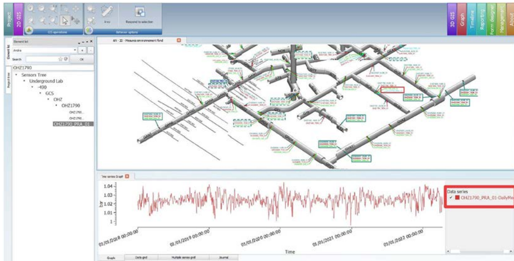
FIG. V–9. Sample visualization of data from drifts, boreholes and sensors produced using the web application (courtesy of Andra).
