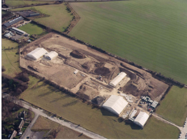
FIG. 8. Aerial view of the Southern Storage Area, Harwell, UK, during remediation work. Photograph courtesy of the United Kingdom Atomic Energy Agency and Magnox Ltd.
