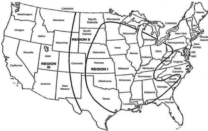
FIG. 19. Three hazard regions given in Ref. [109]. Tornado and straight wind hazard curves are given for each region. Region II includes two hurricane hazard curves (reproduced with permission from the American Nuclear Society).
