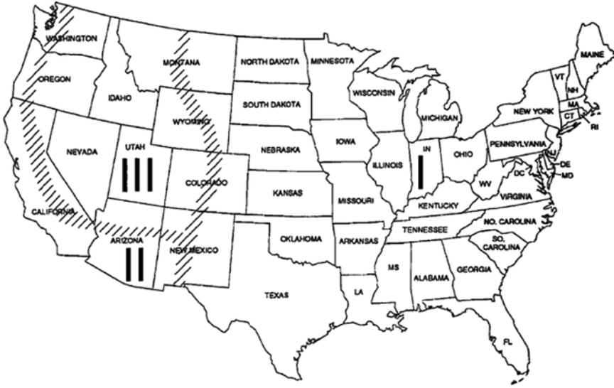
FIG. 18. Regional tornado hazard zones given in Ref. [107]. The region I wind speed is 360 mile/h (160 m/s), the region II wind speed is 300 mile/h (134 m/s) and the region III wind speed is 240 mile/h (107 m/s) (reproduced with permission from the US Nuclear Regulatory Commission).
