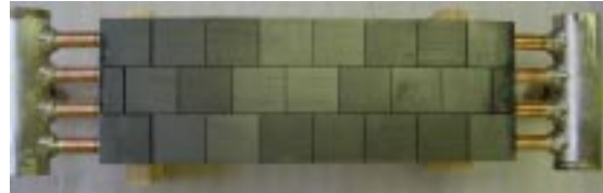
Fig. 6. A prototype flat CFC target with heat removal of 10 MW/m 2 .
