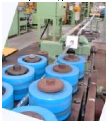
Fig. 3. A view of the 30 m length Nb 3 Al full-size conductor in trial manufacture.
