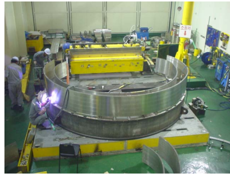
FIG. 3. Outer intercoil structure
