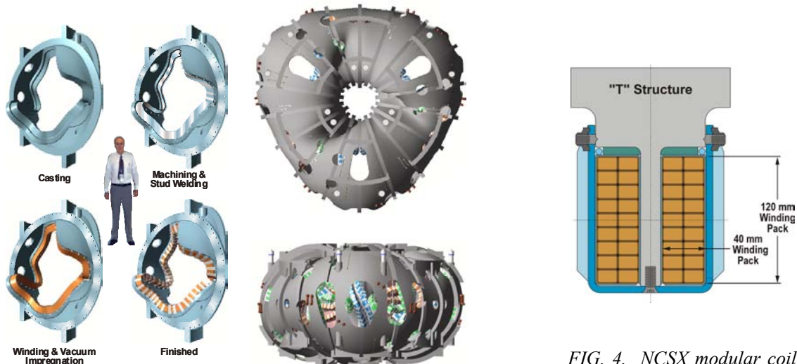
FIG. 4. NCSX modular coil cross section showing winding packs on either side of structural support
