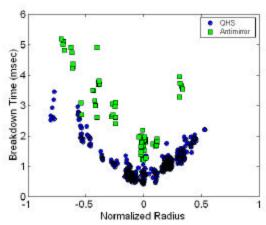
FIG. 1. Variation of the breakdown time with resonace location in the QHS and antiMirror configurations.
