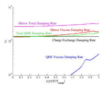
FIG. 7. Parallel viscous damping rates, the charge exchange damping rate, and the total damping rates, in the QHS and Mirror mode.
