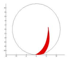
FIG. 2b. Orbit of a deeply trapped electron in the antiMirror configuration
