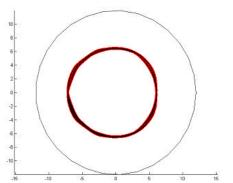
FIG. 2b. Orbit of a deeply trapped electron in the OHS configuration
