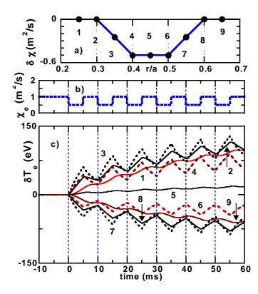
Fig. 5 Simulation of P-ITB-events (a) $\delta \chi_e$  profile, (b) evolution of  $\chi_e$  in time (c) evolution of  $\delta T_e$ .
