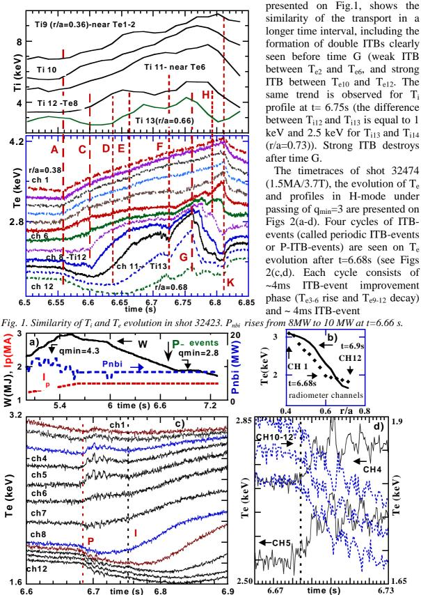
Figure 2(a) Timetraces of W,  $P_{nbi}$  and  $I_p$  in shot 32474. Transitionless H-mode [10] starts from t ~5.7s. P- start of periodical ITB-events at  $q_{min}=3$ . (b) Positions of radiometer channels and  $T_e$  (r) for t=6.68, 6.9 s. (c-d)  $T_e$  timetraces at periodical P-ITB-events and ITB-event-improvement I
