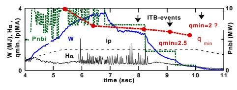
Fig.6. Timetraces of  $I_p$ , W,  $H_{\alpha}$ ,  $P_{nbi}$  and  $q_{min}$  in shot 36639
