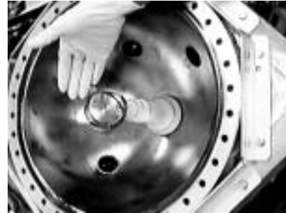
vacuum chamber : inner dia. = 340mm cathode grid (Ta) : inner dia. = 50mm outer dia. = 60mm thickness = 0.3mm
