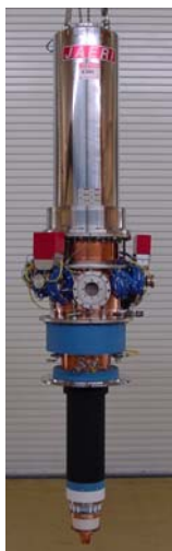
Fig.1: Appearance of 170GHz gyrotron. Height is ~3m.
