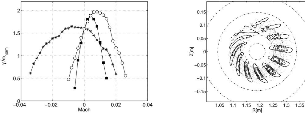
Figure 3: *Left: growth rates of the most unstable toroidal ITG mode vs Mach number for a sheared profile of  $u = E \times B/B^2$  (open symbols), for a shearless profile of  $u/\rho$  (filled symbols) and for a shearless profile of  $d\Phi_0/d\psi$  (stars). Right: perturbed  $\phi$  for a shearless profile of  $d\Phi_0/d\psi$  with  $\text{Mach}=-0.034$ .*
