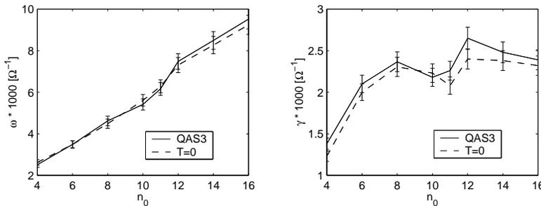
Figure 2: *Frequencies (left) and growth rates (right) of ITG modes vs dominant toroidal mode number in QAS3 (continuous line) and an equivalent tokamak (broken line).*
