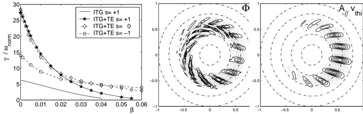
Figure 4: *Left: growth rates of most unstable ITG modes vs  $\beta$ , for different values of magnetic shear (plain line: without trapped electrons, other curves with). Perturbed  $\phi$  (middle) and  $A_{\parallel}$  (right), for the case  $\beta=4\%$ , shear= $+1$ .*
