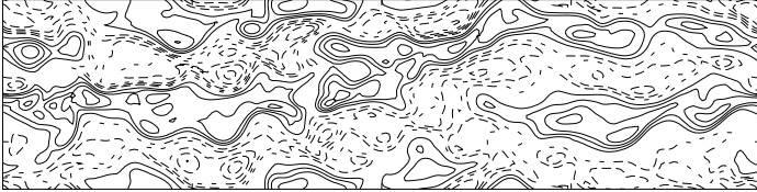
Figure 7: Characteristic \phi contours in the outboard x - y plane. This snapshot was taken at the end of the ETG run shown in Fig. 2. The figure is 256\rho_e \times 64\rho_e .
