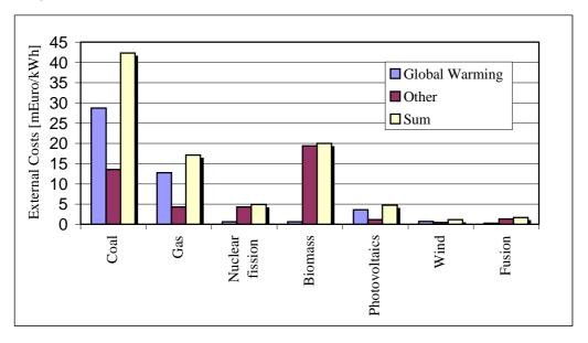
Figure 4 shows a comparison of the external costs of fusion with those of other major electricity sources. The external costs of fusion are rather low and compare well with those of wind and solar, which may play a major role in future energy systems.
