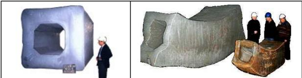
FIG. 11. Model 1 (Forging) - Austenitic Steel 316 LN (N=0.18%)
