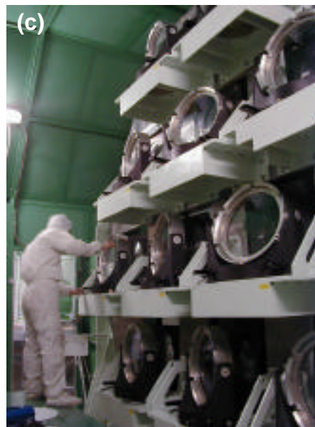
FIG. 1 HIPER focusing system. (a): schematic optical arrangement, (b): arrayed KDP cells, and (c): final mirror bundle.
