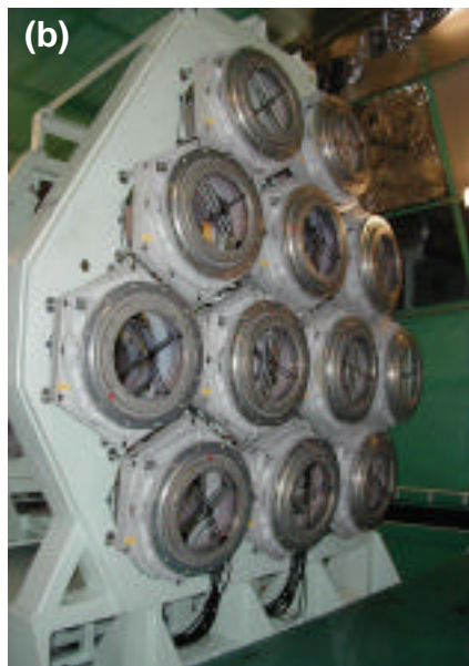
FIG. 1 HIPER focusing system. (a): schematic optical arrangement, (b): arrayed KDP cells, and (c): final mirror bundle.
