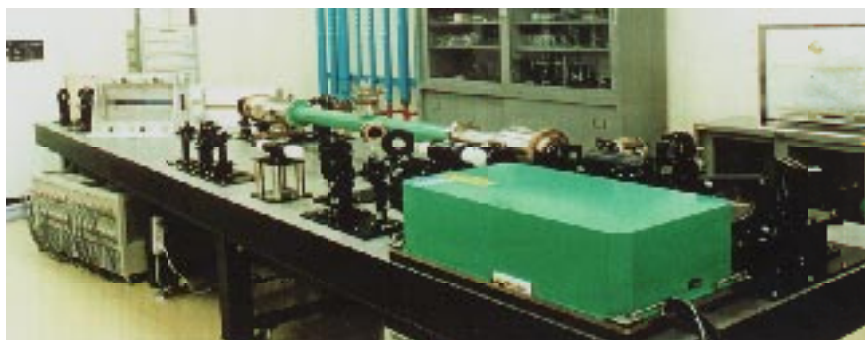
FIG.2. Photograph of laser-diode pumped 10 J x 10 Hz, Nd: glass slab laser module, HALNA 10.
