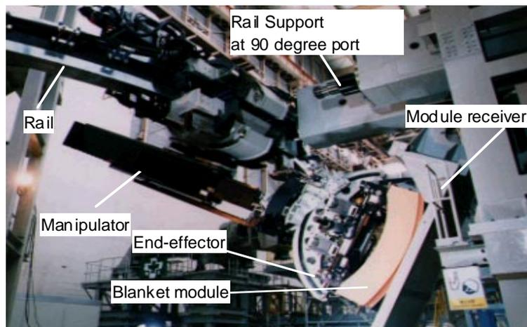
*FIG.4 Module transfer from manipulator to receiver*
