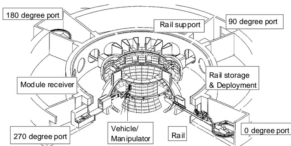
FIG.1 Rail-mounted vehicle manipulator system for blanket remote maintenance
