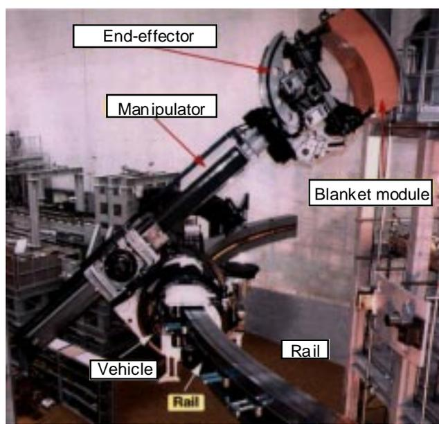
FIG.3 Module replacement by manipulator
