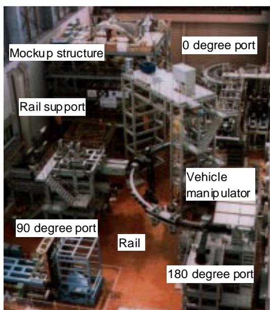
FIG.2 Blanket test platform
