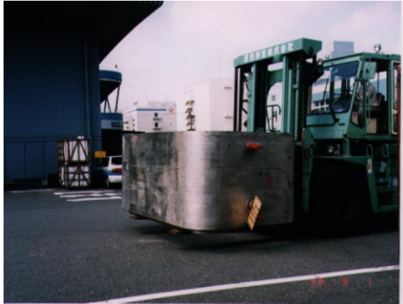
FIG. 4 View of the full-scale mid plane port extension shipped to Japan
