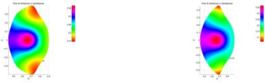
Fig. 2. The mod-B distribution in the Sphellamak at the beginning of the period (left) and at half period (right) for a case with -200\text{kA} toroidal current and \beta = 5.24\% .
