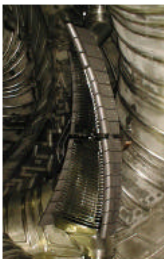
Fig.1. Water cooled antenna installed in the LHD.
