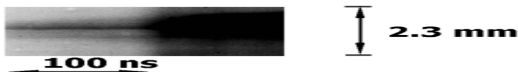
FIG. 3. The radial optical streak photograph of a fibre neck
