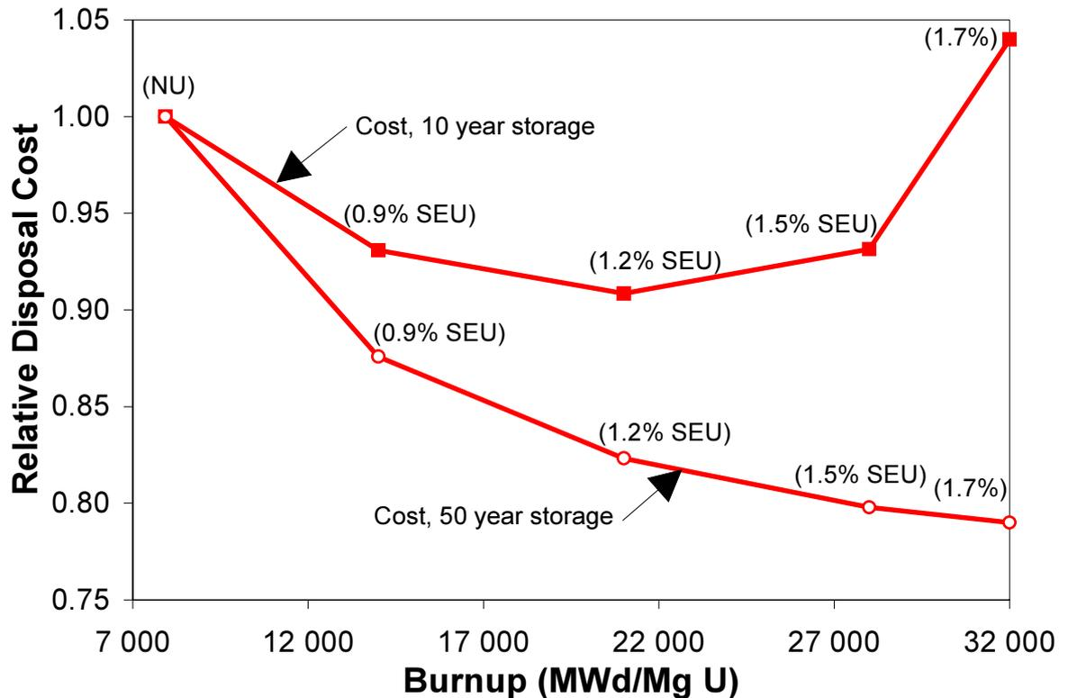
FIG. 4. Relative (Total disposal) Costs as a Function of Burnup (Enrichment) for the Direct Disposal of Spent CANDU Fuel Using Borehole Emplacement of Waste Containers in a Repository Excavated in Crystalline rock of the Canadian shield for a Fixed Generation of 4300 TW.h of Electricity.
