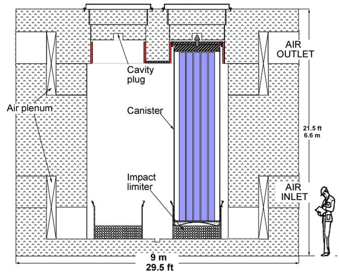
FIG. 3. MACSTOR Dry Storage Module - LWR Configuration
