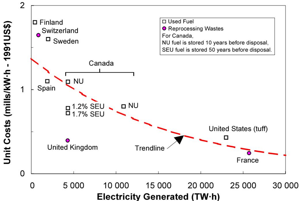
FIG. 5. Costs of Packaging and Disposing of Nuclear Fuel as a Function of Generated Electricity.
