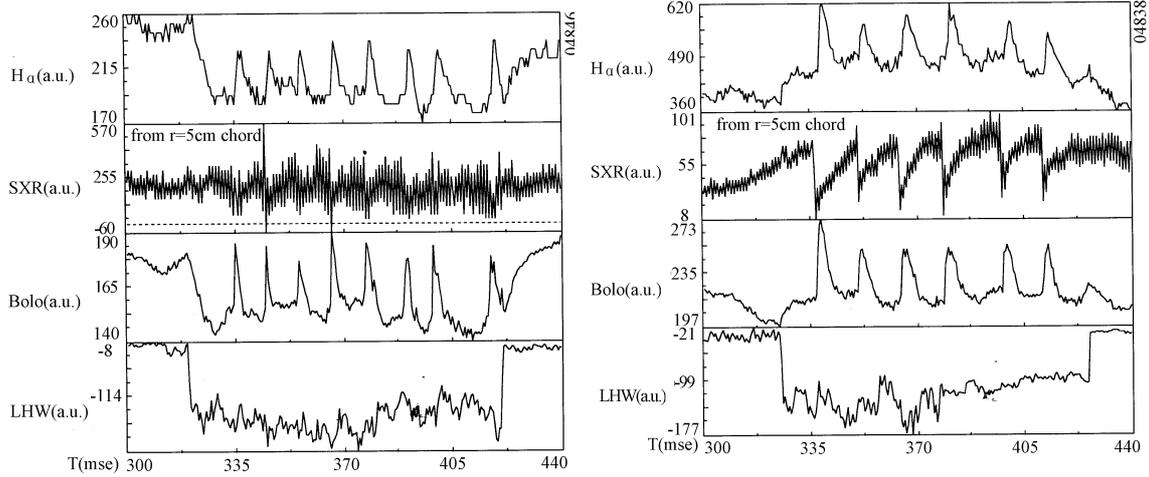
Fig.3 (a) ELM-like perturbation at low density (b) Low-frequency perturbation at high density
