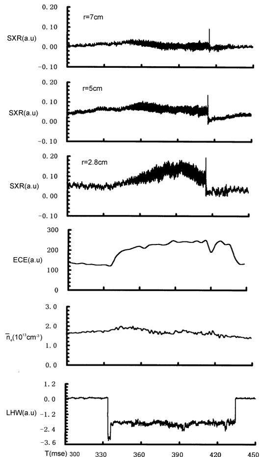
Fig.4 Plasma behaviors before and after the collapse of the soft-X ray radiation
