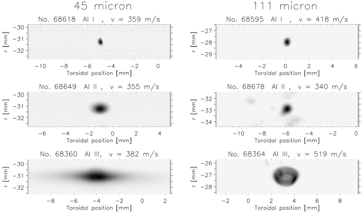
FIG. 3.  $1 \mu\text{s}$  exposure images of the pellet cloud in Al I, Al II and Al III light for two different pellet diameters.
