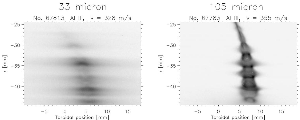
FIG. 2. Time integrated pictures of the Al III light of abating pellets of different diameters. The pellets travel upwards, the magnetic field is horizontal.
