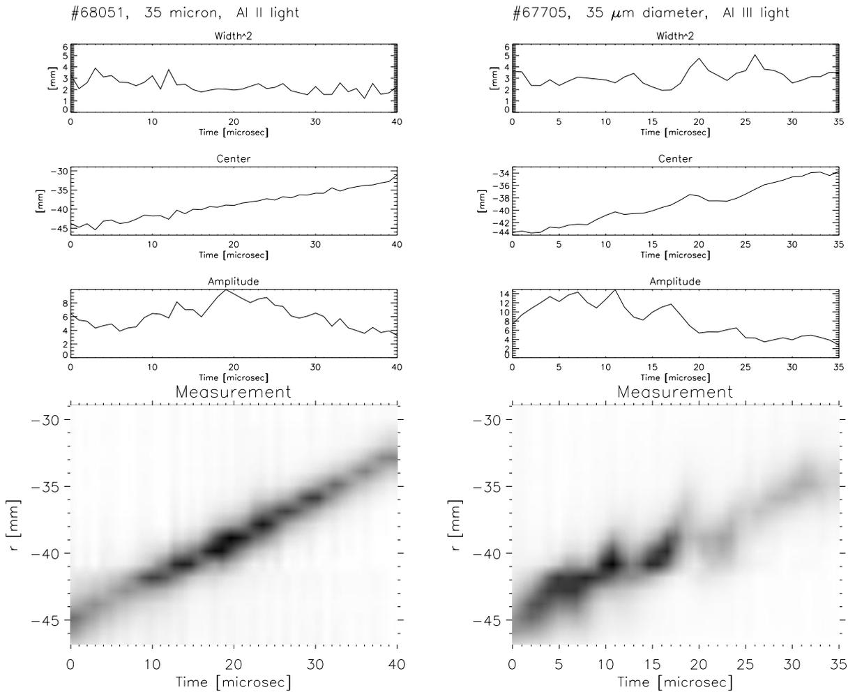
FIG. 4. Time evolution of the radial distribution of Al II and Al III light during the ablation of a small ( $35 \mu\text{m}$  diameter) pellet. The horizontal axis on the 2D plots is time, the vertical is the radial coordinate. The radially integrated amplitude, the center of mass and the width of the profiles are plotted as a function of time on the curves above the images.
