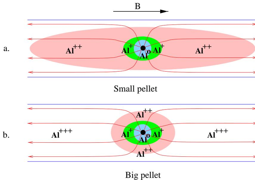
FIG. 1. Structure of the pellet cloud for small (a.) and large (b.) pellet.
