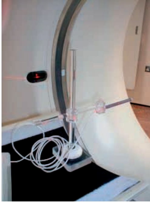
FIG. 8.7. Arrangement for the measurement of the CT air kerma index free in air, C_{a,100} . The chamber is clamped in a specially designed support and aligned so that it is coaxial with the scanner rotation axis and its sensitive volume is bisected by the scan plane. In this particular example, alignment has been achieved with the aid of lasers.
