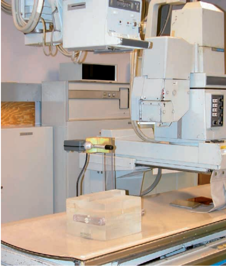
FIG. 8.1. Experimental set-up for measurements using a CDRH abdomen/lumbar spine phantom on the table top with the ionization chamber positioned above the phantom.
