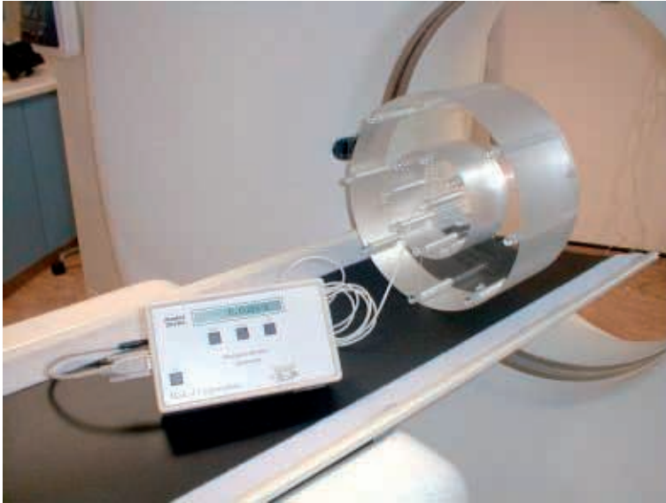
FIG. 8.8. Arrangement for the measurement of the CT air kerma index, C_{PMMA,100,\phi} in the standard body phantom. The phantom is positioned on the couch top and the chamber is positioned in the central hole of the phantom. A plastic sleeve is placed over the chamber to ensure a good fit within the phantom. The central plane of the phantom has still to be aligned with the position of the scan slice. In practice, the phantom may be secured in position using masking tape.
