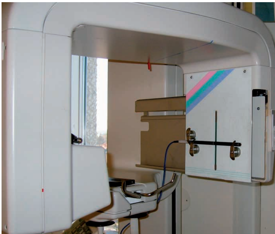
FIG. 8.9. Experimental arrangement for measurements of the air kerma–area product for a dental panoramic unit using a CT chamber.
