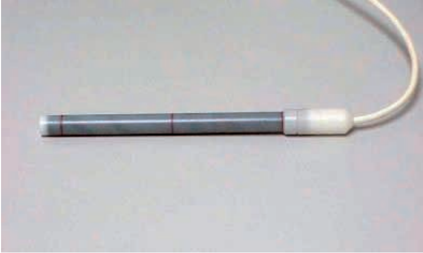
FIG. 8.6. Pencil ionization chamber used for dosimetry of CT examinations. The active volume of the chamber is 3 \text{ cm}^3 and the active length 100 mm.
