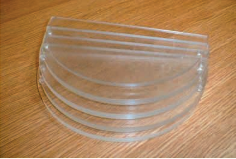
FIG. VII.3. Photograph of a 45 mm thick PMMA phantom for use in breast dosimetry. This particular phantom is comprised of four semicircular slabs of thickness 10 mm and one slab of thickness 5 mm. The slabs have been partially separated for purposes of illustration. The use of a multislab phantom allows the possibility of measurements at thicknesses other than 45 mm. The thickness tolerance specified for the phantom applies to the total thickness and not the thickness of the individual slabs.
