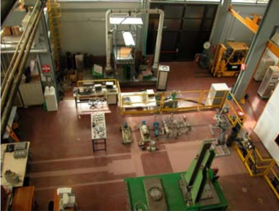
*FIG. 16. Former hall of the RB-2 reactor, now converted to an experimental test laboratory for structures and components at ambient and high temperature.*
