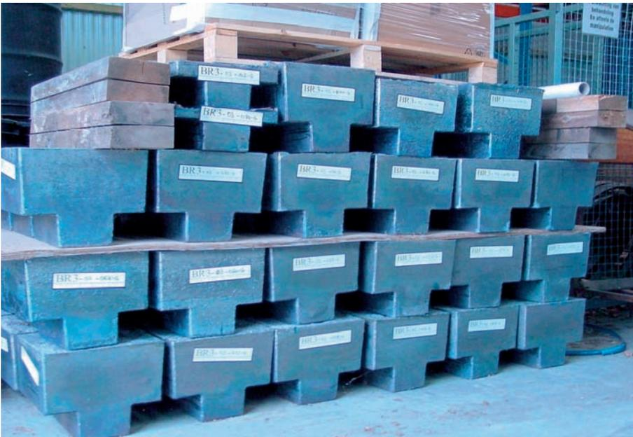
*FIG. A-14. Thirty-four tonnes of lead has been extracted and unconditionally cleared.*
