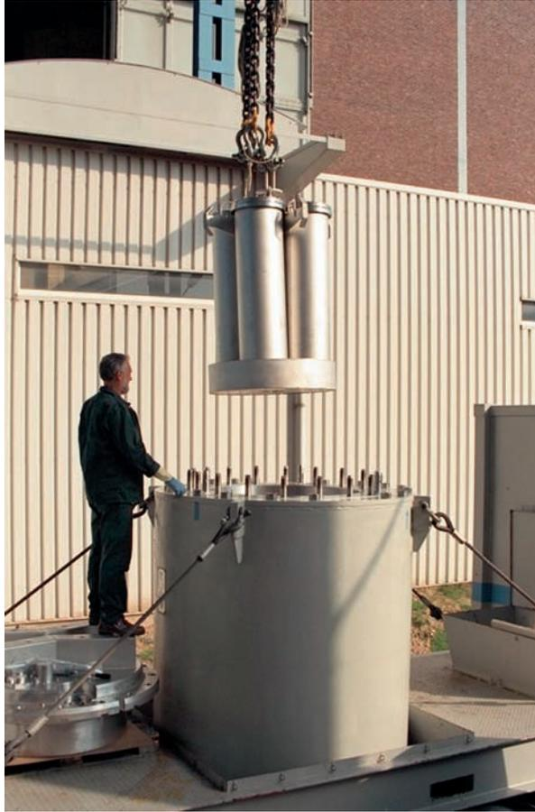
*FIG. A-5. Four empty canisters for holding the beryllium and the empty transport container arriving at the BR2 MTR.*
