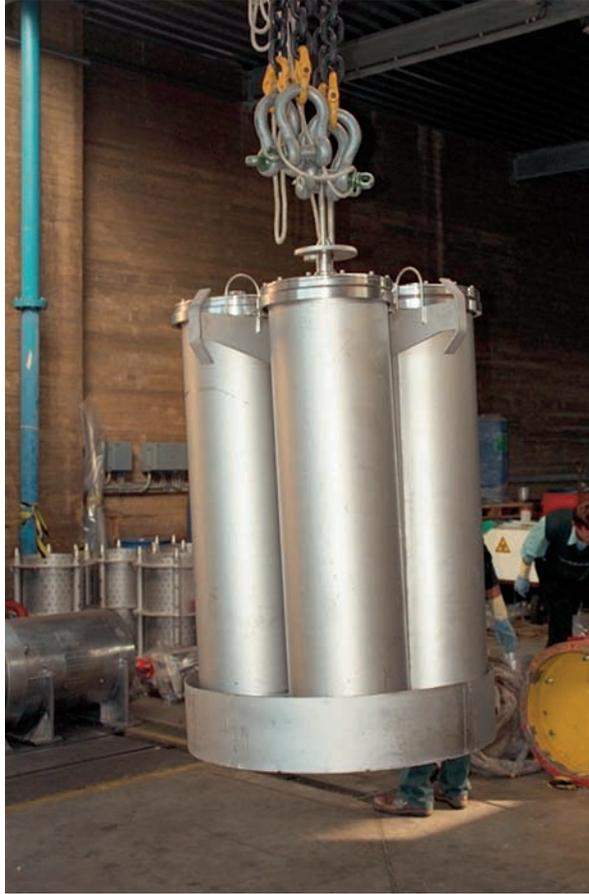
*FIG. A-4. Four empty canisters for holding the beryllium.*
