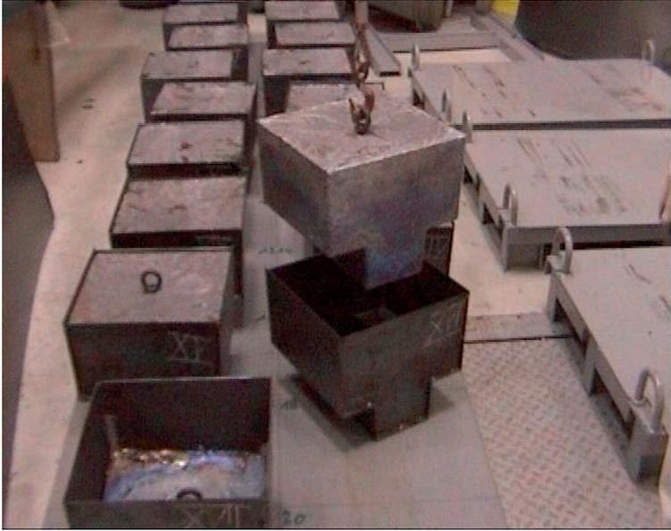
*FIG. A-13. Removal of the lead ingots after cooling.*
