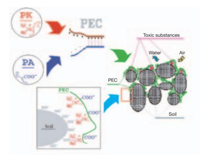
FIG. 12. Binding of soil particles and entrapment of contaminants using organic polymers (S. Mikheykin, VNIICHT, Moscow, personal communication).
