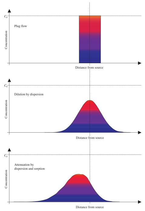
FIG. 4. Transport mechanisms effecting dilution and attenuation.
