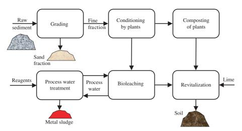
FIG. 22. The experimental process from raw contaminated sediment to reconditioned soil, after Ref. [377].
