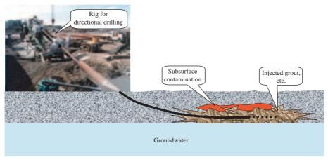
FIG. 8. The principle of directional drilling and grouting.
