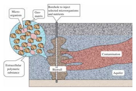
FIG. 13. The principle of a biowall.
