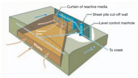
FIG. 9. Trench and gate system [202].
