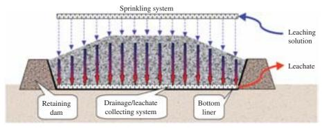
FIG. 21. A heap leaching system.
