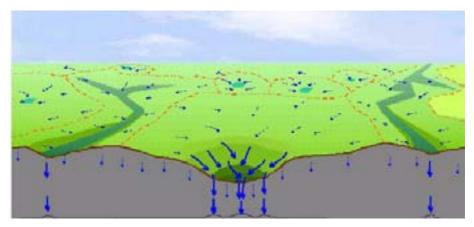
FIG. 1. Schematic representation of radionuclide accumulation in topographical depressions due to near surface migration, soil erosion, etc. [21].
