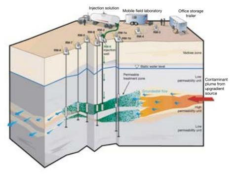
FIG. 11. In situ redox manipulation (courtesy of Batelle).
