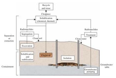
FIG. 3. Classification of remediation technologies by function (adapted from Ref. [34]).
