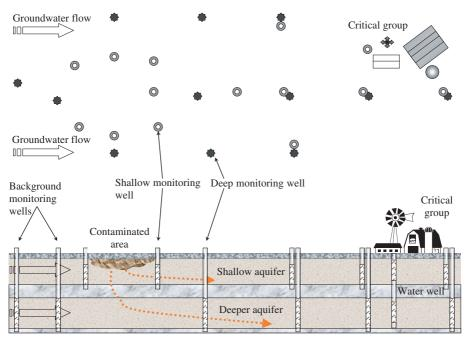
FIG. 5. The principle of monitored natural attenuation.
