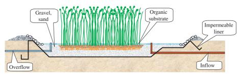
FIG. 15. Schematic cross-section of a constructed wetland.
