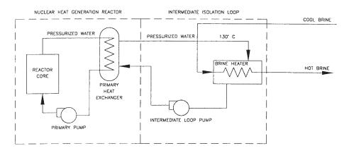
FIG. 5.2. Intermediate isolation loop between heating reactor and MSF plamt.
