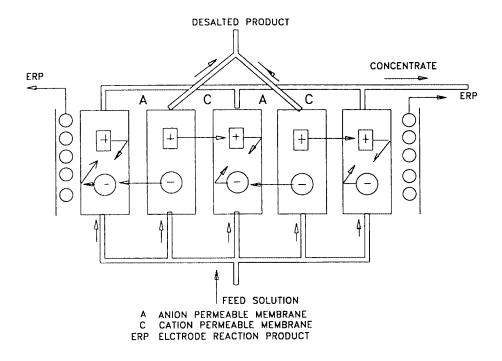
FIG. 4.5. Schematic diagram of the electrodialysis (ED) desalination process.
