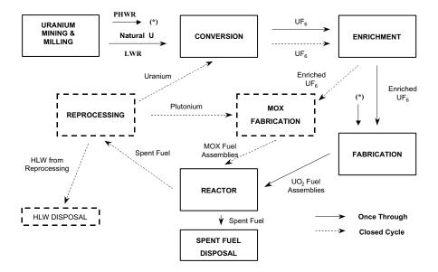
FIG. 3.1. Schematic representation of LWR once-through and closed fuel cycles.
