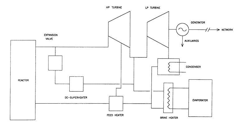
FIG. 6.2. Dual purpose plant extraction cycle.
