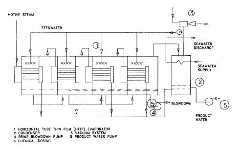
FIG. 4.2. Schematic flow diagram of the multiflect (MED) desalination process.
