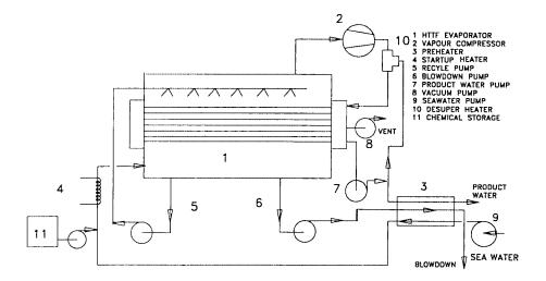
FIG. 4.3. Schematic flow diagram for the vapour compression (VC) desalination process.
