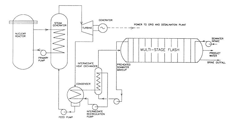
FIG. 5.4. Schematic diagram of a nuclear power reactor coupled to an MSF plant.
