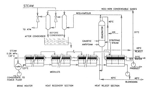
FIG. 4.1. Schematic flow diagram of the multistage flash (MSF) desalination process with brine recirculation.
