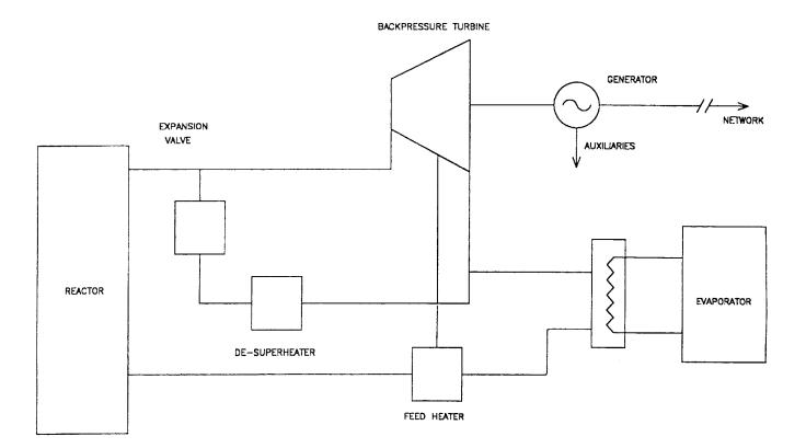
FIG. 6.1. Dual purpose plant backpressure cycle.
