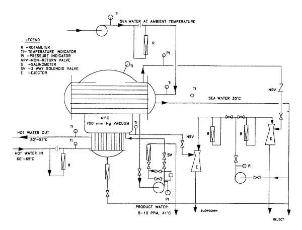
FIG. 4.6. Schematic flow diagram of a low temperature vacuum evaporation (LTE) desalination system.
