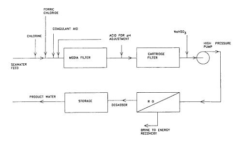
FIG. 4.4. Schematic flow diagram of a reverse osmosis (RO) desalination plant.
