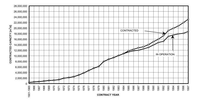
FIG. 2.3. Cumulative capacity of all land based desalting plants capable of producing 100  $m^3/d$  and per unit or more fresh water versus contract year.
