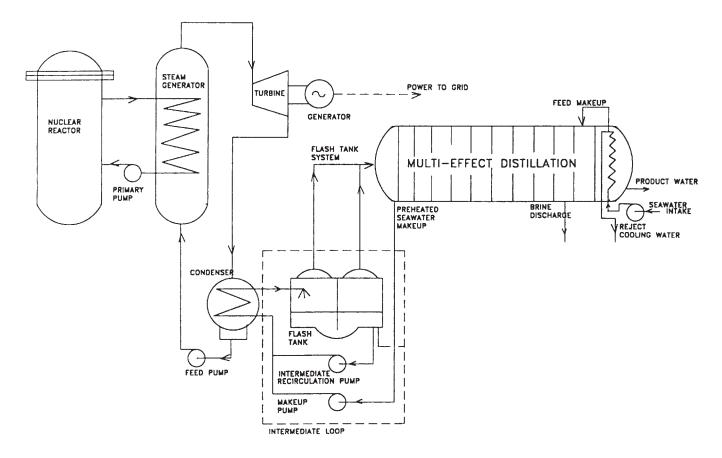
FIG. 5.5. Schematic diagram of a nuclear power reactor coupled to an MED plant.
