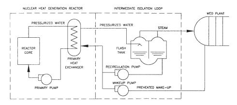
FIG. 5.3. Intermediate isolation loop between heating reactor and MED plant.
