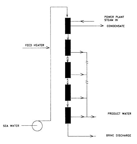
FIG. 4.7. Schematic process flow diagram of a stacked vertical tube evaporation plant.
