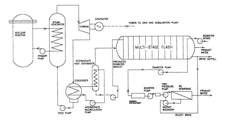
FIG. 5.6. Schematic diagram of a nuclear power reactor coupled to an MSF-RO plant.
