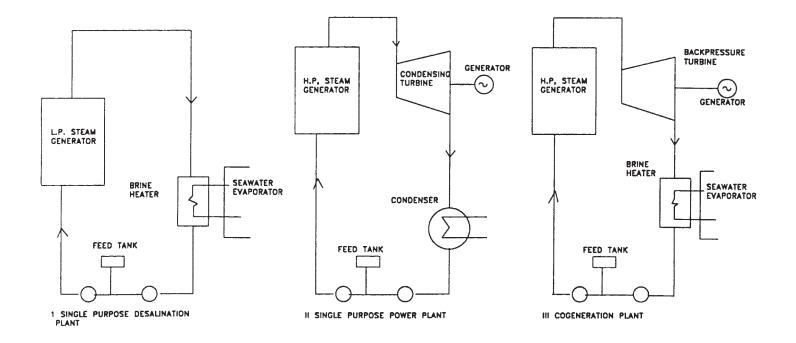
FIG. 5.1. Schematic representation of single purpose plants and a co-generation plant.
