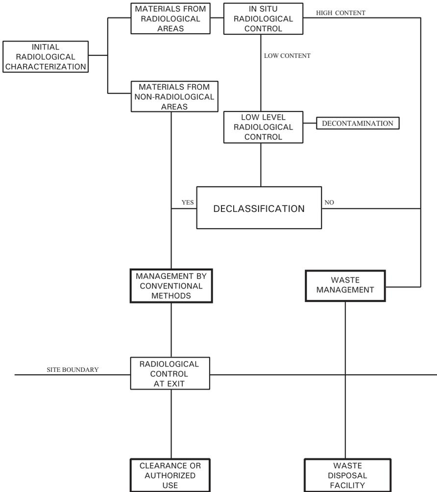
FIG. 5. Material/waste management during Vandellós decommissioning.
