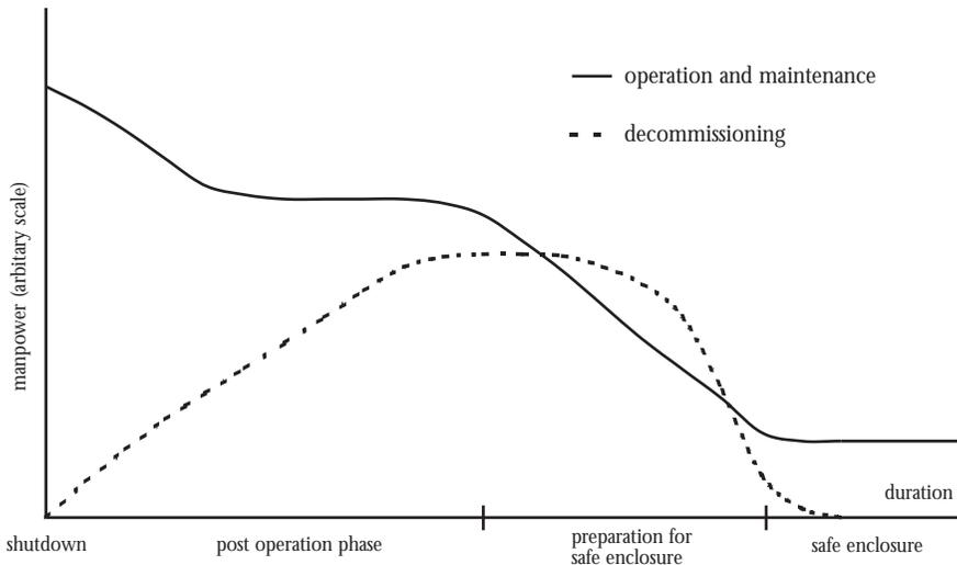
FIG. 1. Typical staff reduction profile during decommissioning.
