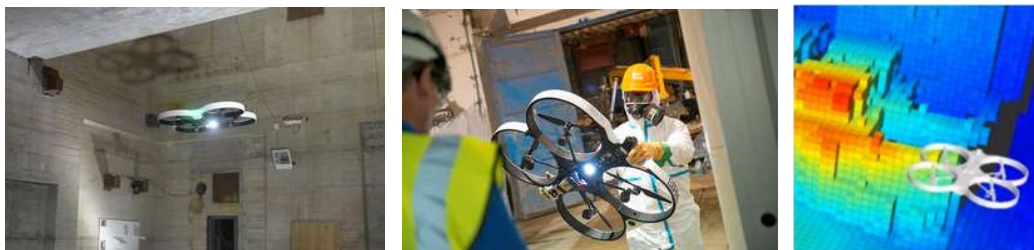
FIG.17. Sellafield: remotely operated unmanned aerial vehicle combined with radiation mapping software (Photo courtesy of Blue Bear Systems Research Ltd, United Kingdom)
