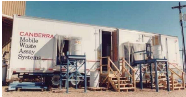
FIG. 16. The Mobile Characterization Solutions (MCS) unit for TRU drum characterization – WIPP Overview, USA (Photo courtesy of Mirion Technologies)
