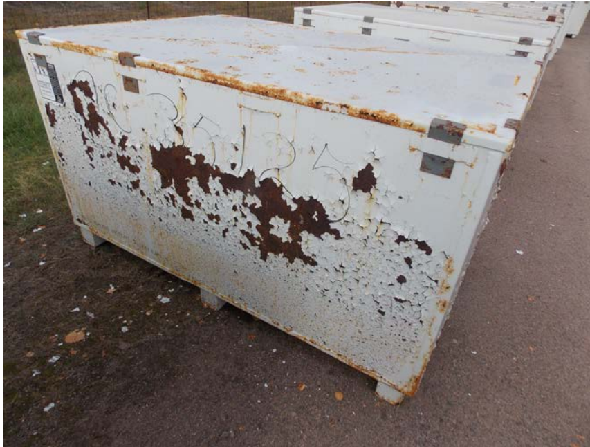
FIG.12. Corroded containers after a decade storage period (photo courtesy of AECL Canada)
