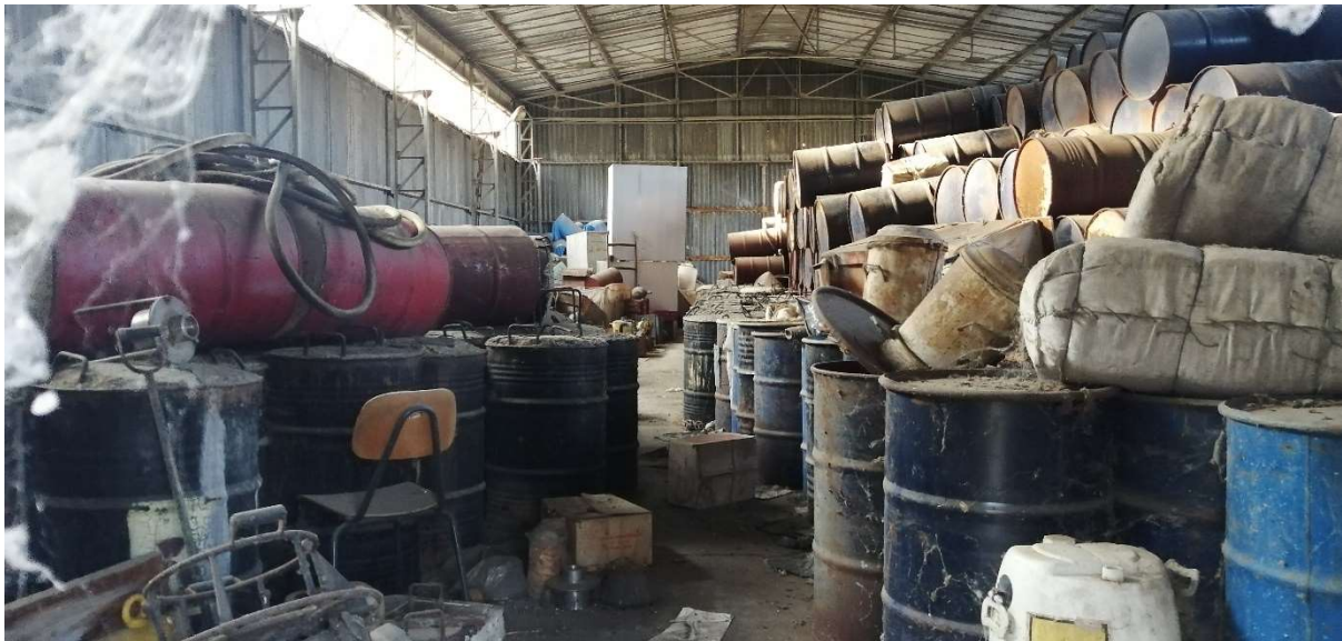
FIG. 4. Solid waste stored in Hangar 1 at Vinca site, Serbia illustrating a wide variety of wastes stored in varying containers. (Photo courtesy of Public Company Nuclear Facilities of Serbia - PC NFS)
