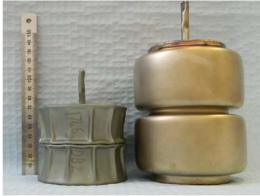
FIG. 22. Photos of the HIPed (left) and unHIPed (right) 2DB canisters for future waste encapsulation (Photo courtesy of ANSTO, Australia)
