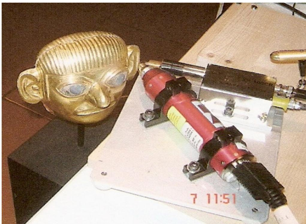
FIG 1. Experimental set-up, showing, on the left, the Eclipse II X ray tube (with a brass collimator), and the Si-PIN detector (also collimated with a brass cylinder), during measurements on the golden mask, in the Museum “Tumbas Reales de Sipán”, in Lambayeque, Peru.
