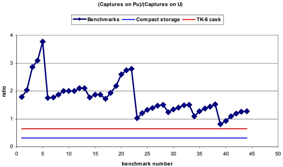
Fig. 8. Ratio of captures happening on plutonium to the fission happening on uranium homogeneous MOX benchmarks.
