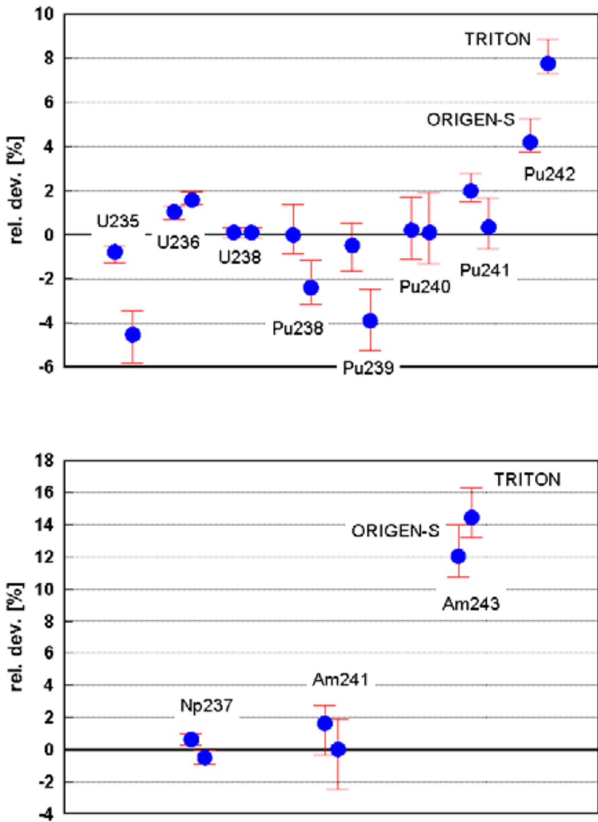
Fig.2.4a Deviation of nuclide concentration, numerical benchmark CB2 (6 samples).
