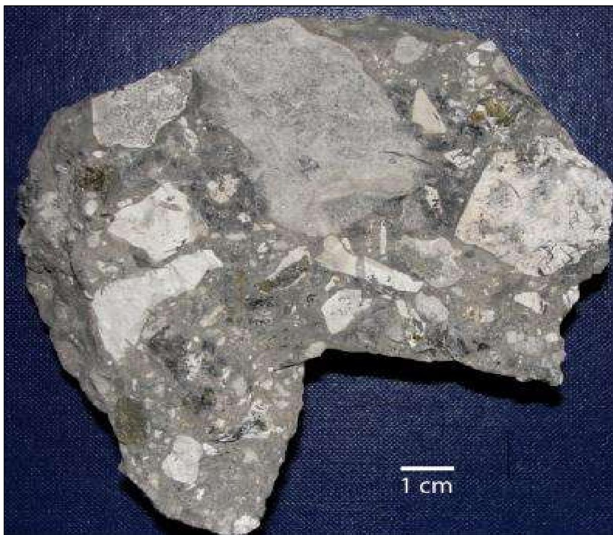
FIG. 123. Example of uranium ore from a solution collapse breccia pipe in northern Arizona, USA. This breccia is from the Pigeon (mine) breccia pipe. The sample contains 0.606% U, 0.25% As, 0.13% Zn, 0.07% Ni and many other metals. Uraninite (UO<sub>2</sub>) is the principal uranium mineral. Photograph courtesy of B. Van Gosen (reproduced with permission).
