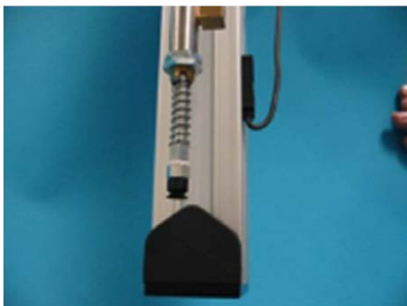
FIG. 14. Left: Rubber seal at the end of a tube connected to an underpressure system; capsule is sucked to this rubber (TU Delft, Netherlands); Right: similar system, positioned on top of a sample vial (courtesy of Centro de Desenvolvimento da Tecnologia Nuclear, Brazil).
