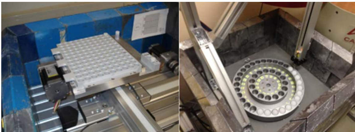
FIG. 16. a) Left: Rectangular sample storage on an X-Y positioning table (courtesy of TU Delft, Netherlands); b) Right: Rotating disc containing samples (courtesy of JINR, Russian federation).
