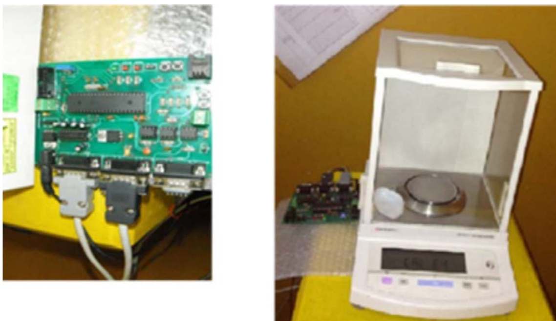
FIG. 19. Interface card and its connection to the balance at IPEN, Peru (courtesy of Instituto Peruano de Energía Nuclear, Peru).
