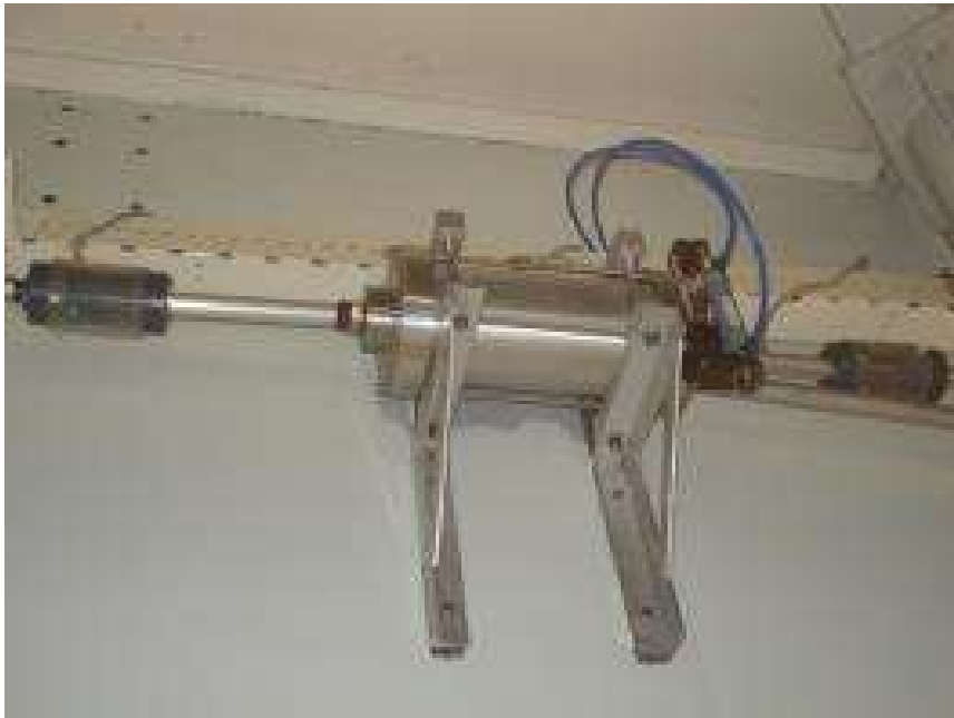
FIG. 5. Example of a diverter in the fast pneumatic system at Reactor Institute Delft. The diverter is pneumatically operated. Optical sensors can be seen on the left and right of the diverter (courtesy of TU Delft, Netherlands).
