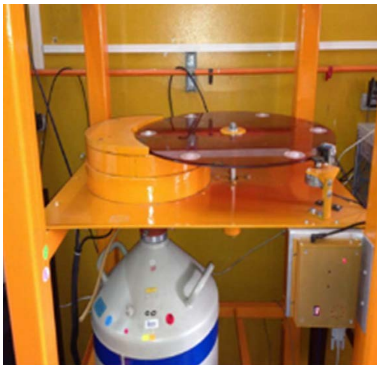
FIG. 17. Lead shield with sample disc on top (courtesy of Instituto Peruano de Energía Nuclear, Peru).
