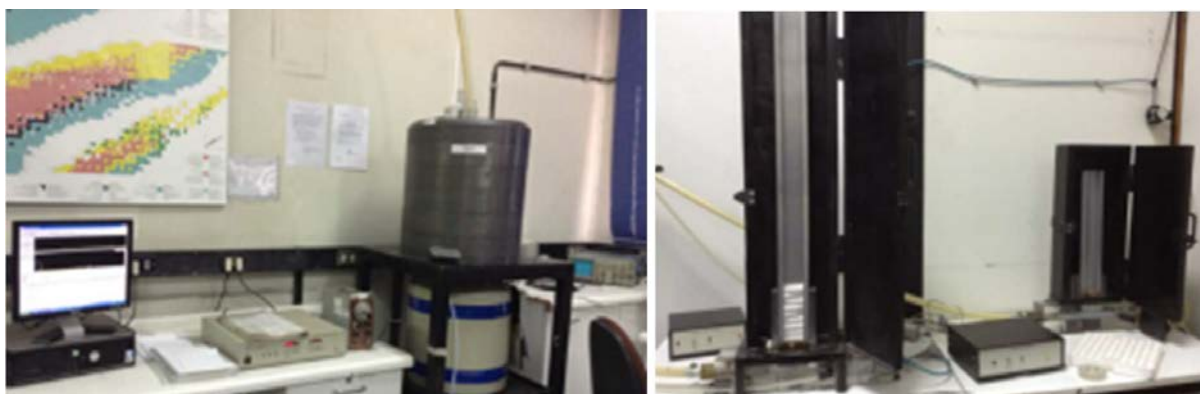
FIG. 9. Counting room at CCHEN, Chile, showing (left) shielded Ge detector and part of the tubing of the pneumatic transfer system of the sample changer and (right) stack loader of the sample changer (courtesy of Comisión Chilena de Energía Nuclear, Chile).
