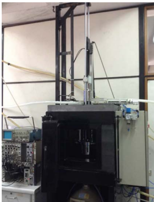
FIG. 4. Compton suppressor gamma system with automatic sample changer (courtesy of Comisión Chilena de Energía Nuclear, Chile).
