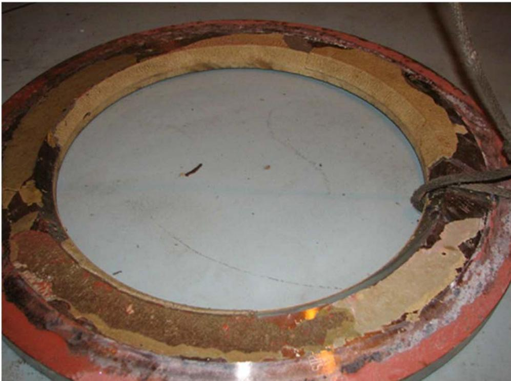
*FIG. 37. The orifice plate as removed for inspection (Courtesy of the SAFARI-1 of the South African Nuclear Energy Corporation (NECSA), South Africa).*
