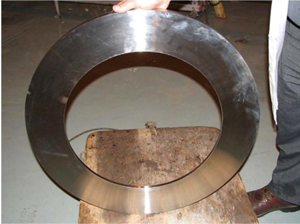
*FIG. 38. Cleaned orifice plate ready for installation (Courtesy of the SAFARI-1 of the South African Nuclear Energy Corporation (NECSA), South Africa).*
